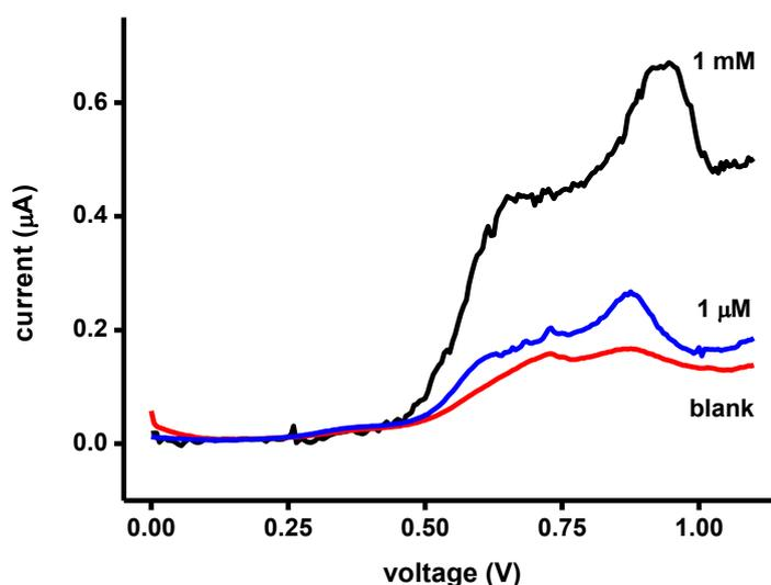
**Figure 4.** SWV for colored dipsticks with bound AChE. Black and blue curves: assay of 1 mM and 1 µM paraoxon, red curve: assay of 5% isopropanol only (blank).
