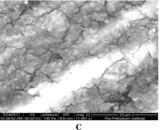
**Figures 1 A-C.** ESEM images of the Indian aluminum sample after exposure to green cabbage solution at boiling temperature for 20 minutes.
