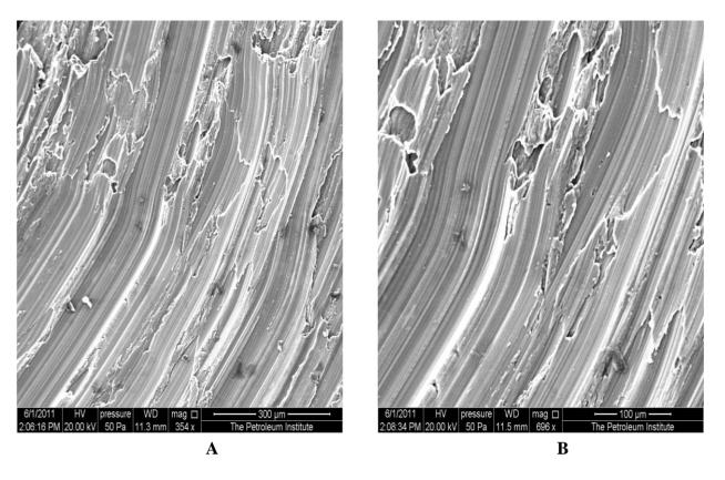
**Figures 5 A-B.** ESEM images of the Indian sample after exposure to peeled eggplant solution at boiling temperature for 20 minutes
