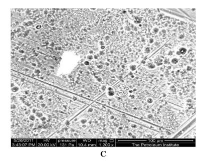
**Figures 2** A-C. ESEM images of the Indian aluminum sample after exposure to the concentrated green cabbage solution at boiling temperature for 20 minutes.
