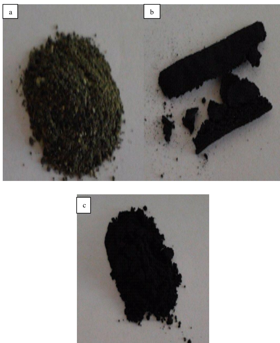
Scheme 1. Photos for the samples obtained in preparing stages. Photo a : after being dried at 80°; photo b : sample dried at 300 °; photo c : the product of 7 wt% PANI-doped Li 3 V 2 (PO 4 ) 3 .
