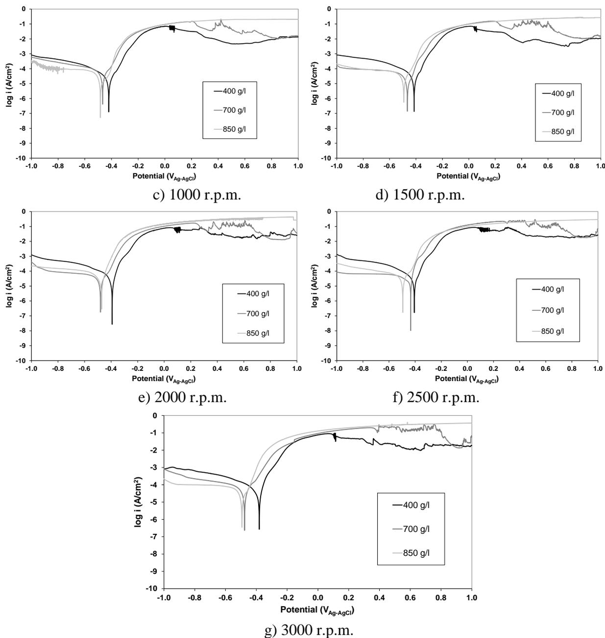
**Figure 2.** Polarisation curves of copper at the different rotation rates in the three used LiBr solutions at 25 °C.
