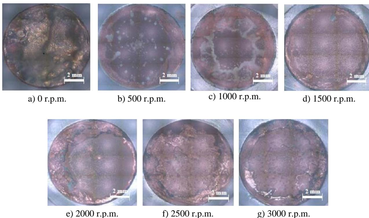
**Figure 9.** Images of the electrode surface after the tests in the 400 g/l LiBr solution at 25 °C at the different rotation rates.
