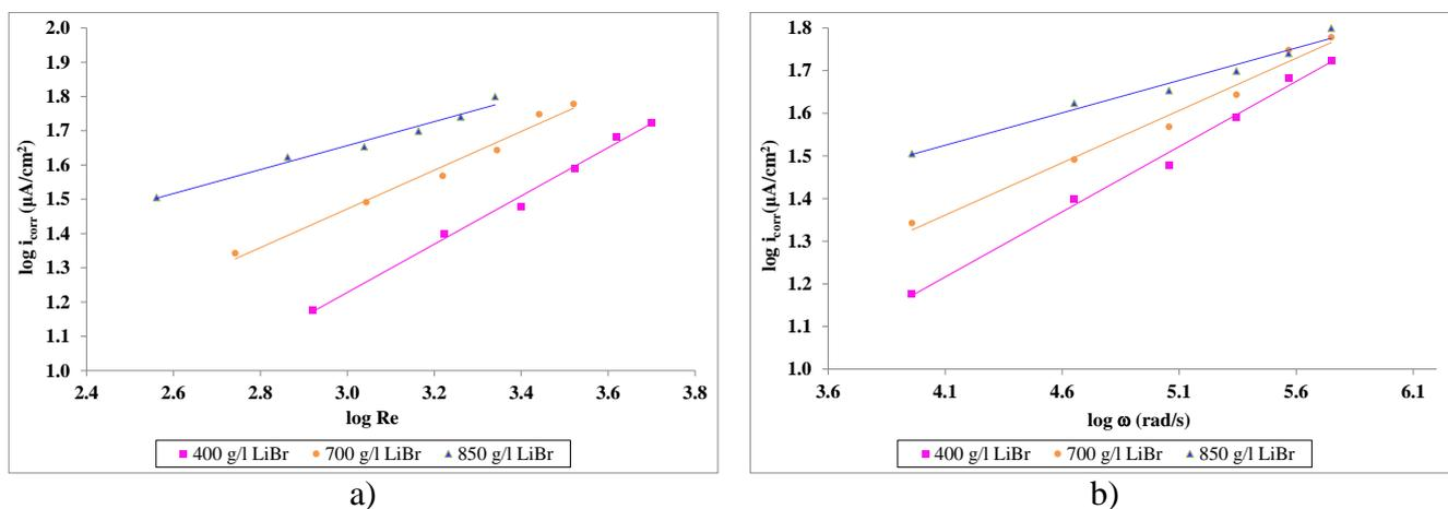
**Figure 8.** a) Logarithm of  $i_{\text{corr}}$  versus the logarithm of the Reynolds number in the different aqueous LiBr solutions at 25 °C. b) Logarithm of  $i_{\text{corr}}$  versus the logarithm of the angular velocity  $\omega$  in the different aqueous LiBr solutions at 25 °C.
