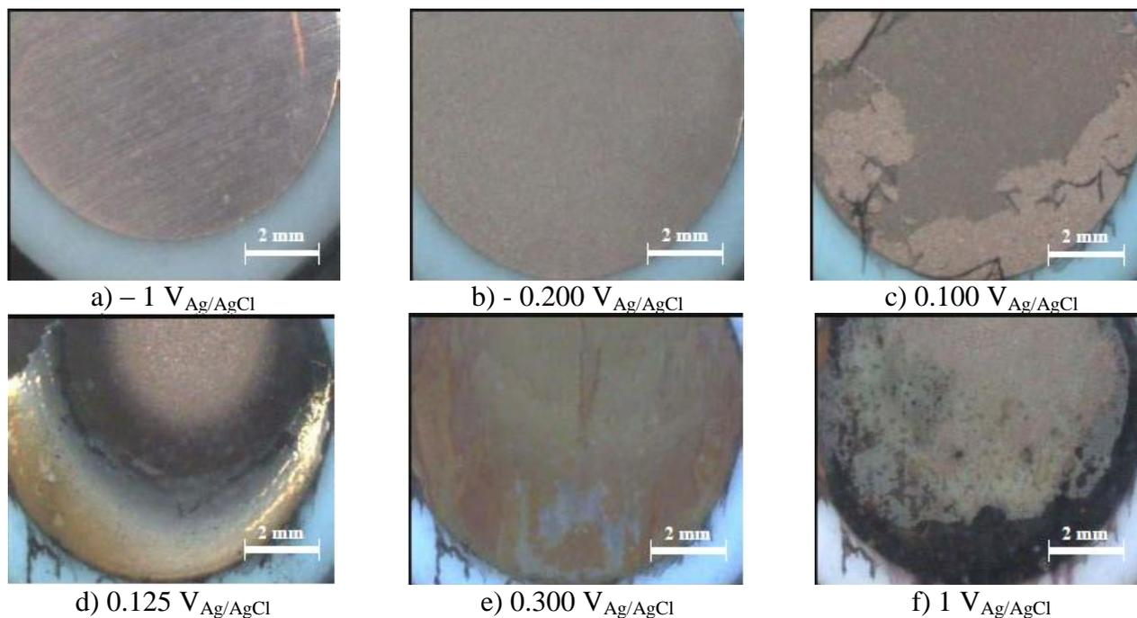
**Figure 5.** Images of the electrode surface obtained at different points of the polarisation curves taken with the electro-optical patented devices in the 850 g/l LiBr solution at 25 °C under static conditions.
