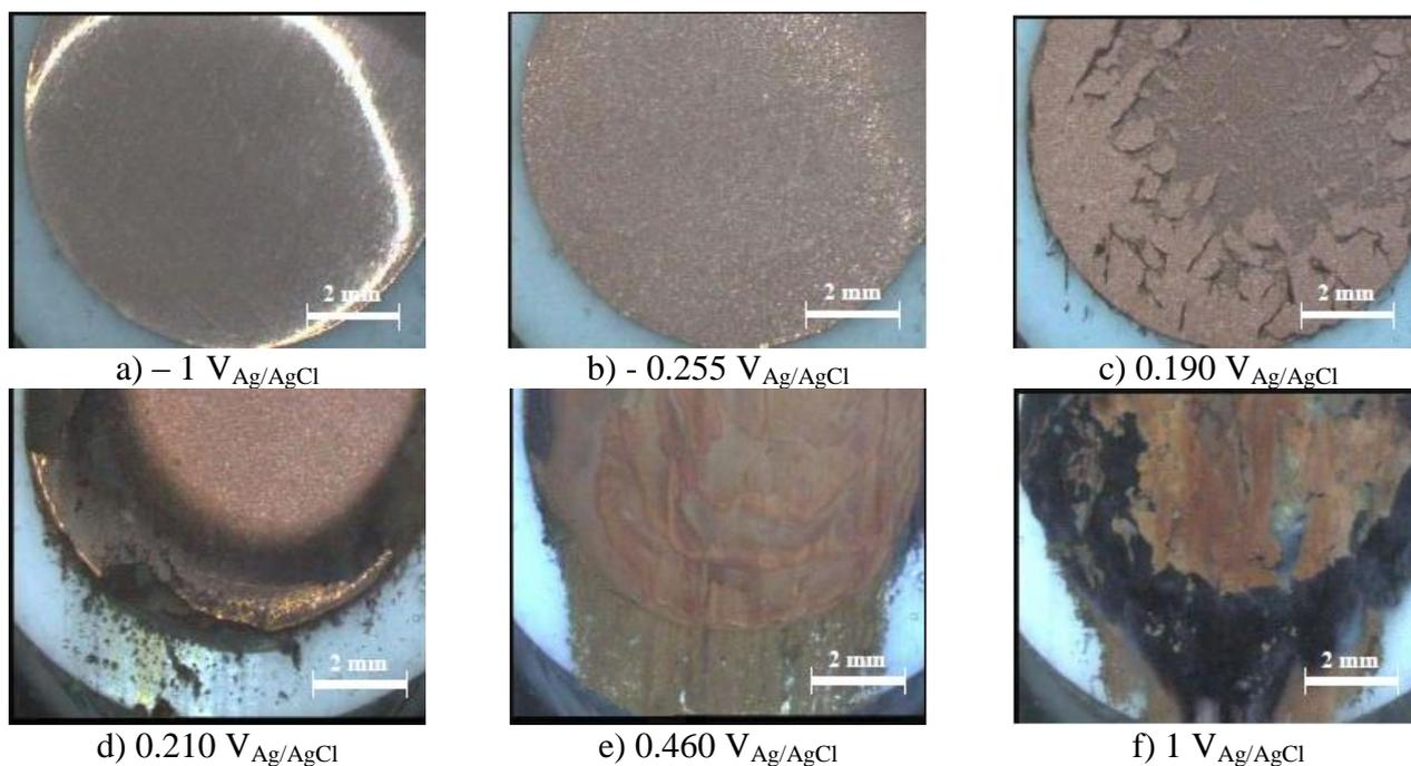
**Figure 4.** Images of the electrode surface obtained at different points of the polarisation curves taken with the electro-optical patented devices in the 700 g/l LiBr solution at 25 °C under static conditions.
