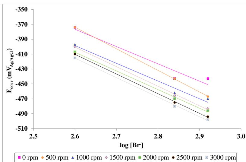
**Figure 7.** Evolution of the corrosion potential of copper with the logarithm of the LiBr concentration for every rotation rate value at 25 °C.
