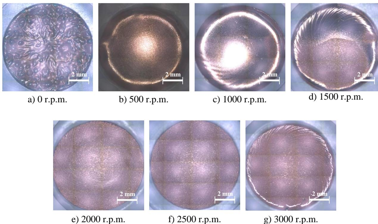
**Figure 11.** Images of the electrode surface after the tests in the 850 g/l LiBr solution at 25 °C at the different rotation rates.
