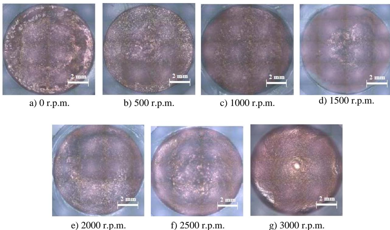
**Figure 10.** Images of the electrode surface after the tests in the 700 g/l LiBr solution at 25 °C at the different rotation rates.
