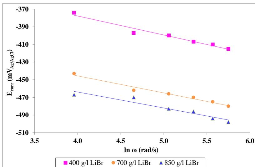
**Figure 6.** Corrosion potential ( $E_{corr}$ ) of copper in function of the  $\ln \omega$  (rad/s) in the different aqueous LiBr solutions at 25 °C.
