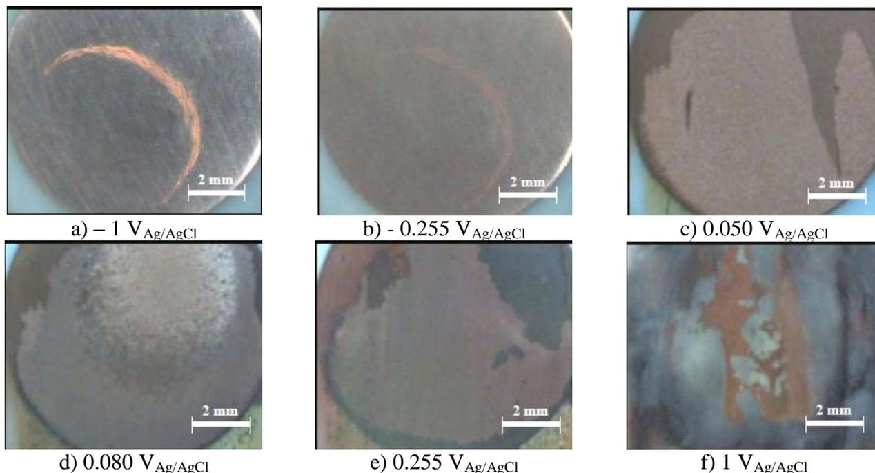
**Figure 3.** Images of the electrode surface obtained at different points of the polarisation curves taken with the electro-optical patented devices in the 400 g/l LiBr solution at 25 °C under static conditions.
