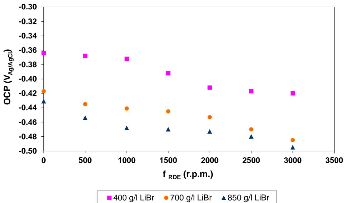
**Figure 1.** Effect of the rotation rate on the open circuit potential (OCP) of copper in the different aqueous LiBr solutions at 25 °C.
