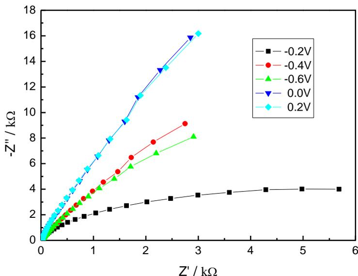
**Figure 7.** Simulated curves of EIS impedance at different potentials.
