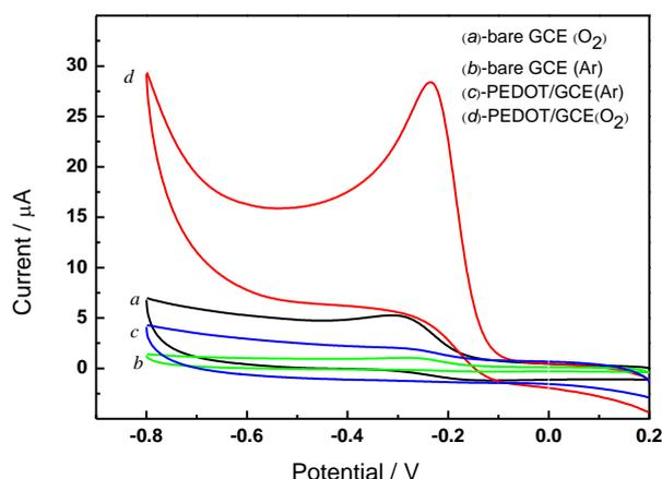
**Figure 3.** Cyclic voltammograms of :(a)bare GCE with  $\text{O}_2$ ; (b)bare GCE with Ar; (c) PEDOT-modified GCE with Ar; (d)PEDOT-modified GCE with  $\text{O}_2$ . (Scan rate =  $50\text{mV}\cdot\text{s}^{-1}$ )
