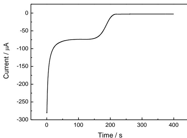
**Figure 2.** The current-time curve for electropolymerisation of EDOT at 1.19V on GCE.
