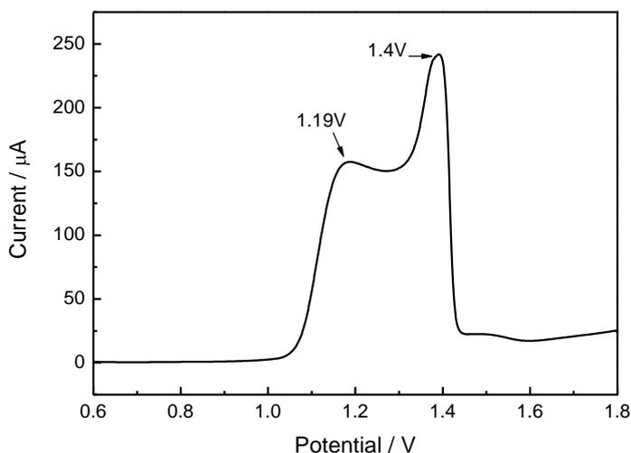
**Figure 1.** Linear voltammogram of  $1 \times 10^{-3}$  M EDOT in 0.1 M  $\text{Na}_2\text{SO}_4$  using a GCE (scan rate:  $10 \text{ mV} \cdot \text{s}^{-1}$ )
