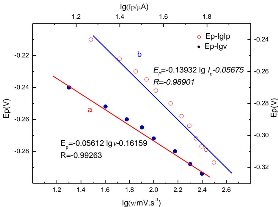
**Figure 5.** Tafel plot of Afc and sulfite: (a)  $E_p$  vs.  $\text{Log } v$ ; (b)  $E_p$  vs.  $\text{log } I_p$ .
