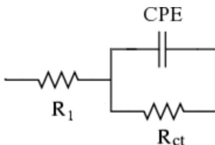
**Figure 6.** Equivalent circuit used to fit the experimental EIS data.
