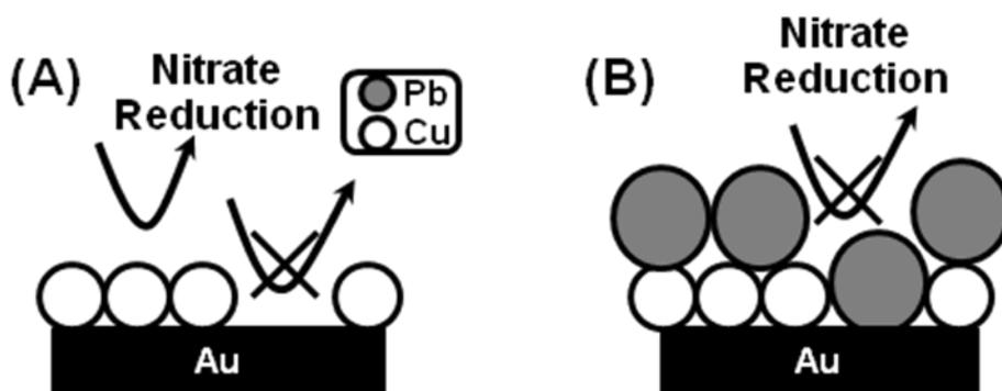
**Scheme 2.** Schematic diagram of nitrate reduction (A) on copper modified Au and (B) Pb upd layer on Cu modified Au.
