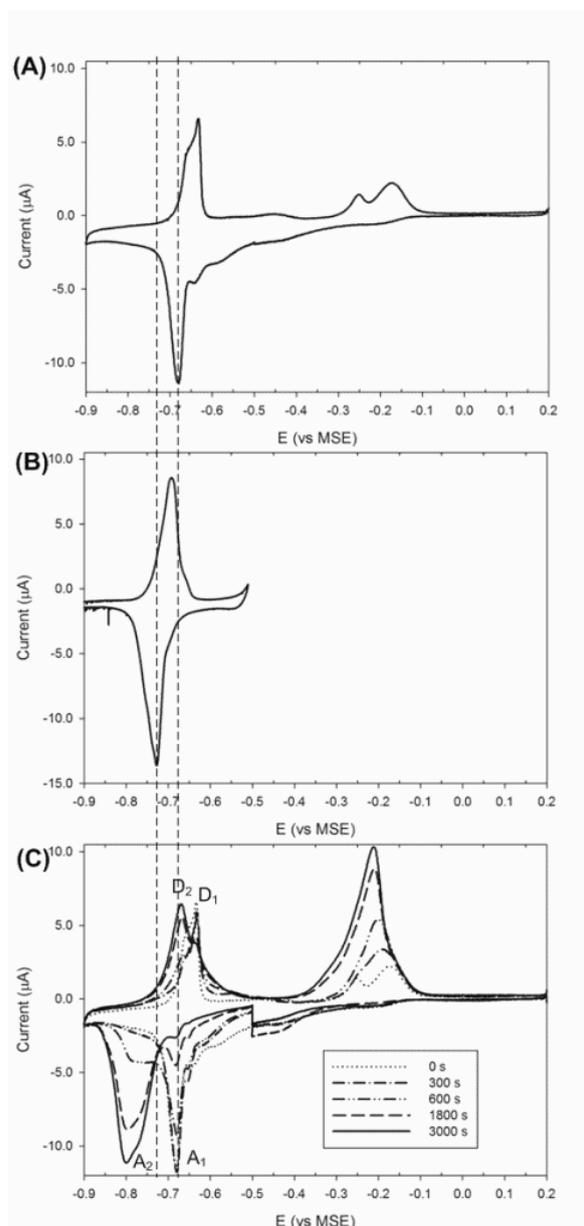
**Figure 1.** CVs for Pb upd in 10  $\mu\text{M}$   $\text{CuSO}_4$ , 5 mM  $\text{PbO}$ , and 0.1 M  $\text{H}_2\text{SO}_4$ : (a) on Au substrate (b) on Cu substrate (c) on Cu modified Au with various coverage of Cu by variation of  $t_{\text{Cu}}$ . Scan rate = 0.01 V/s.
