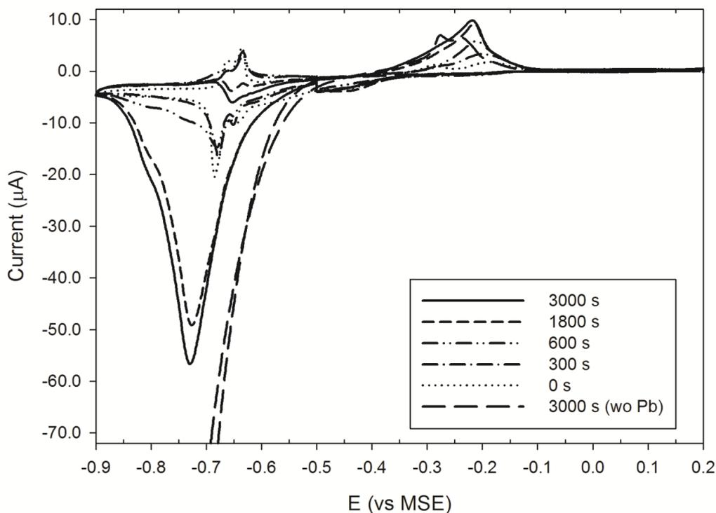
**Figure 2.** CVs for Pb upd in 10  $\mu\text{M}$   $\text{CuSO}_4$ , 5 mM  $\text{PbO}$ , 5 mM  $\text{NaNO}_3$  and 0.1 M  $\text{H}_2\text{SO}_4$  on Cu modified Au with various coverage of Cu by variation of  $t_{\text{Cu}}$ . As a control, CV without Pb in 10  $\mu\text{M}$   $\text{CuSO}_4$ , 5 mM  $\text{NaNO}_3$  and 0.1 M  $\text{H}_2\text{SO}_4$  was shown. Scan rate = 0.01 V/s.
