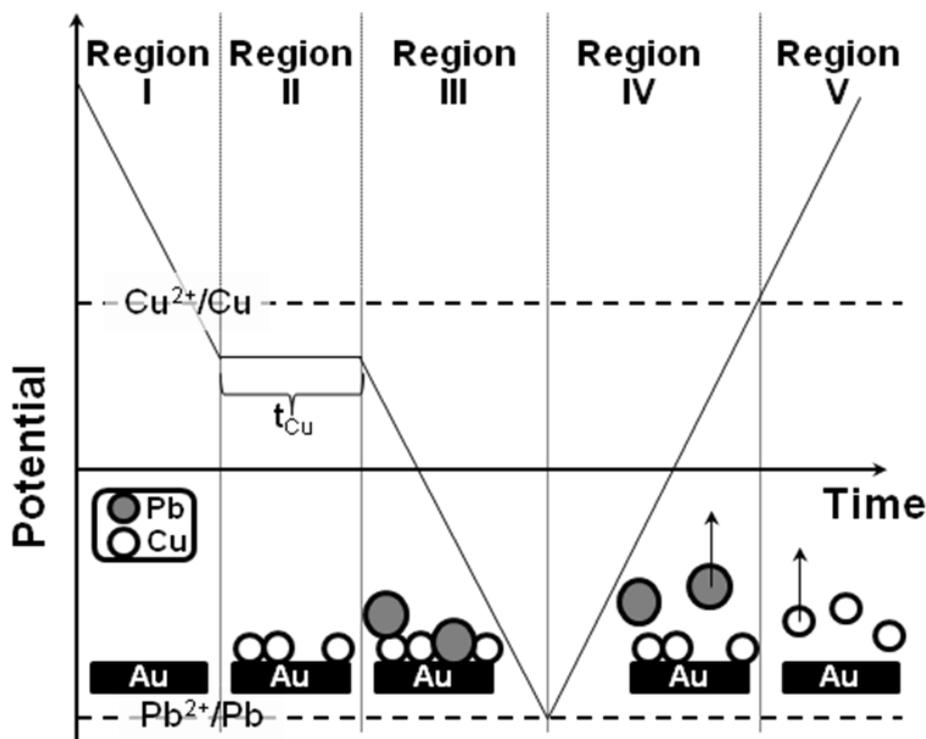
**Scheme 1.** Schematic potential program for dipping technique. In region II, the deposition of copper takes place under extremely diffusion controlled condition, so that the coverage of copper can be controlled by variation of  $t_{Cu}$ . Subsequent potential scan in region III and region IV enables adsorption and desorption of Pb up on Cu modified Au substrate, respectively. Continued potential scan desorbs copper adatoms indicating the coverage from charge.
