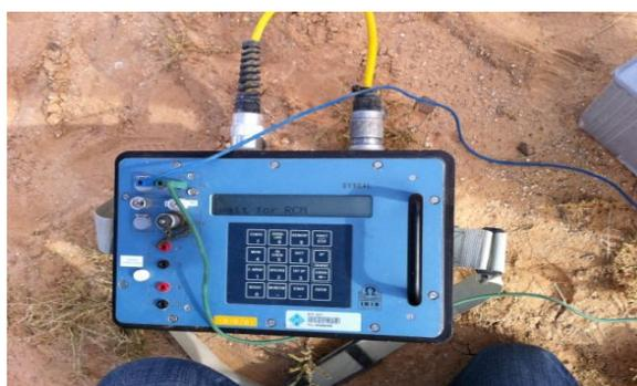
**Figure 3.** Syscal R1 Electrical Resistivity equipment.
