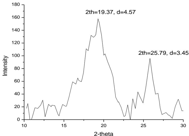
**Figure 4.** X-ray diffraction spectra of soot obtained from the Engine combustion of diesel
