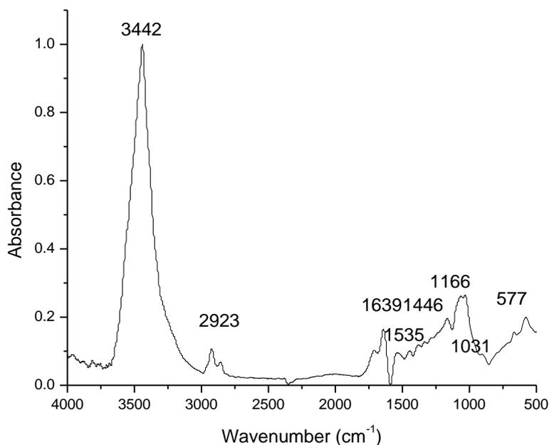
**Figure 5.** FTIR spectra of soot obtained from the Engine combustion of diesel
