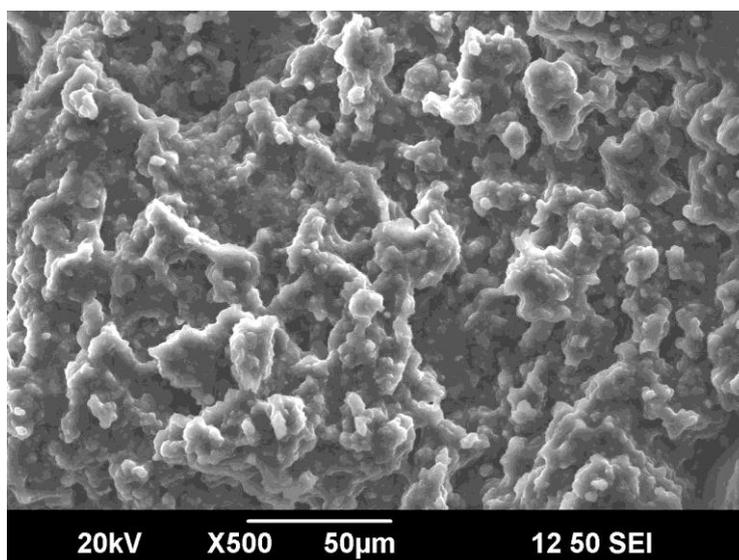
**Figure 1.** Scanning electron micrograph (SEM) of soot obtained from engine combustion of diesel ( $50\mu\text{m}$ )
