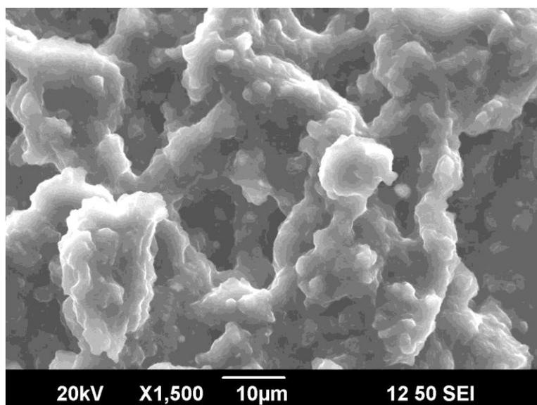
**Figure 2.** Scanning electron micrograph (SEM) of soot obtained from engine combustion of diesel ( $10\mu\text{m}$ )
