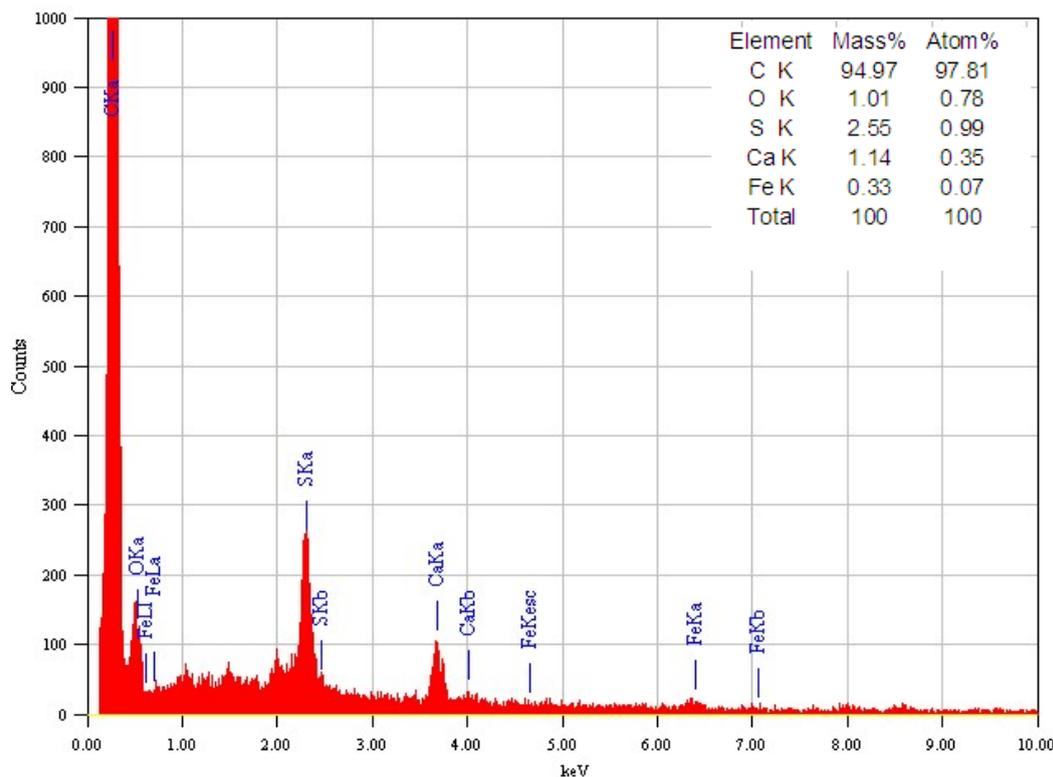
**Figure 3.** Energy dispersive spectroscopy (EDS) spectra of soot obtained from Engine combustion of diesel
