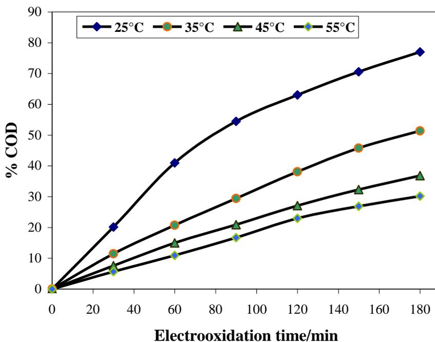
**Figure 9.** Influence of temperature on the decay of %COD during electro-oxidation of 50 mg/L cypermethrin on SnO<sub>2</sub> anode. Conditions: current density  $80 \text{mA cm}^{-2}$ ; pH=5.4; 2% (NaCl).
