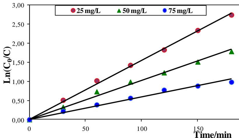
**Figure 8.** Linear regression for concentration removal with time during the electrochemical oxidation of cypermethrin on the SnO<sub>2</sub> anode for different concentrations.  $i_{app} = 80 \text{mAcm}^{-2}$ ; pH=4.5 and  $T=25^\circ\text{C}$ .
