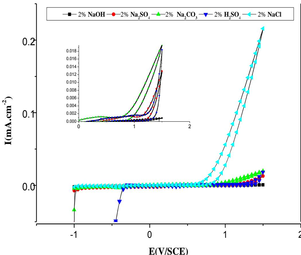
**Figure 2.** Voltammetric profiles of the SnO<sub>2</sub> electrode in different supporting electrolyte of cypermethrin 50 mg.L<sup>-1</sup>. Auxiliary electrode: platinum; reference electrode: SCE; scan rate: 10 mVs<sup>-1</sup>.
