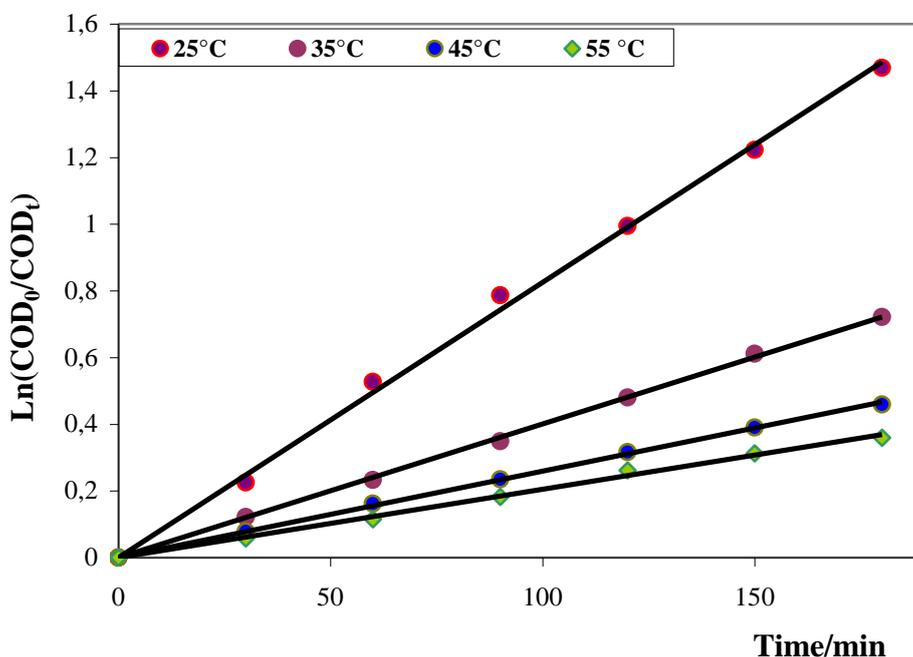
**Figure 10.** Pseudo first-order plot oxidation of cypermethrin 50 mg/L in 2% NaCl at 80 mA under different temperatures (COD at a given time, t during electrolysis).
