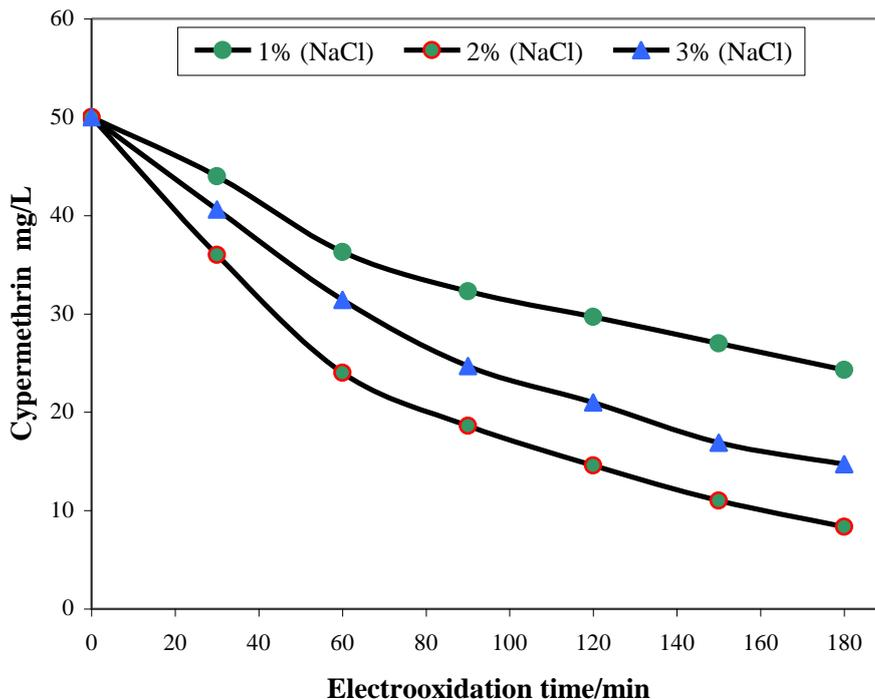
**Figure 4.** Evolution of concentration cypermethrin during the galvanostatic electrolyses of wastes polluted with 50 mg L<sup>-1</sup> of cypermethrin pesticide under effect of NaCl concentration. Operating conditions: T=25°C; pH 5.4; i=80 mA. cm<sup>-2</sup>.
