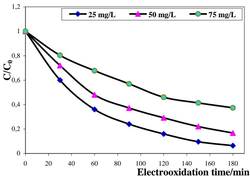
**Figure 7.** Influence of pesticide initial concentration on the normalized concentration cypermethrin during SnO<sub>2</sub>-anodic oxidation (Operating conditions: electrolyte = 2% NaCl, current density = 80 mAcm<sup>-2</sup>, T = 25°C, and pH=5.4).
