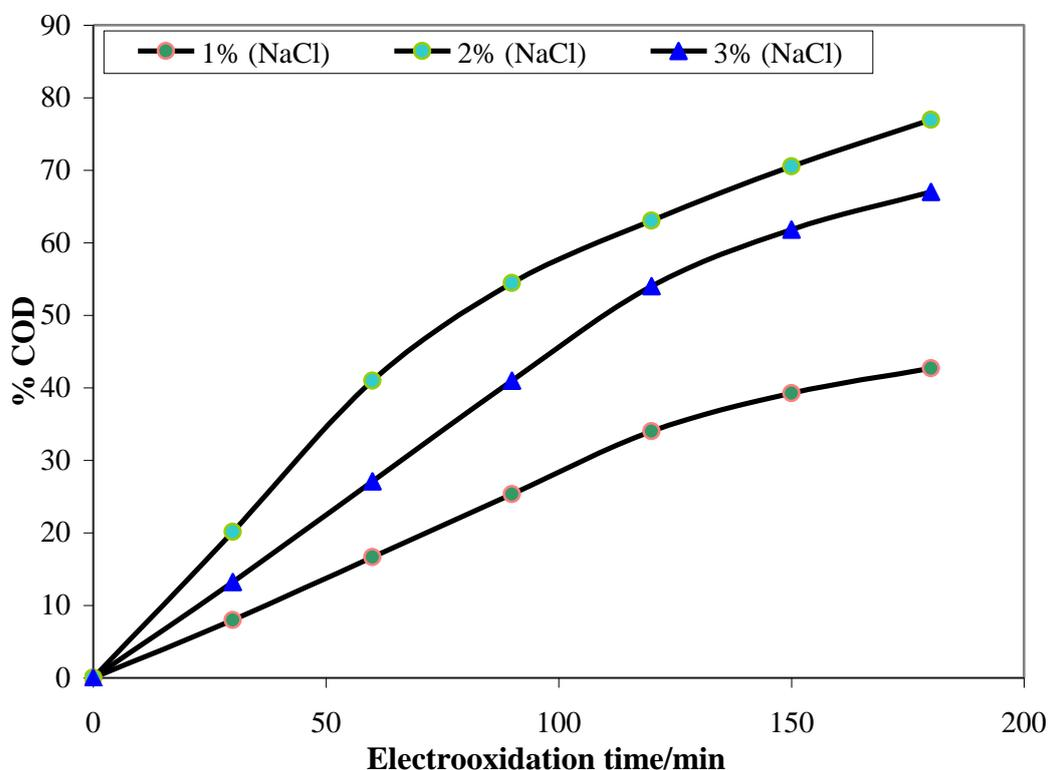
**Figure 3.** Direct electrooxidation at SnO<sub>2</sub> anode: effect of NaCl concentration on the %COD (50 mg.L<sup>-1</sup> cypermethrin solution, 80 mA.cm<sup>-2</sup>, pH=5.4, and T=25°C).
