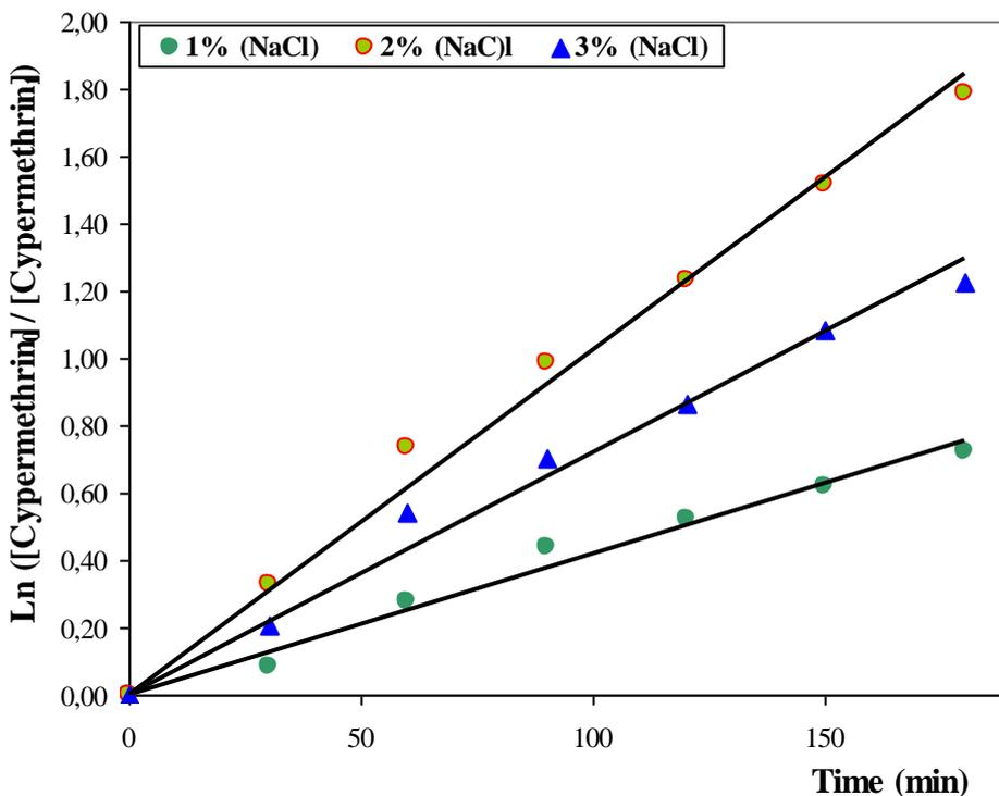
**Figure 5** apparent kinetic constants for oxidation of 50 mg/L Cypermethrin at 80 mA. cm<sup>-2</sup>, pH=5.4 and T=25°C.
