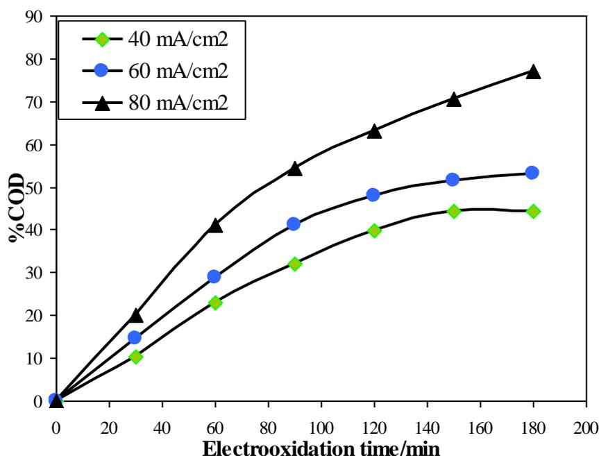
**Figure. 6** Influence of the applied current density on the trends of % COD electrolysis of cypermethrin (C<sub>0</sub> = 50 mg.L<sup>-1</sup>) using a 1cm<sup>2</sup> SnO<sub>2</sub> anode. pH=5.4 and T=25°C.
