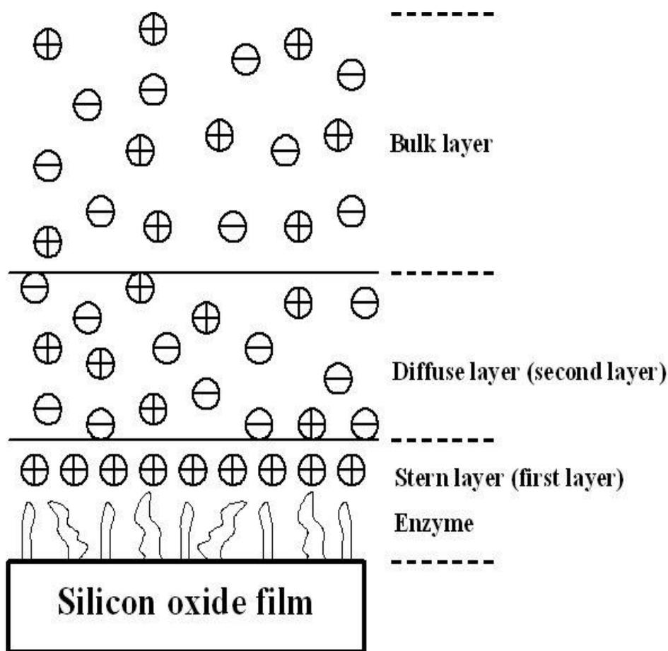
**Figure 7.** The surface diffusion model for the catalytic reaction of sulfotransferase.
