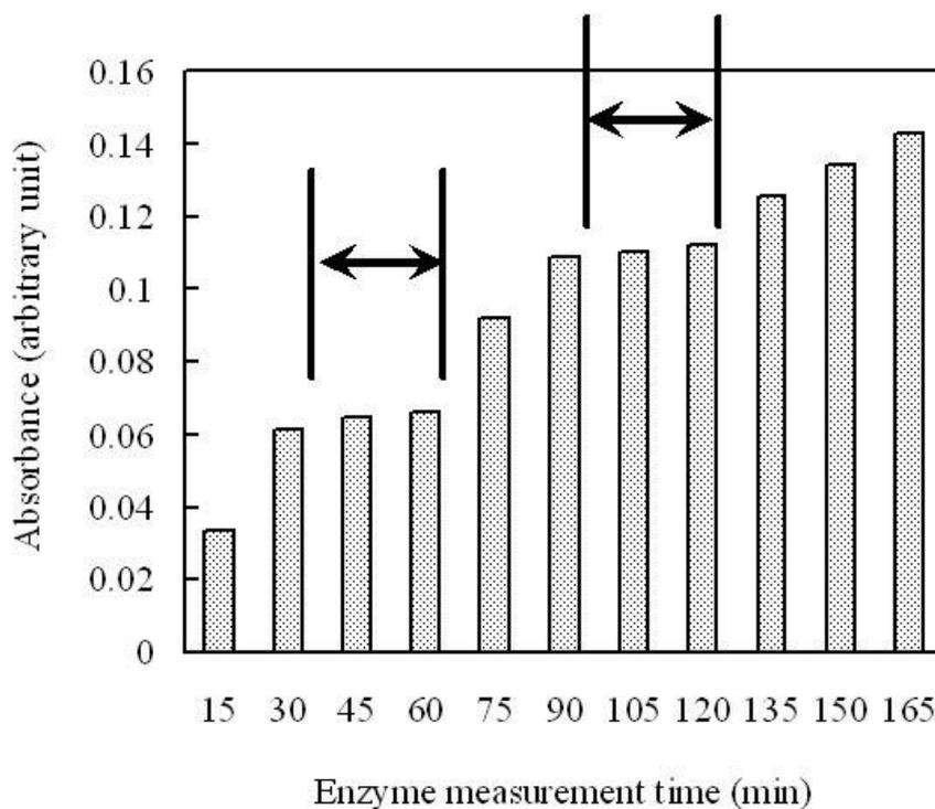
**Figure 8.** The absorbance of 4-nitrophenol at various measurement times for the sample with immobilization of sulfotransferase onto the silicon oxide surface,  $n=3$ . The marked area means the solution is removed from the home-made apparatus. The other samples are catalyzed by the sulfotransferase immobilized in the home-made apparatus.
