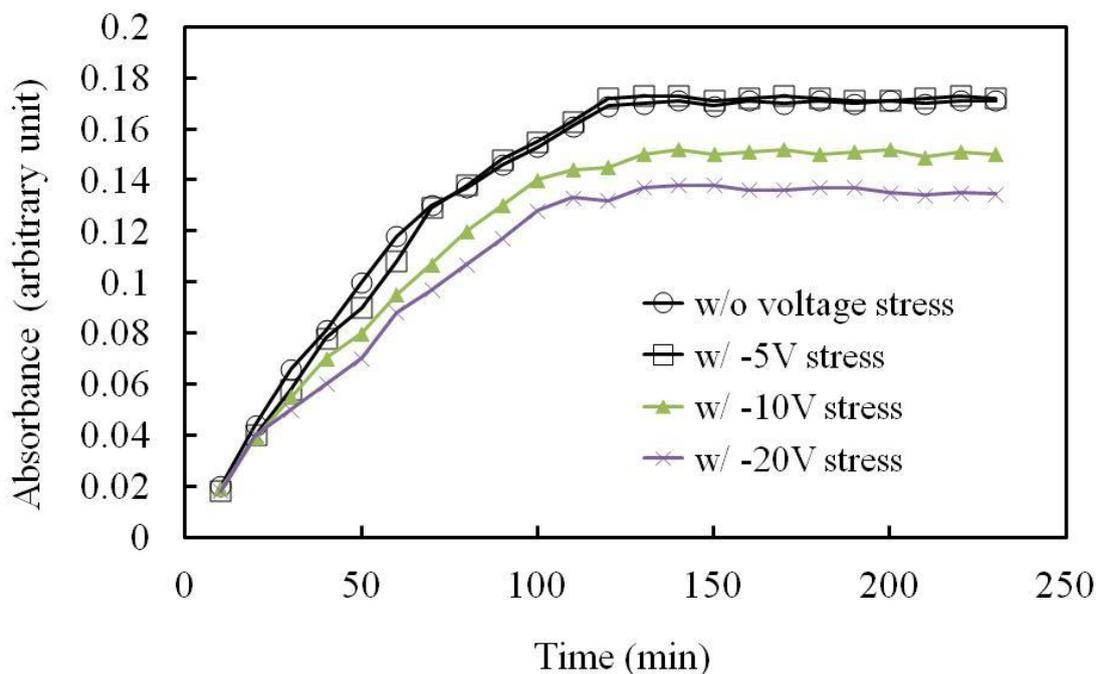
**Figure 9.** The effect of negative electric potential stress on the absorbance of 4-nitrophenol under various enzyme reaction times for sulfotransferase immobilizes onto the silicon oxide surface.
