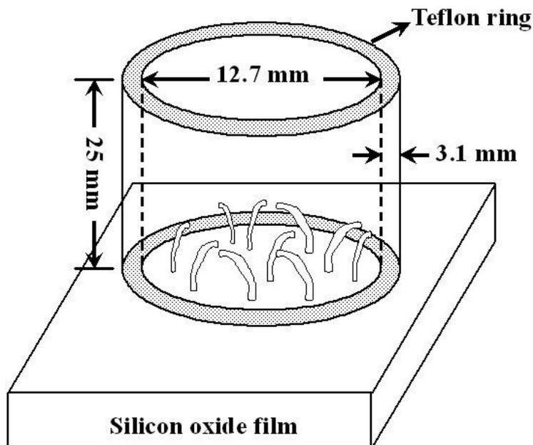
**Figure 1.** Schematic diagram of the home-made apparatus for immobilization of sulfotransferase onto the silicon oxide surface.
