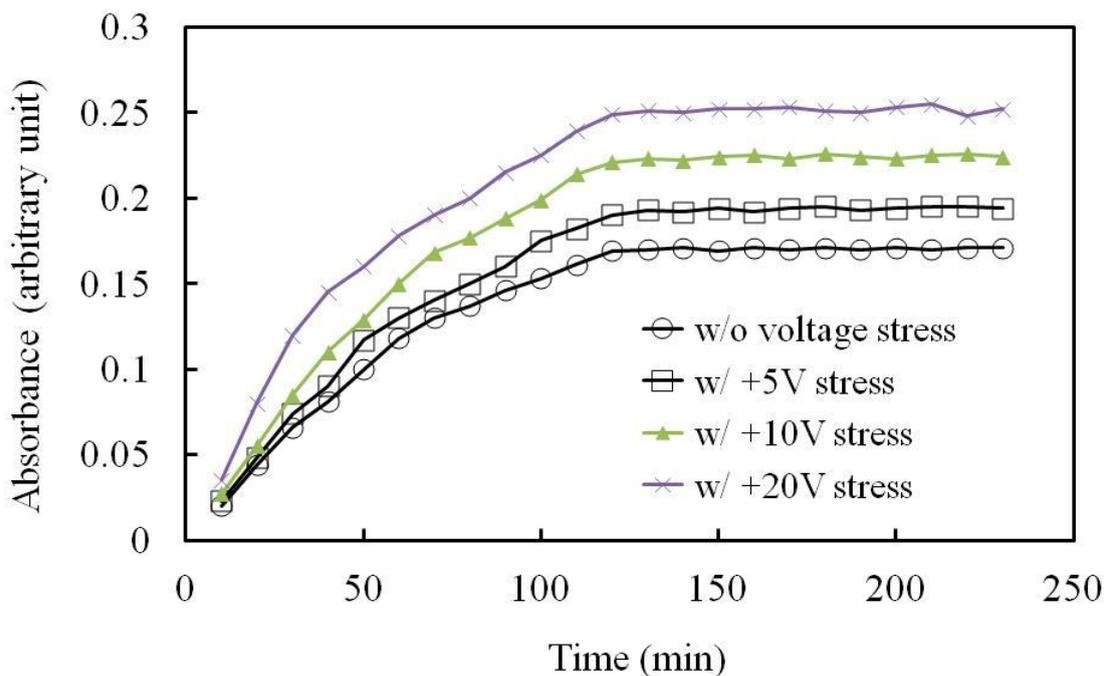
**Figure 10.** The effect of positive electric potential stress on the absorbance of 4-nitrophenol under various enzyme reaction times for sulfotransferase immobilizes onto the silicon oxide surface.
