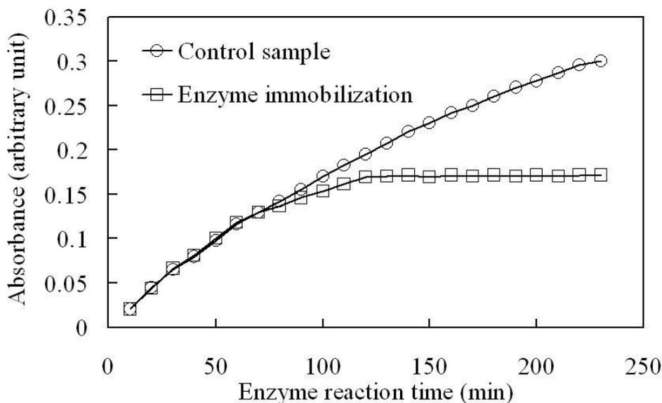
**Figure 6.** The absorbance of 4-nitrophenol at various enzyme reaction times for the control sample (sulfotransferase in solution) and the enzyme target sample (sulfotransferase immobilizes onto the silicon oxide surface),  $n=3$ .
