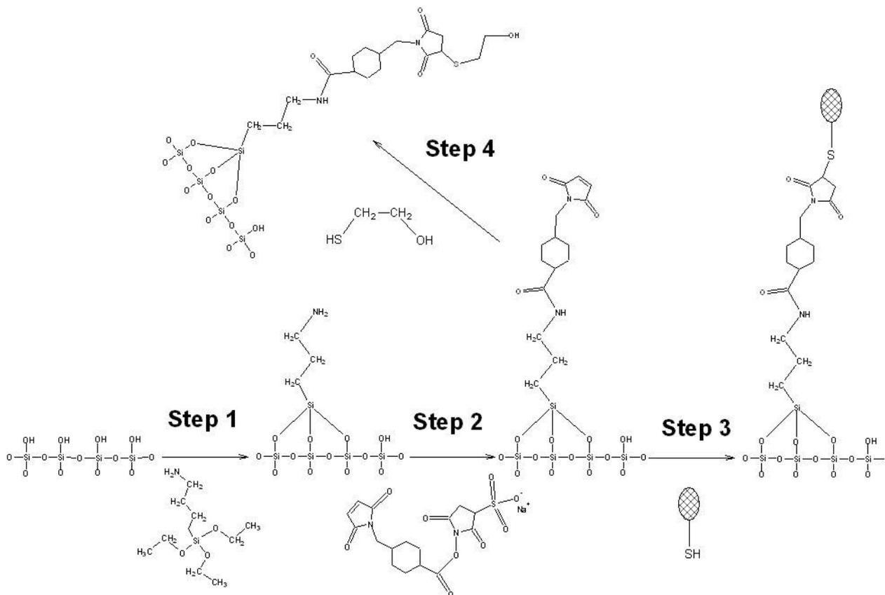
**Figure 4.** The immobilization steps for sulfotransferase onto silicon oxide surface.
