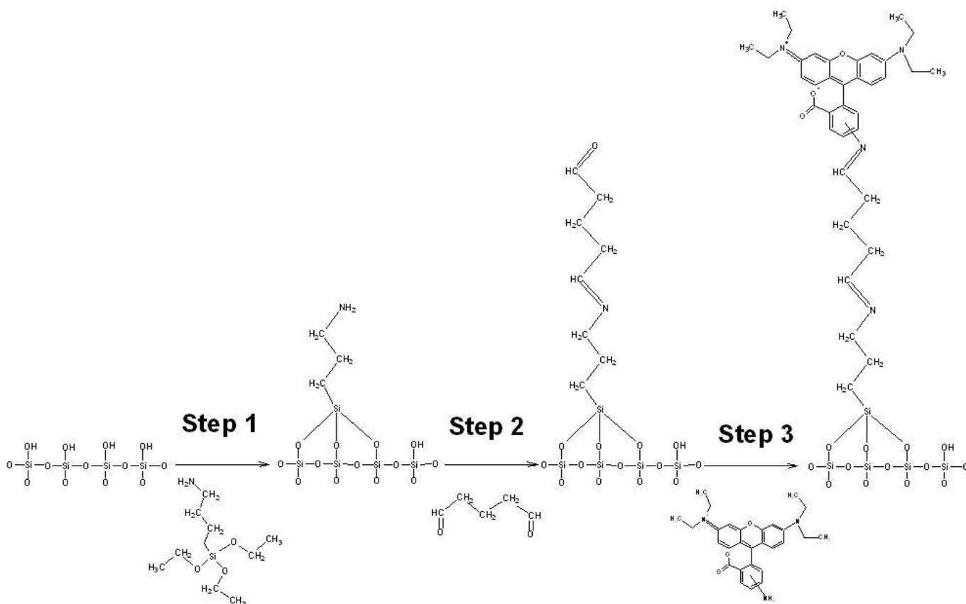
**Figure 2.** The immobilization steps for rhodamine B amine onto silicon dioxide surface.
