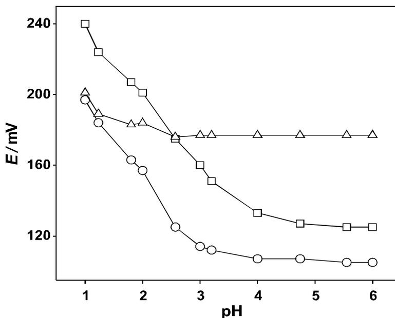
**Figure 4.** The effect of pH on the potentiometric response in  $1.0 \times 10^{-4}$  M of  $\text{Cu}^{2+}$  of the electrodes: A (○); B (□); C (△)
