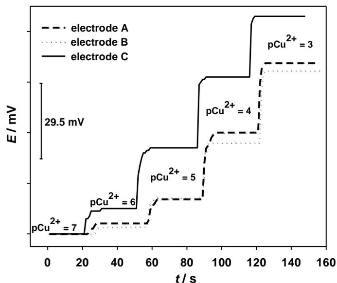
**Figure 5.** Dynamic response of electrodes on different concentration of  $\text{Cu}^{2+}$
