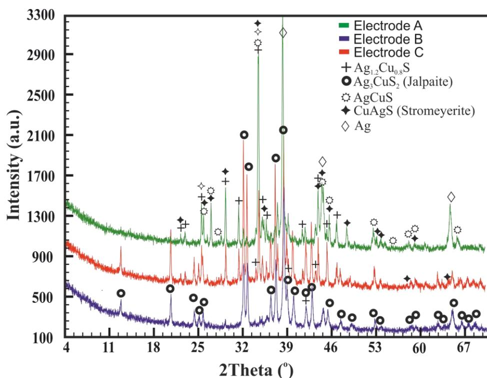
**Figure 1.** XRD pattern of prepared electroactive materials at different metal salts/sulfide mole ratio
