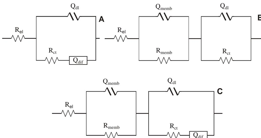
**Figure 7.** Equivalent electrical circuit models used for analysis
