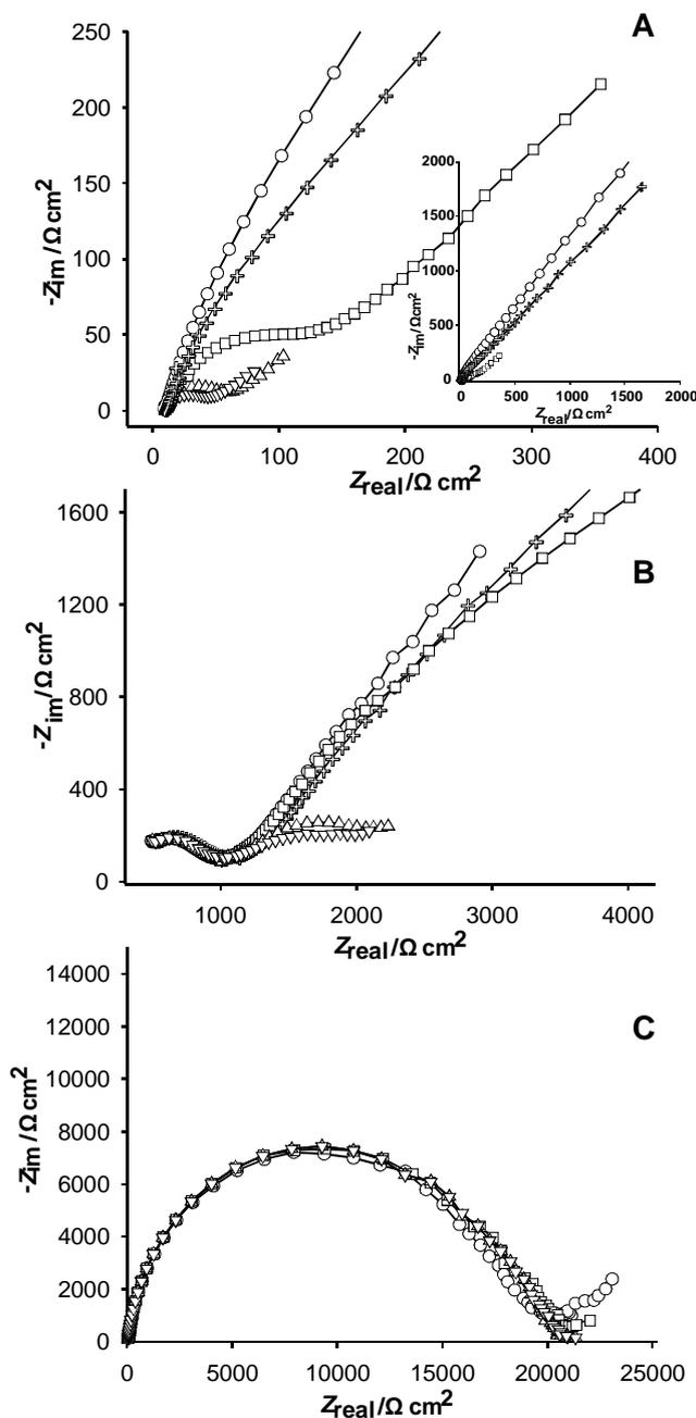
**Figure 6.** Impedance spectra, at obtained in: 0.1  $\text{KNO}_3$  ( $\circ$ ); 0.1  $\text{KNO}_3 + 10^{-5} \text{ M Cu}^{2+}$  ( $\square$ ); 0.1  $\text{KNO}_3 + 10^{-3} \text{ M Cu}^{2+}$  ( $\triangle$ ); 0.1  $\text{KNO}_3 + 10^{-2} \text{ M Cu}^{2+}$  ( $\nabla$ ); 0.1  $\text{KNO}_3$  immediately after measurement in  $10^{-2} \text{ M Cu}^{2+}$  ( $\oplus$ ), for electrodes A , B, C
