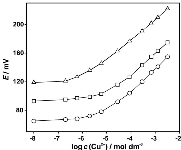
**Figure 2.** Calibration curves obtained by successive increasing of  $\text{Cu}^{2+}$  concentration for: electrode A ( $\circ$ ); electrode B ( $\square$ ); electrode C ( $\triangle$ )
