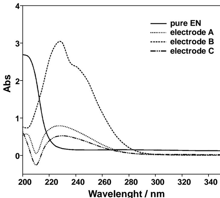
**Figure 3.** Absorption spectra of the EN solutions in which electrodes were been soaked for 2 hours.
