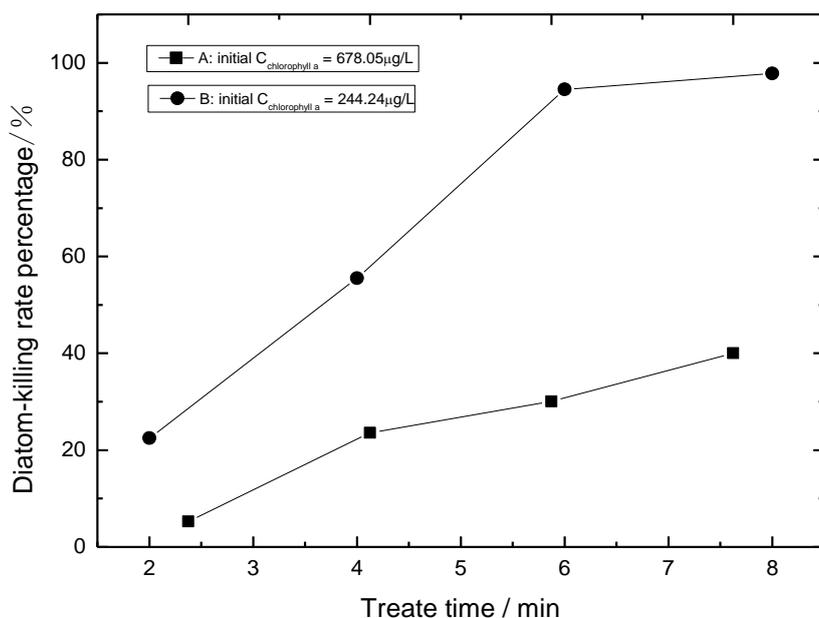
**Figure 5.** Effect of diatom concentration and electrolysis time on diatom-killing rate
