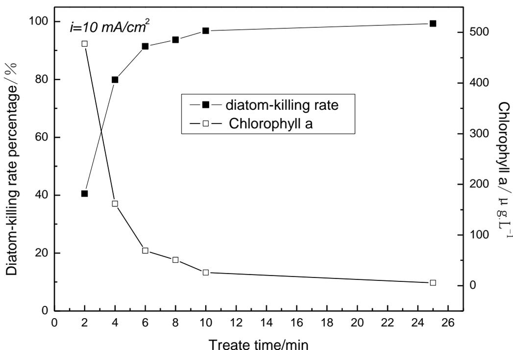
**Figure 2.** Effect of electrolysis time on diatom-killing rate
