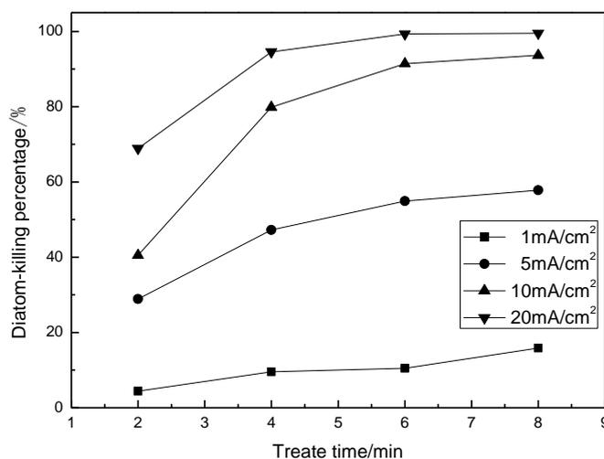
Figure 4. Effect of current density and electrolysis time on diatom-killing rate
