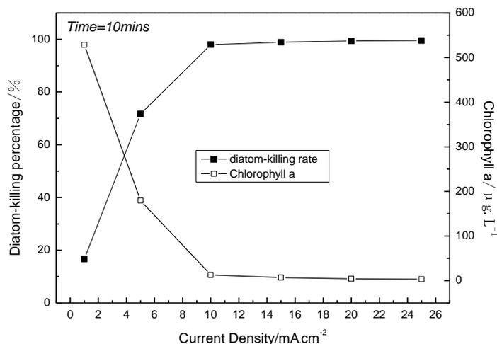
Figure 3. Effect of current density on diatom-killing rate
