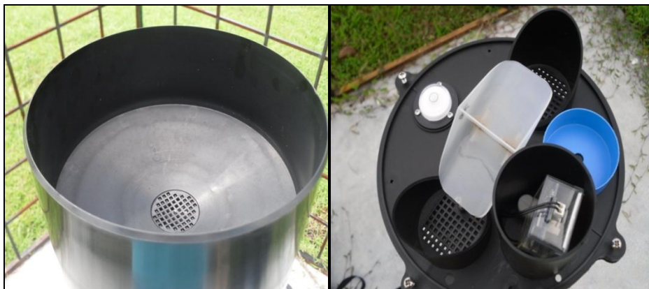
Figure 7. Rainlogger by Rainwise Inc.
