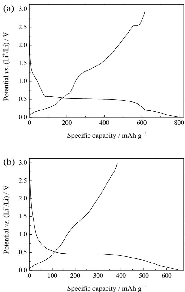
**Figure 5.** The first galvanostatic discharge-charge curve of (a) ZnO microrod array electrode and (b) ZnO microrod powder electrode at the same current density of 0.5 A g<sup>-1</sup>.
