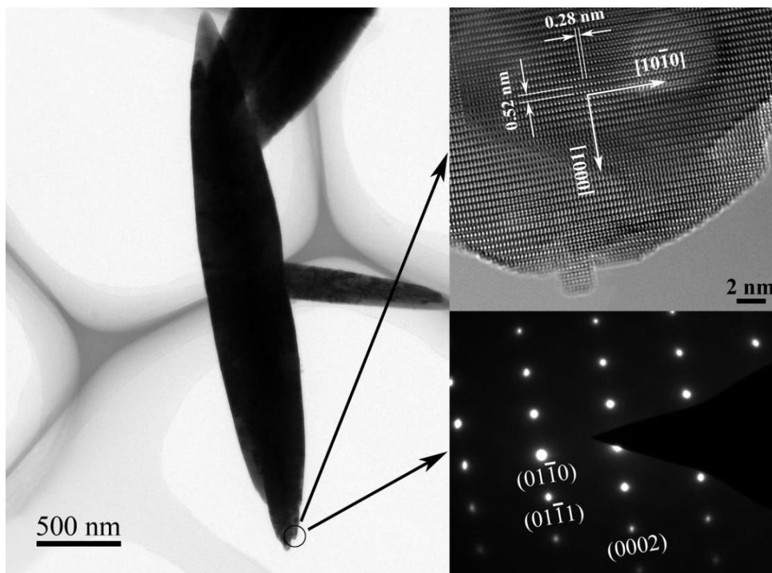
**Figure 3.** TEM results of a ZnO microrod, including an overall image of a single microrod, a high resolution image and the corresponding SAED pattern.
