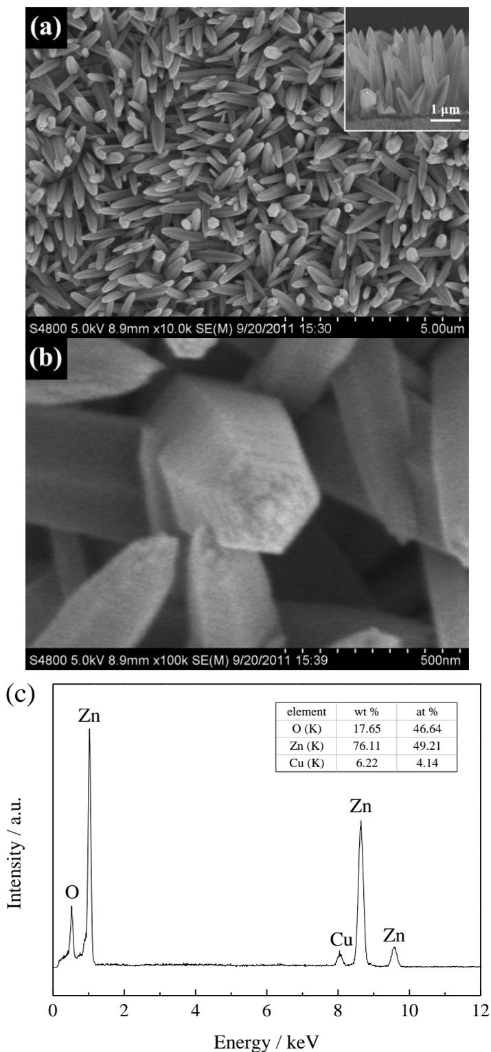
**Figure 2.** SEM results of the ZnO microrod array, (a) top-view image and the cross-sectional image, (b) the magnified image of a ZnO microrod, and (c) the EDS pattern of the ZnO microrod.
