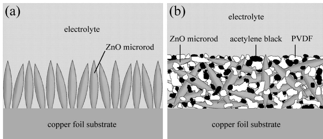
**Figure 6.** The structure diagrams of (a) ZnO microrod array electrode and (b) ZnO microrod powder electrode.
