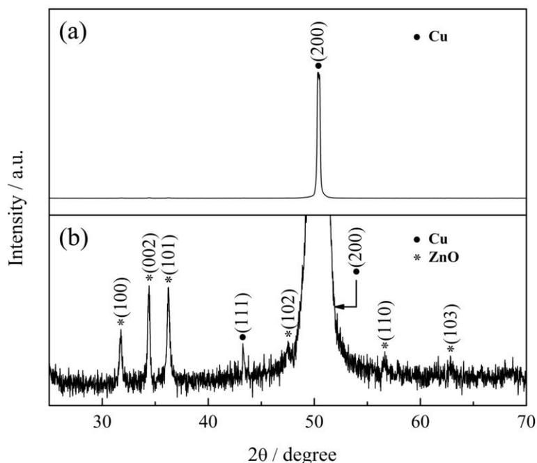
**Figure 1.** XRD pattern of ZnO microrod array deposited on copper foil, (a) the overall pattern, and (b) the magnified pattern.
