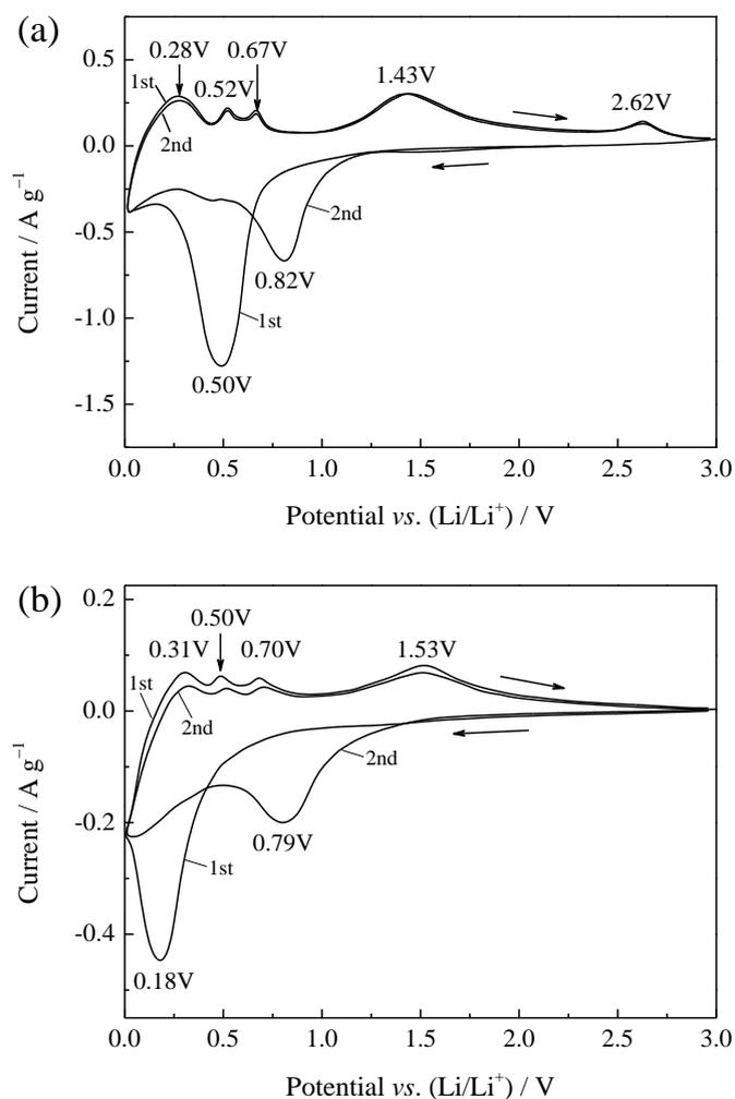
**Figure 4.** CV curves of (a) ZnO microrod array electrode and (b) ZnO microrod powder electrode at the sweep speed of  $0.1 \text{ mV s}^{-1}$ .
