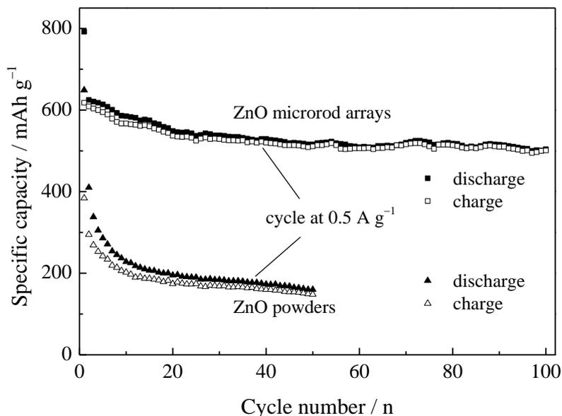
**Figure 7.** Cycling performance of the two electrodes at the same current density of  $0.5 \text{ A g}^{-1}$ .
