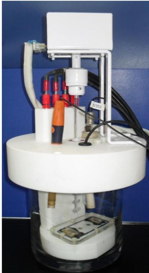
**Figure 2.** Galvanic Corrosion Cell
