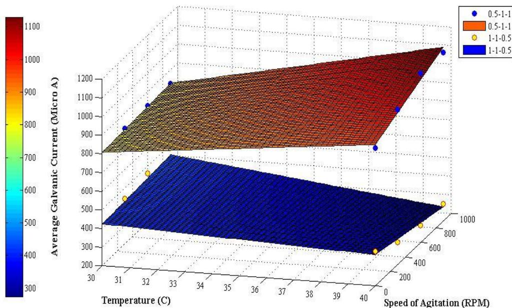
**Figure 5.** Surface response of Eqn (1&2) showing the average galvanic ( $I_g$ ) Vs. temperature ( $^{\circ}C$ ) and speed of agitation (RPM) for the area ratios (0.5:1:1) and (1:1:0.5)
