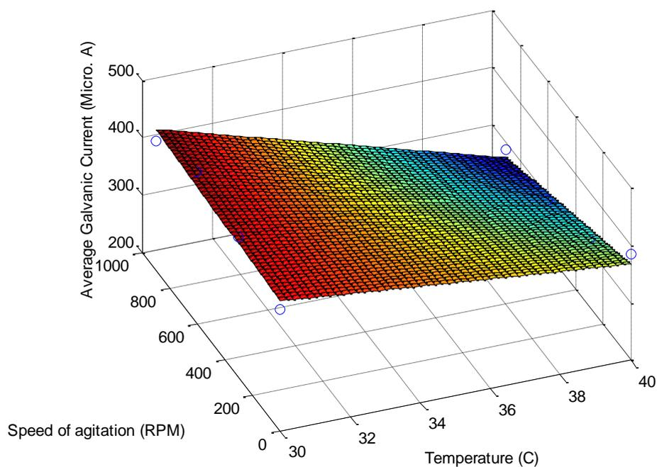
**Figure 4.** Surface response of Eqn (2) showing the average galvanic ( $I_g$ ) Vs. temperature ( $^{\circ}C$  ) and speed of agitation (RPM)
