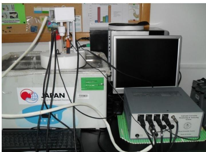
**Figure 1.** Galvanic Corrosion monitoring and analyzing system
