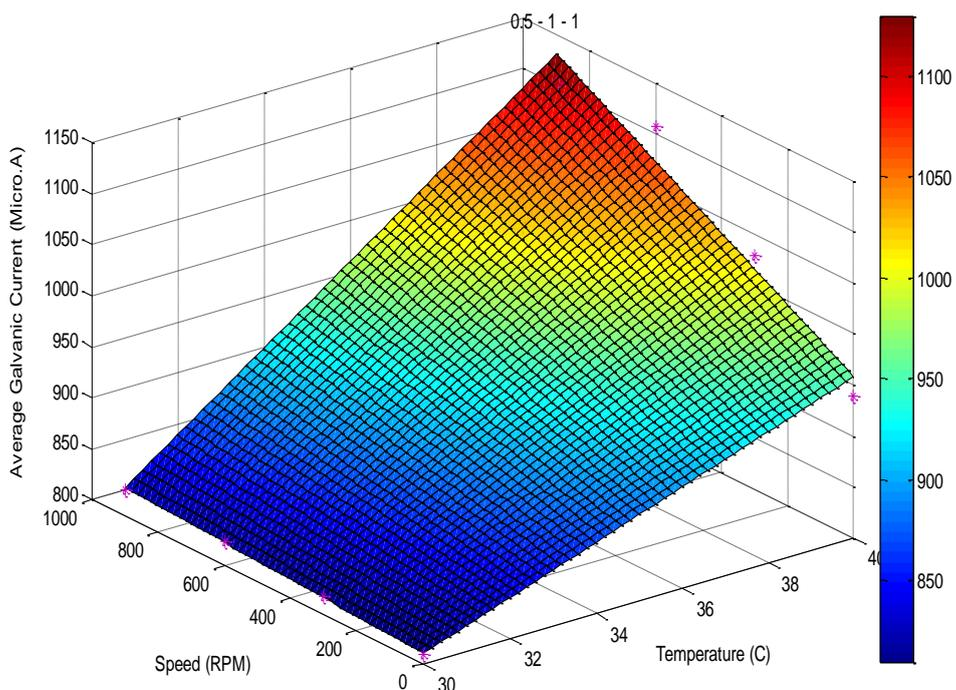
**Figure 3.** Surface response of Eqn (1) showing the average galvanic ( $I_g$ ) Vs. temperature ( $^{\circ}C$  ) and speed of agitation (RPM)
