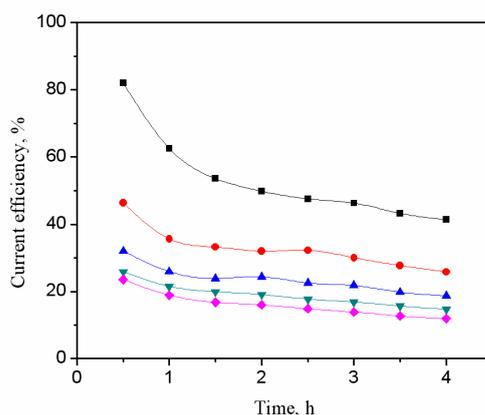
**Figure 7.** Current efficiency for current densities with electrolysis time at initial pH 13. (■) 10 mA cm<sup>-2</sup>; (●) 20 mA cm<sup>-2</sup>; (▲) 30 mA cm<sup>-2</sup>; (▼) 40 mA cm<sup>-2</sup>; (◆) 50 mA cm<sup>-2</sup>. [CN<sup>-</sup>]<sub>0</sub> = 250 mg/L; flow rate = 80 L/h.
