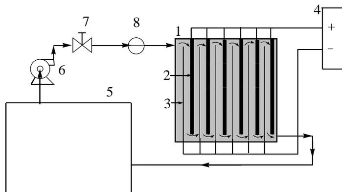
**Figure 1.** Schematic diagram of the experimental setup. (1) electrochemical cell; (2) anodes; (3) cathodes; (4) controlled DC unit; (5) reservoir; (6) pump; (7) flow regulator; (8) flow meter
