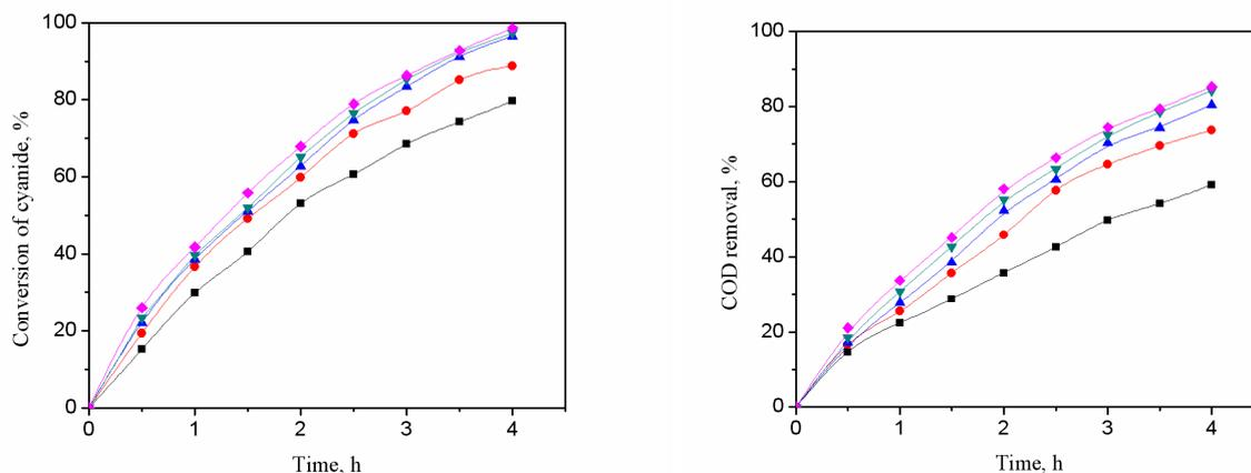
**Figure 6.** Effect of current density on the conversion of cyanide and COD removal with electrolysis time at initial pH 13. (■) 10 mA cm<sup>-2</sup>; (●) 20 mA cm<sup>-2</sup>; (▲) 30 mA cm<sup>-2</sup>; (▼) 40 mA cm<sup>-2</sup>; (◆) 50 mA cm<sup>-2</sup>. [CN<sup>-</sup>]<sub>0</sub> = 250 mg/L; flow rate = 80 L/h.
