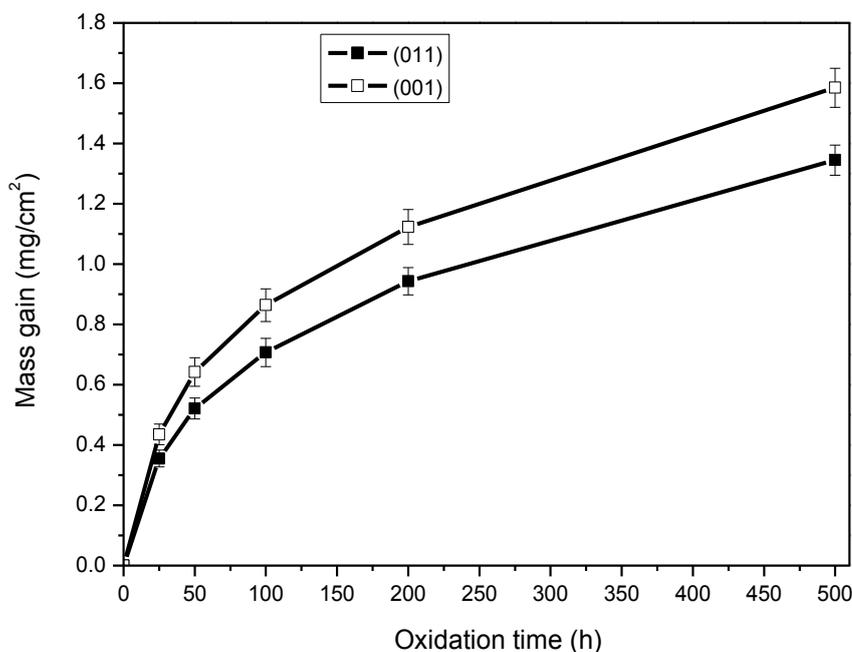
**Figure 3.** Oxidation kinetics curve of Ni-base single crystal superalloy CM186LC.
