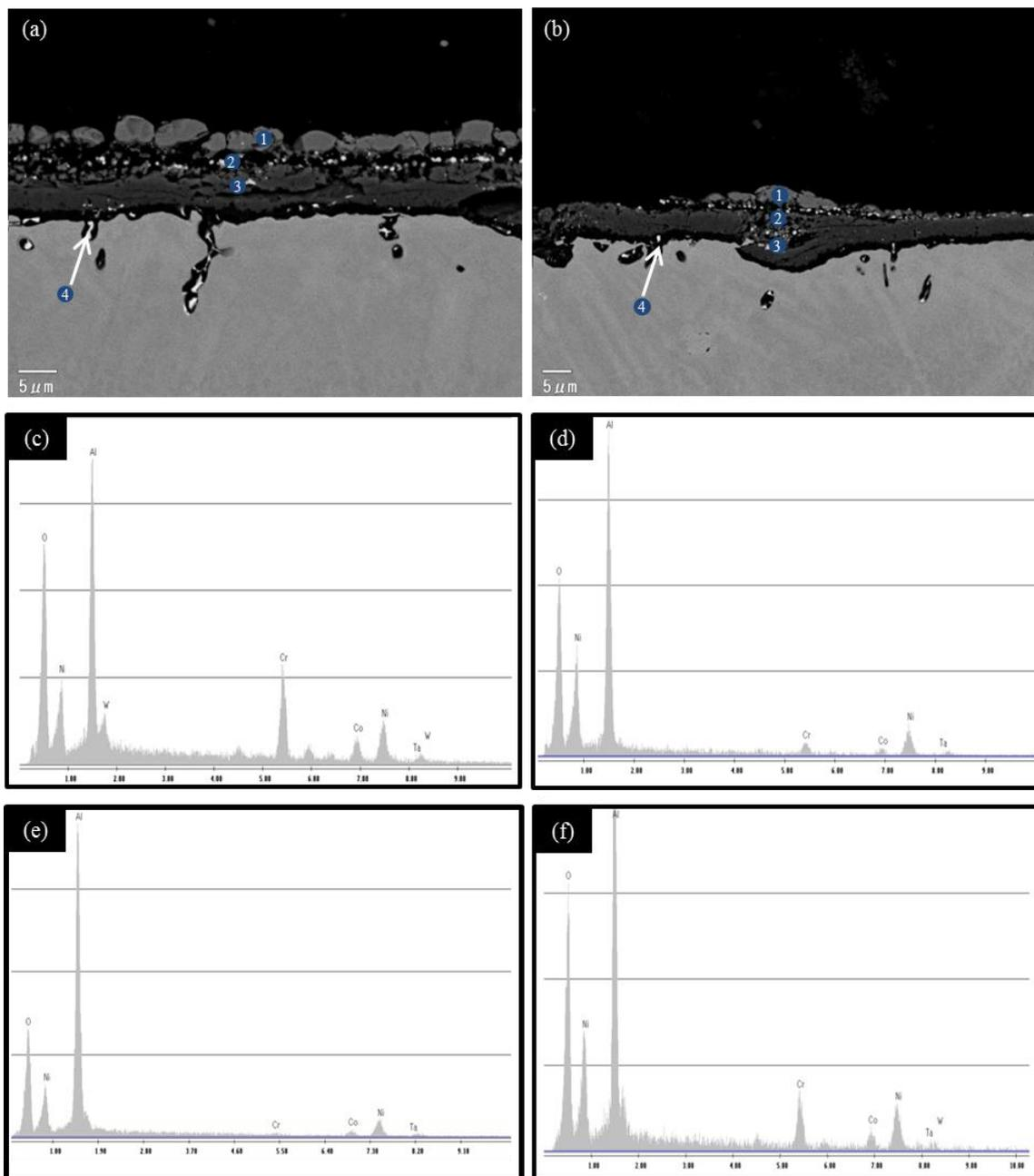
**Figure 9.** Cross-sectional SEM images of Ni-base single crystal superalloy CM186LC after 500 h oxidation at 1100°C: (a) (001) surface and (b) (011) surface; (c) to (f) represent the corresponding EDX profile analysis derived from the intermediate layer (points 2 and 3): (c) and (e) for micrograph shown in (a) whereas (d) and (f) for micrograph shown in (b).
