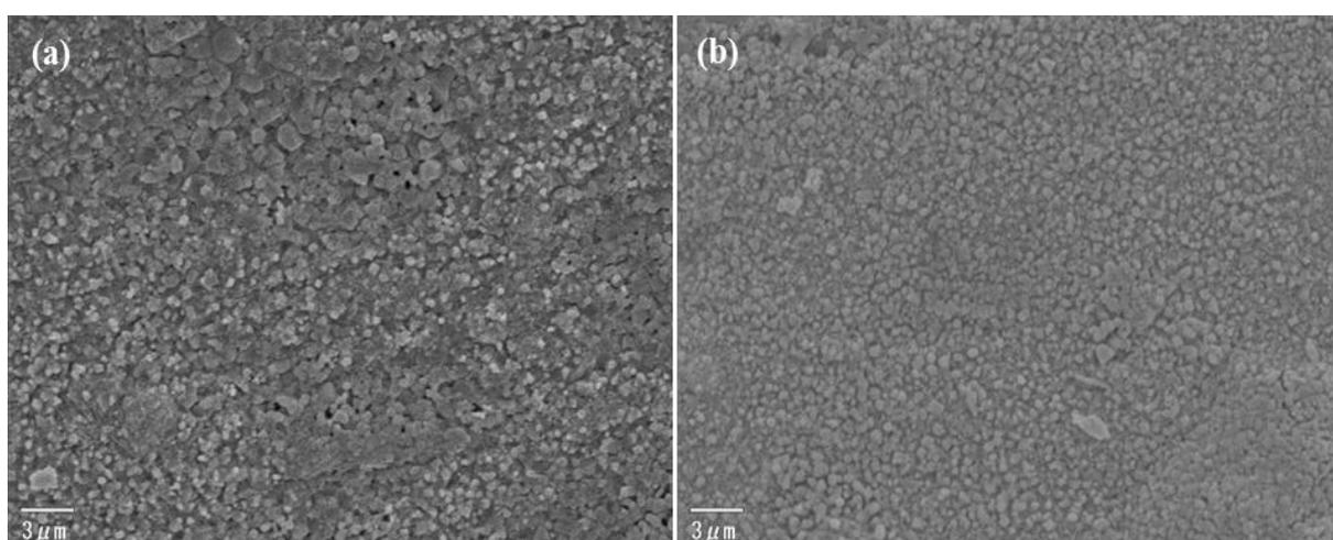
**Figure 7.** Surface morphologies of Ni-base single crystal superalloy CM186LC after 100 h oxidation at 1100°C for: (a) (001) surface and (b) (011) surface.
