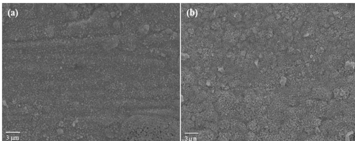
**Figure 6.** Surface morphologies of Ni-base single crystal superalloy CM186LC after 25 h oxidation at 1100°C for: (a) (001) surface and (b) (011) surface.
