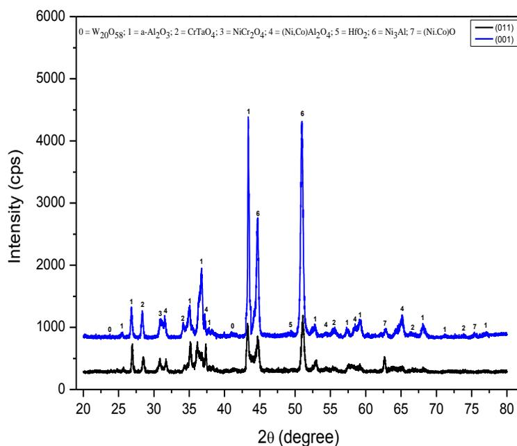
**Figure 5.** XRD patterns of Ni-base single crystal superalloy CM186LC after 500 h oxidation at  $1100^\circ\text{C}$ .
