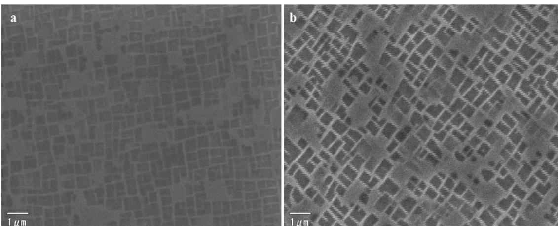
**Figure 2.** SEM micrographs of Ni-base single crystal superalloy CM186LC: (a) (001) surface and (b) (011) surface.
