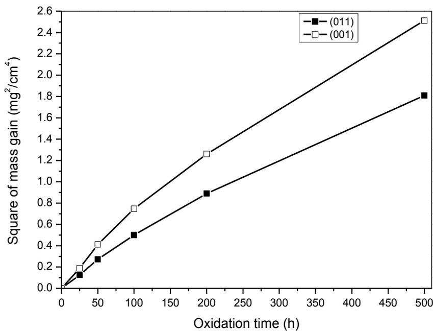
**Figure 4.** Square of the mass gain per unit area vs oxidation time for Ni-base single crystal superalloy CM186LC after oxidation in air at 1100°C.
