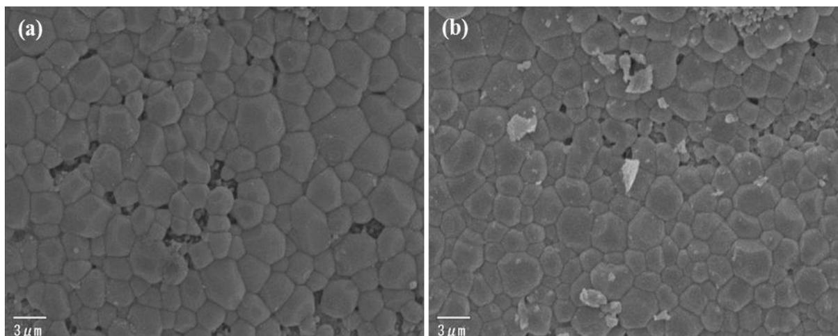
**Figure 8.** Surface morphologies of Ni-base single crystal superalloy CM186LC after 500 h oxidation at 1100°C for: (a) (001) surface and (b) (011) surface.
