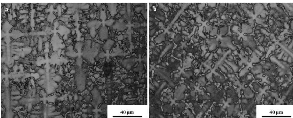
**Figure 1.** Optical micrographs of Ni-base single crystal superalloy CM186LC: (a) (001) surface and (b) (011) surface.
