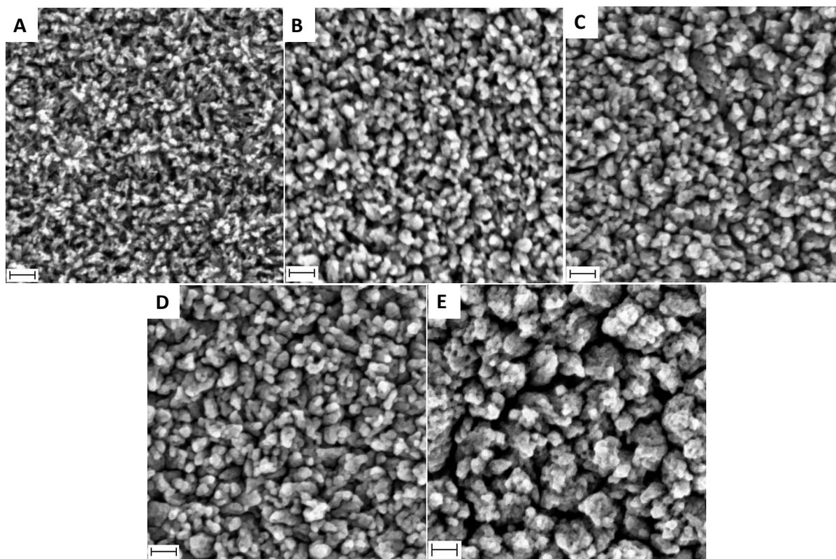
**Figure 1.** FESEM surface micrograph of ZnO nanorod prepared by seed mediated method via multiple growth steps, A) 1× growth step, B) 2× growth steps, C) 3× growth steps, D) 4× growth steps and E) 5× growth steps. Scala bar 100 nm
