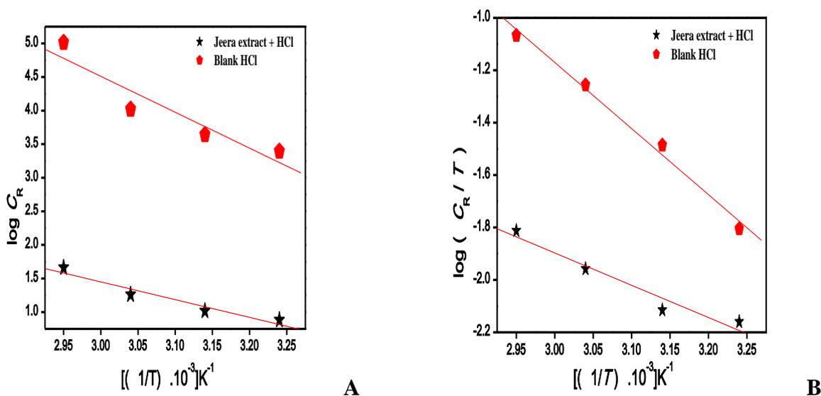
**Figure 5.** Arrhenius plots for (a)  $\log C_R$  versus  $1/T$  (b)  $\log C_R/T$  versus  $1/T$
