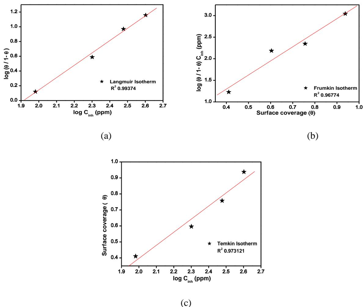
**Figure 6.** (a) Langmuir (b) Frumkin and (c) Temkin adsorption isotherm plots for the adsorption of Jeera (*Cuminum Cyminum*) seed extract on the surface of mild steel
