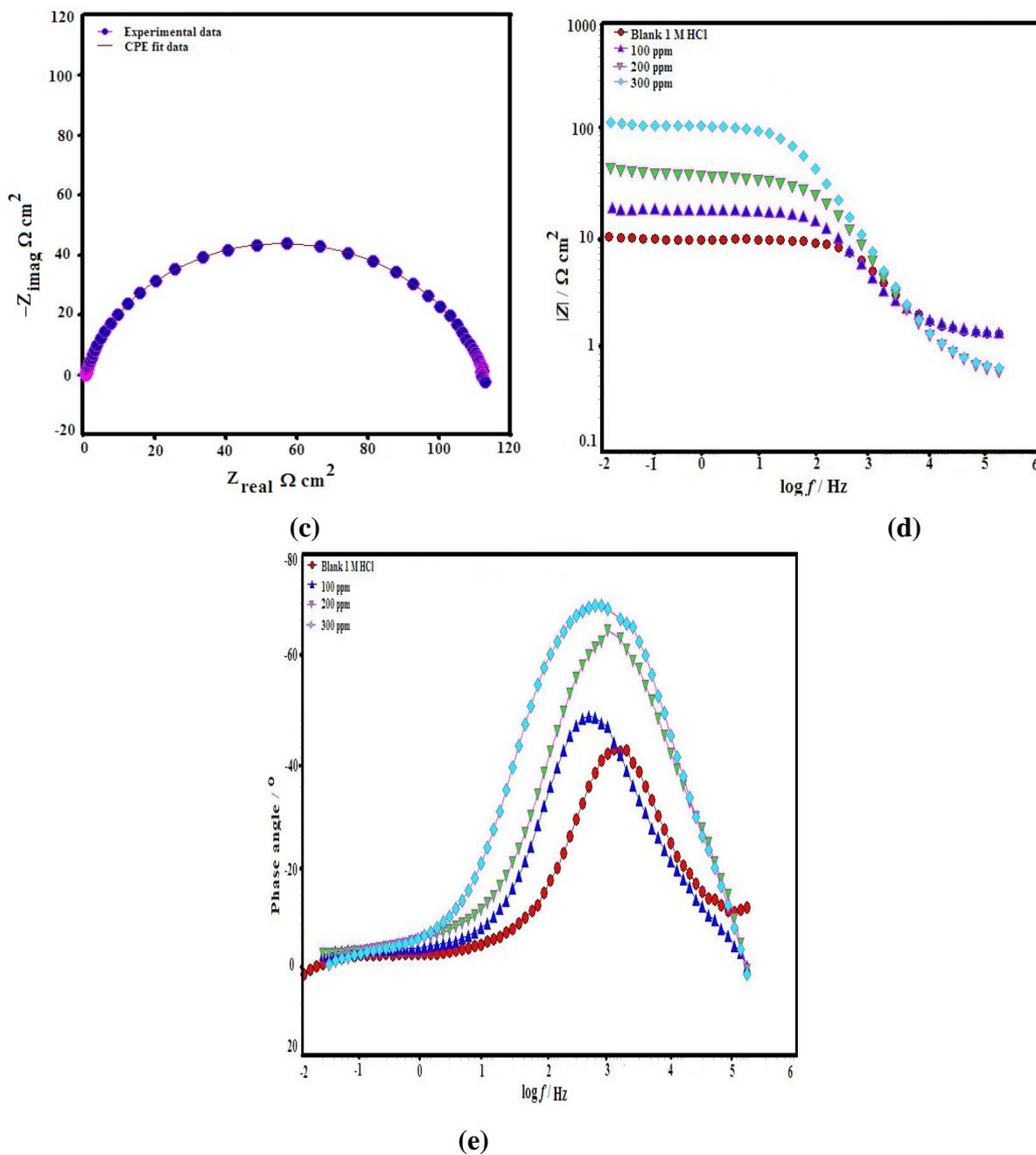
**Figure 2.** (a) Nyquist plots of mild steel in 1 M HCl in absence and presence of different concentrations of Jeera (*Cuminum Cyminum*) seed extract (b) equivalent circuit used to fit the impedance data (c) Nyquist plot with CPE fit data (d) Bode plot and (e) Phase angle plot
