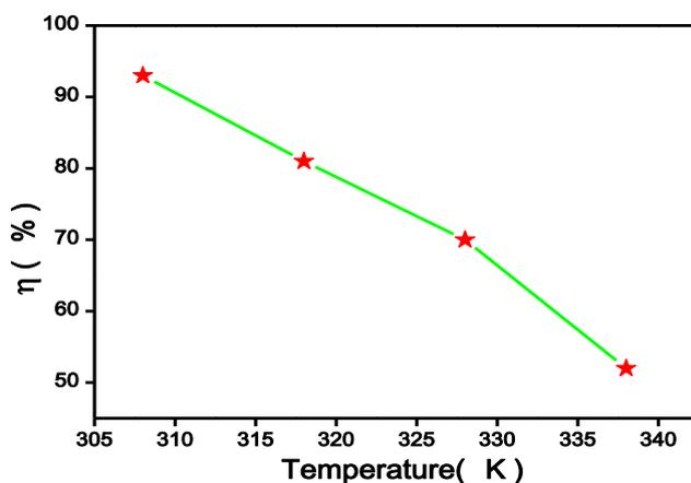
**Figure 4.** Inhibition efficiency of Jeera (*Cuminum Cyminum*) seed extract at different temperatures
