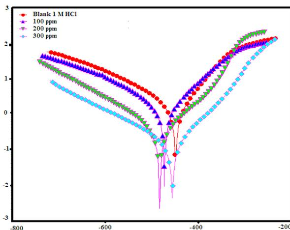
**Figure 3.** Tafel polarization curves for corrosion of mild steel in 1 M HCl in the absence and presence of different concentrations of Jeera (*Cuminum Cyminum*) seed extract
