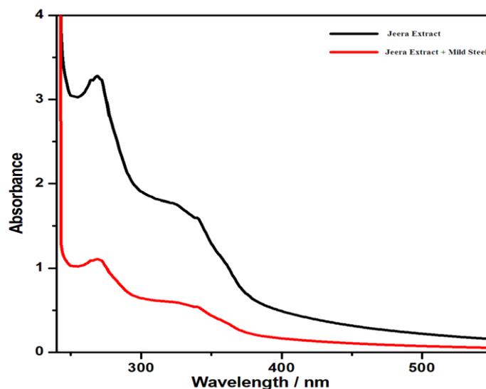
**Figure 7.** UV-Visible spectroscopy with Jeera extract before and after 5 hours immersion of mild steel
