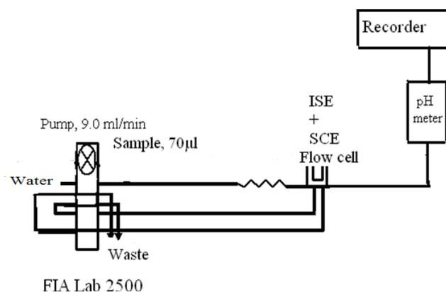
**Figure 1.** Schematic diagram of the flow injection system used in the measurements.
