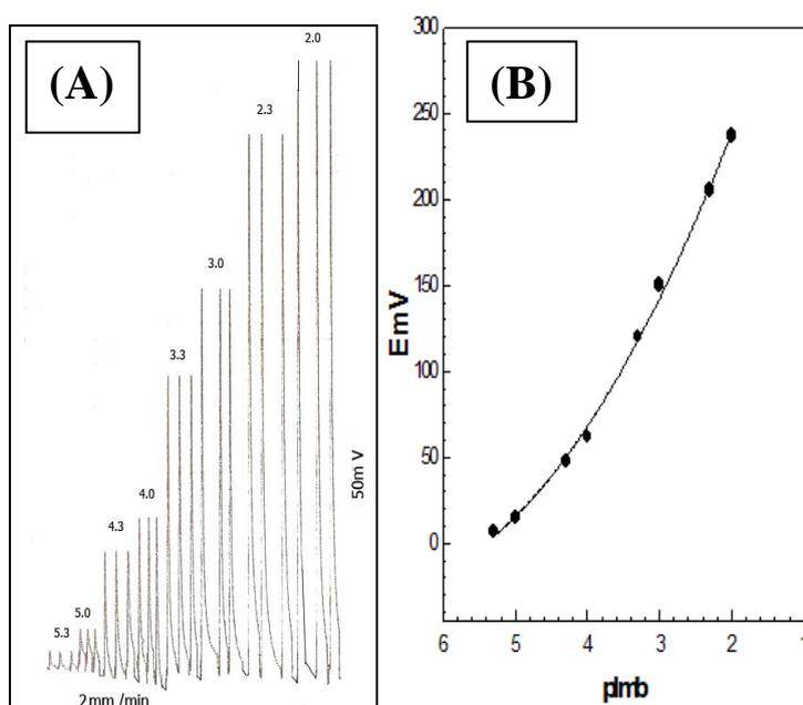
**Figure 2.** The recordings obtained for the flow rate 9.00 mL/min (A) and its corresponding calibration curve (B) on using Imb-TPB electrode.
