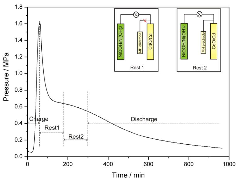
**Figure 5.** The profile of changes of internal pressure over time when a modified Ni-Cd cell with a separated alloy electrode was charged at 2C for 60 minutes, and first rested for 120 minutes. Then the alloy electrode was connected to the negative electrode. After rested for 180 minutes, the cell was discharged at 0.5C down to 1.0 V. Inset: Schematic electrode connection in the modified conventional Ni-Cd cell.
