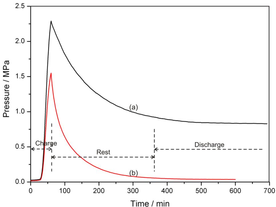
**Figure 1.** The profiles of changes of internal pressure over time when the conventional (a) and improved (b) Ni-Cd cells were charged at 2C for 60 minutes, rested for 300 minutes and then discharged at 0.5C down to 1.0 V.
