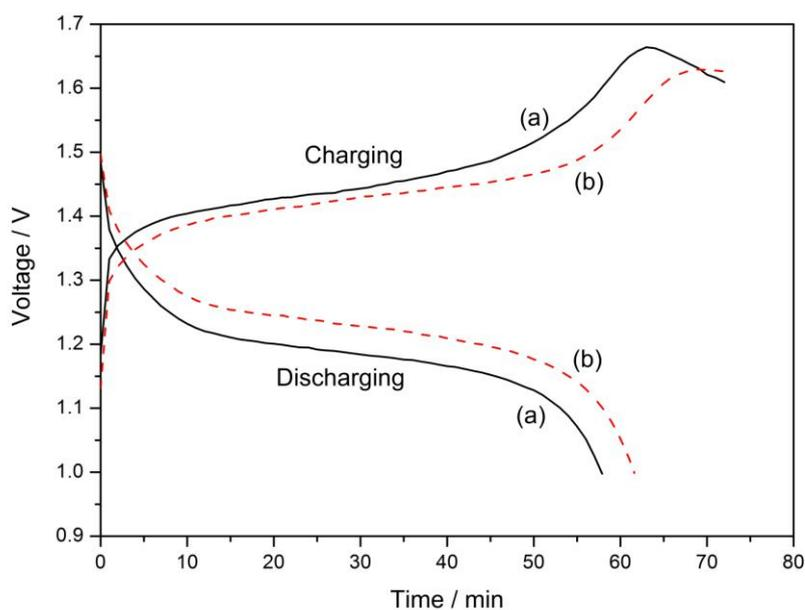
**Figure 7.** The charge/discharge voltage curves of the conventional (a) and improved (b) Ni-Cd cells at the 150<sup>th</sup> cycle.
