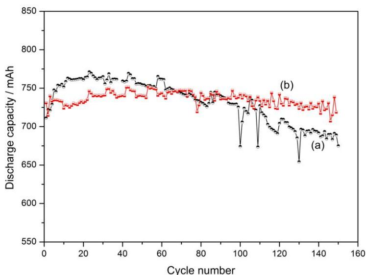
**Figure 6.** Cycling characteristics of the conventional (a) and improved (b) Ni-Cd cells. Ni-Cd cells were charged at 1C for 72 minutes and discharged at 1C down to 1.0 V.
