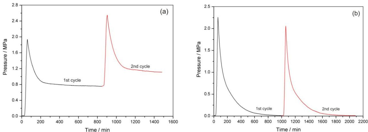
**Figure 2.** Changes of internal pressure over time when the conventional (a) and the improved (b) Ni-Cd cells were cycled at the following regime: charged at 2C for 60 minutes, then rested for 300 minutes and discharged at 0.5C down to 1.0 V.
