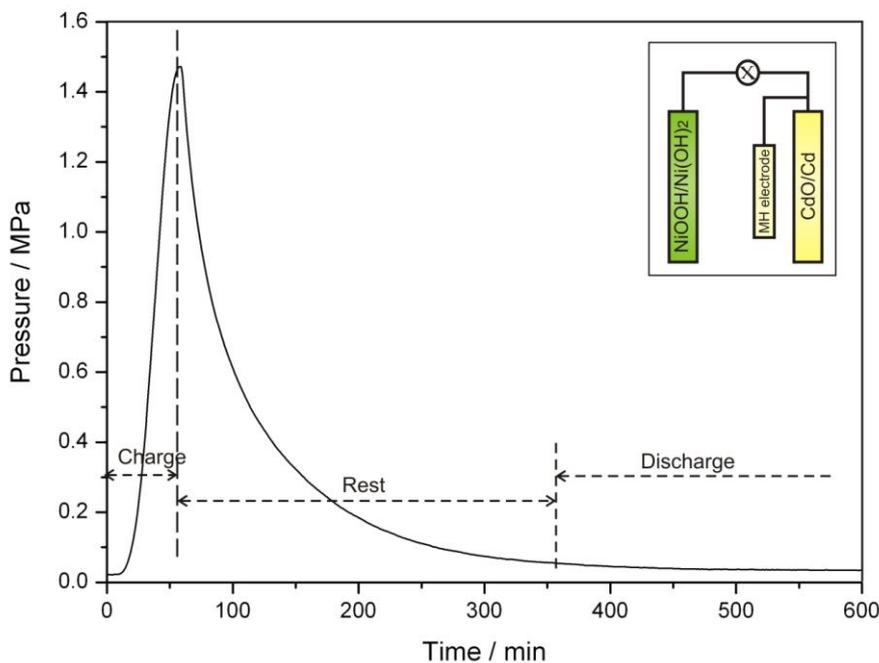
**Figure 3.** The profile of changes of internal pressure over time when a modified conventional Ni-Cd cell was charged at 2C for 60 minutes, rested for 300 minutes and then discharged at 0.5C down to 1.0 V. Inset: Schematic electrode connection in the modified conventional Ni-Cd cell.
