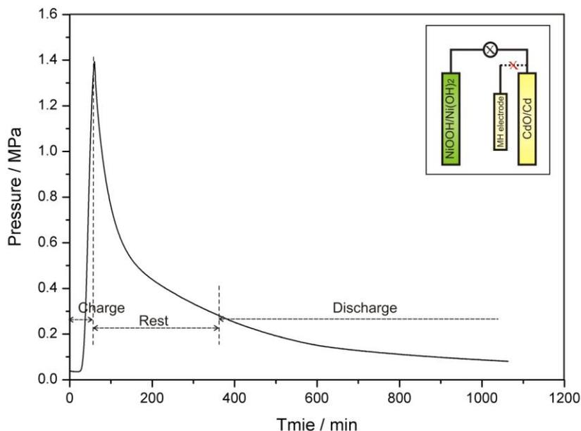
**Figure 4.** The profile of changes of internal pressure over time when the sealed Ni-Cd cell with a isolated alloy electrode was charged at of 2C for 60 minutes, then rested for 300 minutes and discharged at 0.5C down to 1.0 V. Inset: Schematic electrode connection in the modified conventional Ni-Cd cell.
