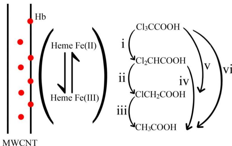
**Figure 7.** Illustrative diagram of TCA dechlorination on the surface of Hb-MWCNT-GE.
