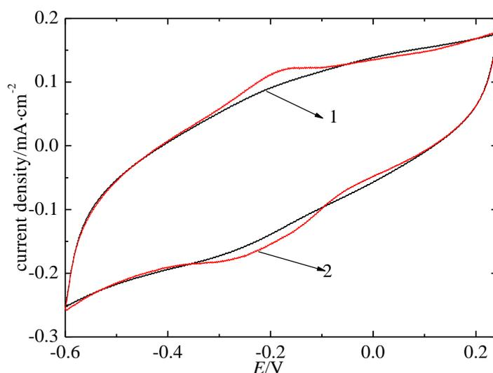
**Figure 1.** Cyclic voltammograms of the MWCNT-GE (curve 1), and Hb-MWCNT-GE (curve 2) in 0.1 M pH 7.0 PBS at a scan rate of  $300 \text{ mV} \cdot \text{s}^{-1}$ .
