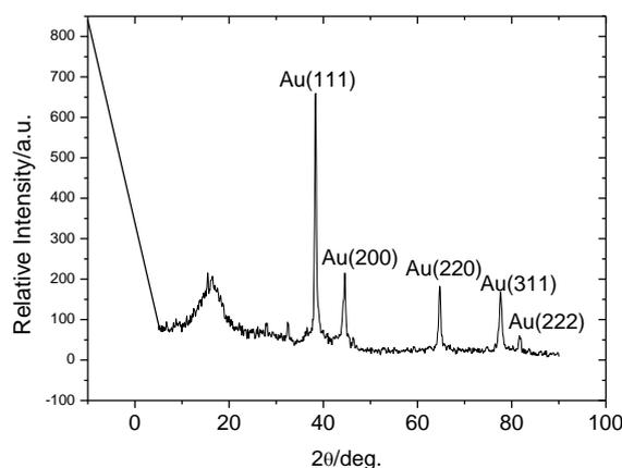
**Figure 2.** XRD pattern of GNPs obtained from aqueous solution
