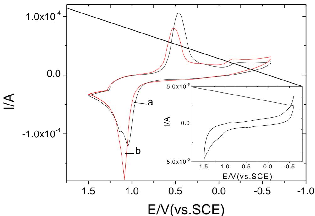
**Figure 4.** CVs of cefoperazone@GNPs (a) and the rinsed GNPs (b). Supporting electrolyte: 0.1 mol.L<sup>-1</sup> PBS of pH 7.3. Insert Figure: CV of 0.4 mg/mL cefoperazone sodium at GCE, supporting electrolyte: 0.5 mol.L<sup>-1</sup> H<sub>2</sub>SO<sub>4</sub>.
