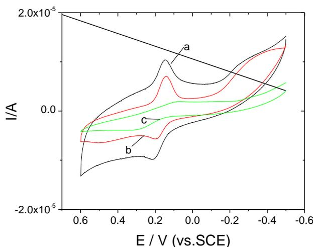
**Figure 6.** CVs of 10.0 mg.L<sup>-1</sup> dopamine at cefoperazone@GNP/GCE (a), the rinsed GNP/GCE (b) and bare GCE (c). Scan rate: 100.0 mV.s<sup>-1</sup>. Supporting electrolyte: 0.1 mol.L<sup>-1</sup> PBS of pH 7.3.
