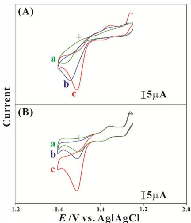
**Figure 3.** (A) shows PEDOT/pt (a), laccase/pt (b) and PEDOT-laccase/pt (c) modified electrode in 0.1 M PBS (pH 7.0 containing 1 mM ABTS) saturated with oxygen. (B) shows the voltammograms recorded at a PEDOT-laccase/pt modified electrode in 0.1 M PBS (pH 7.0 containing 1 mM ABTS) saturated with nitrogen (curve a), ambient air (curve b) and oxygen (curve c). The corresponding cyclic voltammograms have been obtained at  $100 \text{ mVs}^{-1}$  scan rate in the potential range of 1.0 to -0.4 V.
