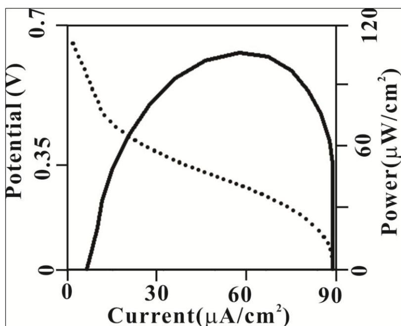
**Figure 7.** Polarization curve (dashed line) and dependence of the power density on the operating voltage (solid line) for a biofuel cell consisting of GOx/MWCNTs modified electrode as anode in combination with a PEDOT-laccase/pt electrode as cathode. As fuel a 5 mM solution of glucose in PBS (pH 7.0) containing 1 mM ABTS was used.
