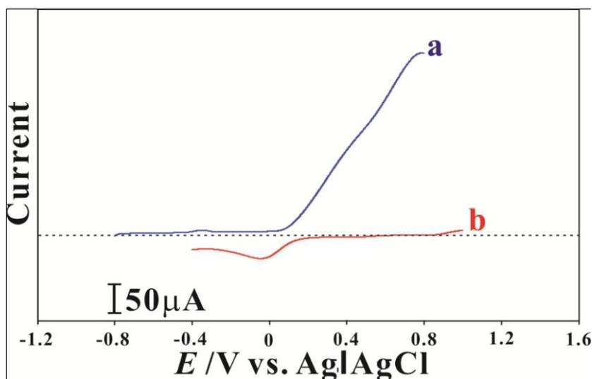
**Figure 6.** Polarization curves obtained in pH 7.0 PBS for the bioanode GOx/MWCNTs modified GC electrode in a 5 mM glucose solution (curve a) and for the biocathode PEDOT-laccase/pt modified electrode in air-saturated solution (curve b).
