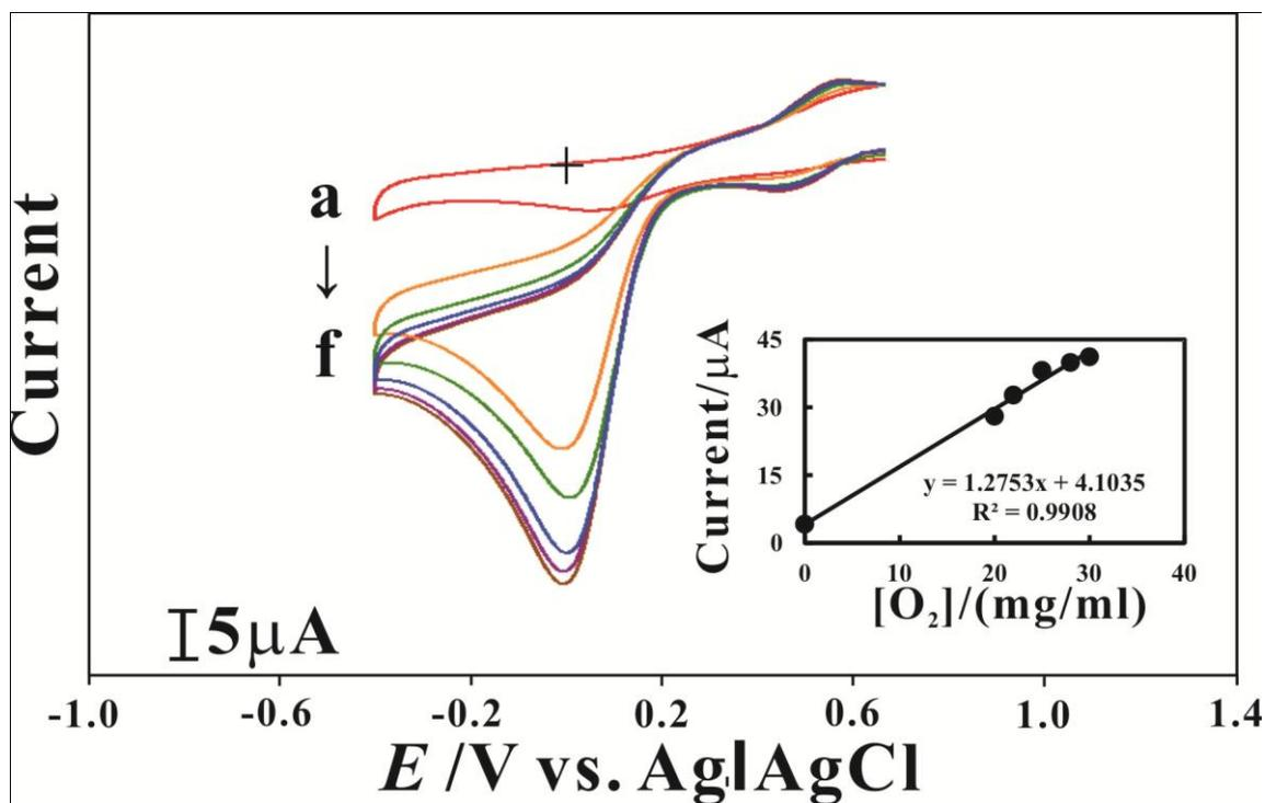
**Figure 4.** CVs of PEDOT-laccase/pt modified electrode was transferred to pH 7.0 PBS (containing 1 mM ABTS) for the electrocatalysis of oxygen. (a) to (f) upon addition of oxygen. Inset shows a current vs. concentration plot of oxygen at PEDOT-laccase/pt modified electrode.
