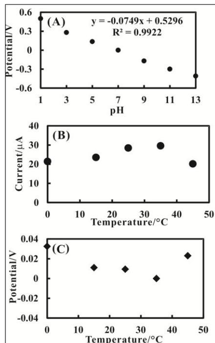
**Figure 5.** Optimization of PEDOT-laccase/pt modified electrodes in (A) shows the stability plot of PEDOT-laccase/pt modified electrodes in different pH 1.0 to 13 solution. (B) shows PEDOT-laccase/pt modified electrode in pH 7.0 PBS (containing 1 mM ABTS) and saturation oxygen conditions at various temperature from 0 to  $45^{\circ}\text{C}$ . (C) shows various temperature vs. reduction potential.
