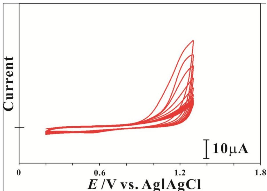
**Figure 1.** Pt electrode was immersed in pH 1.5  $\text{H}_2\text{SO}_4$  solution containing 0.1 mM EDOT and 1 mg/ml laccase from 0.2 V to 1.3 V, scan rate  $100 \text{ mVs}^{-1}$ .
