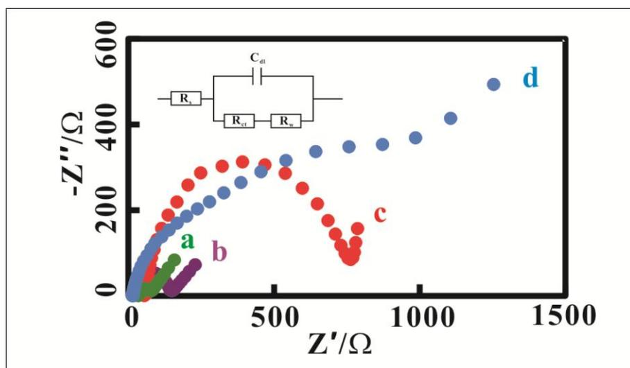
**Figure 2.** Electrochemical impedance spectroscopy (EIS) for (a) PEDOT/pt, (b) Pt, (c) PEDOT-laccase/pt and (d) laccase/pt modified electrodes in the presence pH 7.0 PBS of equimolar 5 mM  $[\text{Fe}(\text{CN})_6]^{3-/4-}$ . The insert displayed the equivalent circuit (Randles model) was used to fit Nyquist diagrams.
