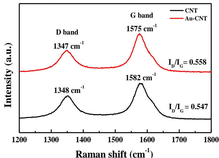
**Figure 3.** Raman spectrum of the CNTs and Au-coated measured at room temperature.
