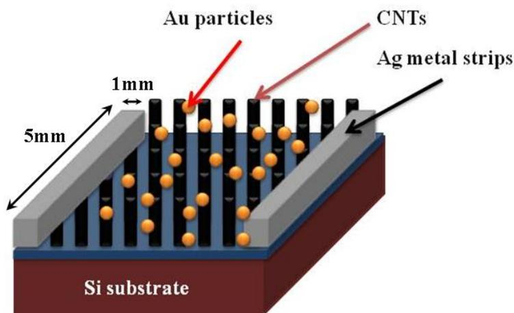
**Figure 1.** Schematic diagram of the fabricated carbon nanotubes gas sensing device.
