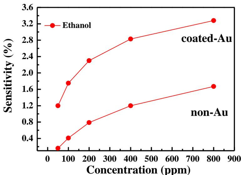
Figure 5. Sensitivities of the CNTs sensors without and with Au adsorption measured at various ethanol concentrations.
