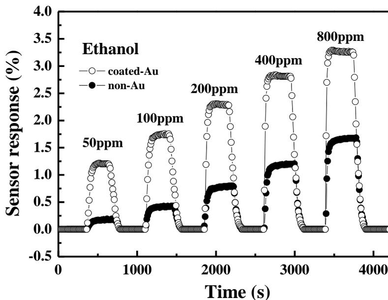
Figure 4. CNT gas sensors measured at various ethanol concentrations.
