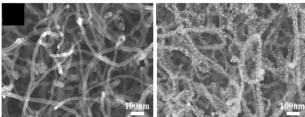
**Figure 2.** (a) Top-view FESEM image of the CNTs grown onto SiO<sub>2</sub> Si substrate (b) with Au adsorption.
