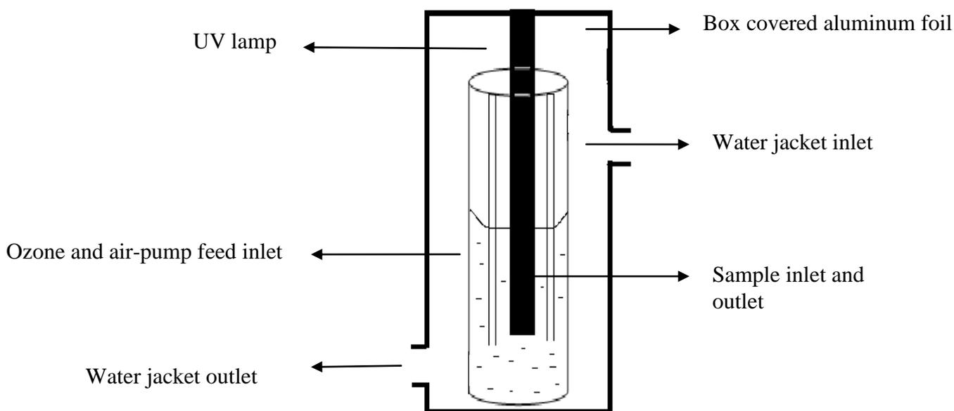
**Figure 1.** Experimental set up for all systems studied.
