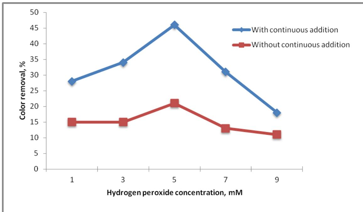
**Figure 2.** Removal of 20 ppm MO by UV/Fe(III)/H<sub>2</sub>O<sub>2</sub> system, with Fe(III) = 2ppm and various H<sub>2</sub>O<sub>2</sub> concentration at initial pH ≈ 6
