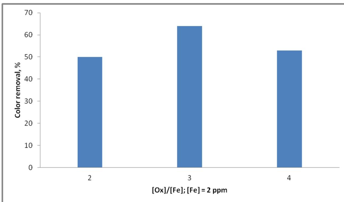
**Figure 5.** Determination of  $[\text{Ox}]/[\text{Fe}^{3+}]$  concentration ratio, ( $[\text{Fe}^{3+}] = 2 \text{ ppm}$ ) for decolorization of 20 ppm MO at  $\text{pH} \approx 6$
