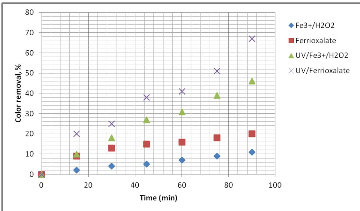
**Figure 4.** MO removal with different homogeneous systems studied; MO = 20 ppm, Fe(III) = 2 ppm, Oxalate (Ox) = 6 ppm, H<sub>2</sub>O<sub>2</sub> = 5 mM at pH ≈ 6
