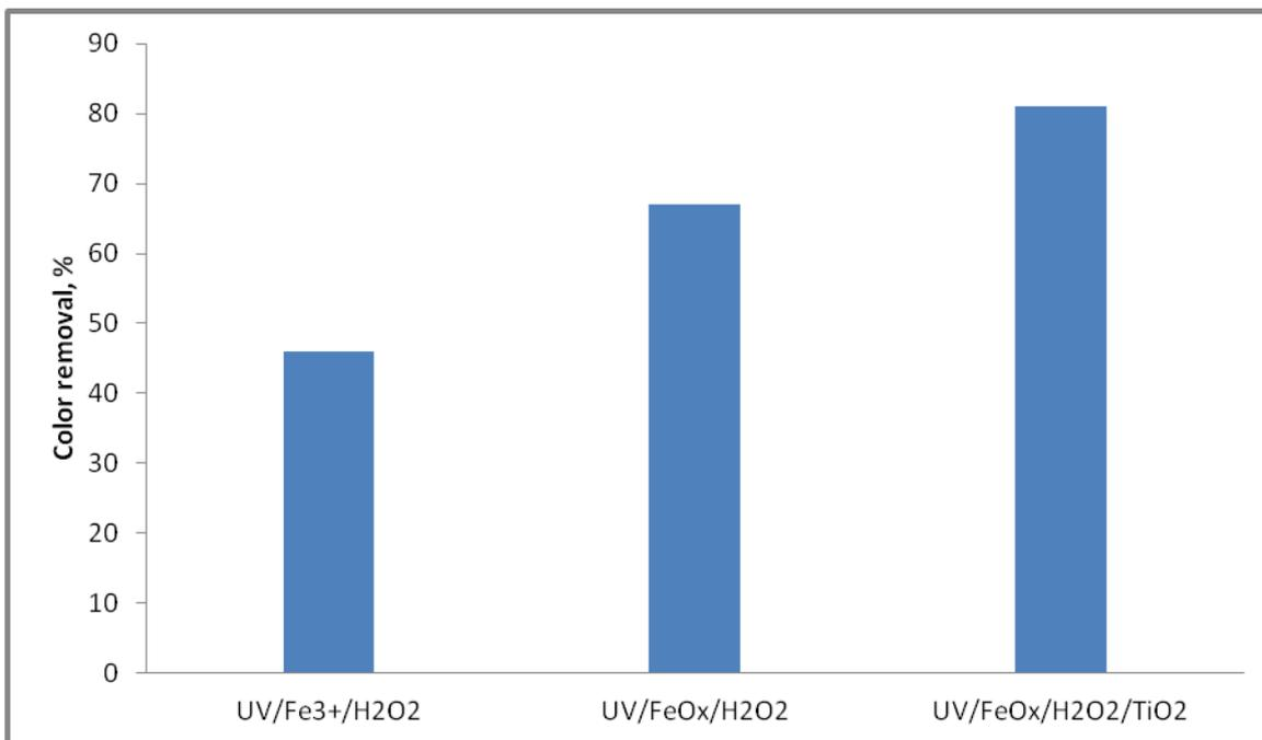
**Figure 6.** Efficiency of photo Fenton, photo Ferrioxalate and photo Ferrioxalate/TiO<sub>2</sub> systems in MO removal, [MO] = 20 ppm, [Fe<sup>3+</sup>] = 2 ppm, [oxalate] = 6 ppm, [H<sub>2</sub>O<sub>2</sub>] = 5mM.
