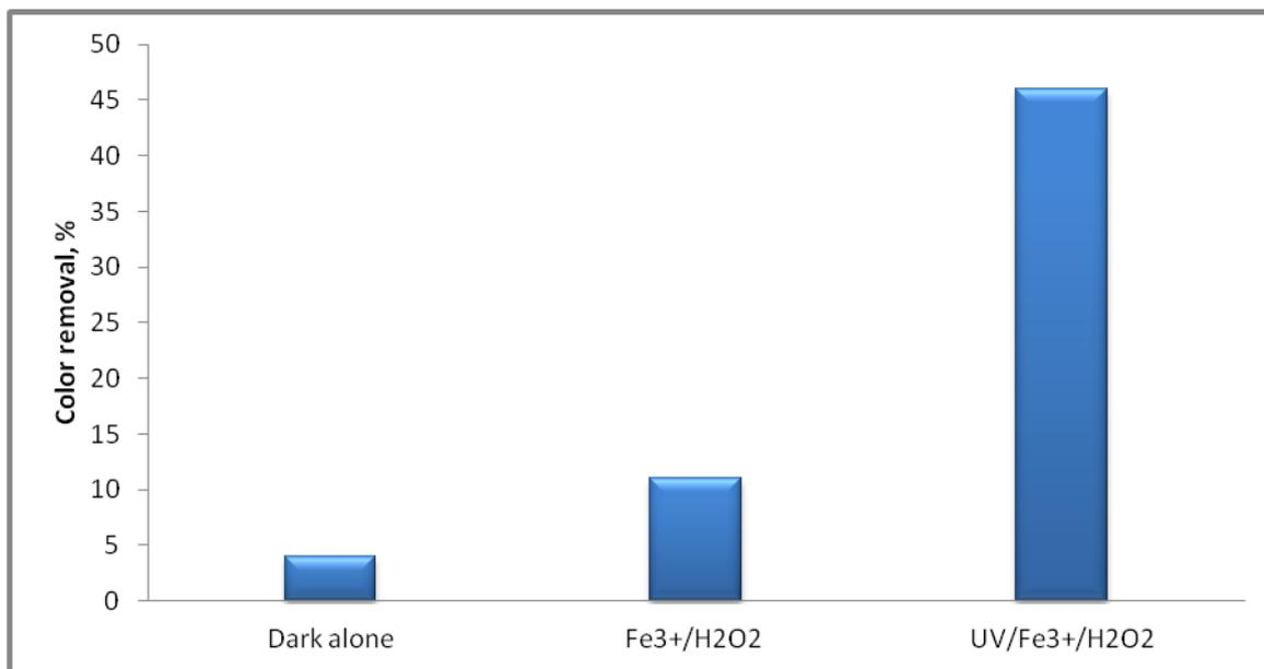
**Figure 3.** The effect of UV and Fenton’s reagent (Fe(III) = 2ppm, H<sub>2</sub>O<sub>2</sub> = 5 mM) for 20 ppm MO removal at pH ≈ 6
