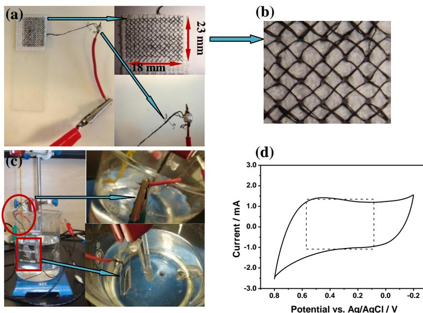
Figure 3. The photographs of weaved CNT fibers on a cloth and the electrochemical test for this weaved CNT fiber cloth. (a) The weaved CNT fiber cloth electrode; (b) The large image of CNT fiber weaved on a cloth; (c) The photographs of three electrodes system of weaved CNT fiber cloth for electrochemical tests; (d) The CV curve of weaved CNT fiber cloth.
