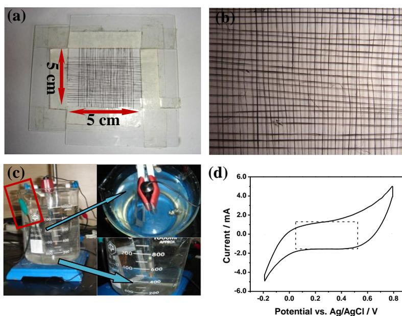
**Figure 4.** The photographs of a pure-weaved CNT fabric and the electrochemical test for this CNT fabric. (a) The pure-weaved CNT fabric; (b) The large image of self-weaved CNT fabric; (c) The photographs of three electrodes system of self-weaved CNT fabric for electrochemical tests; (d) the CV curve of self-weaved CNT fabric.
