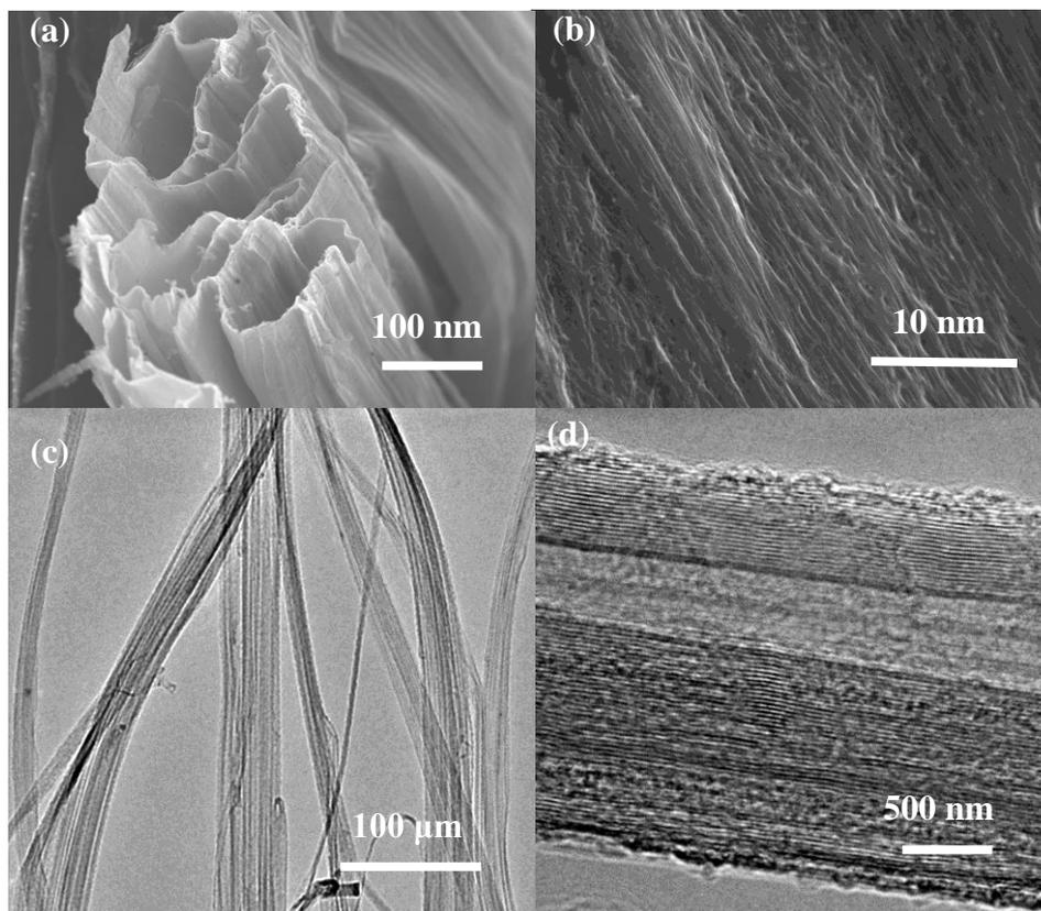
**Figure 5.** Microstructures of the multilayered CNT fibers observed by SEM (a, b) and TEM (c, d). (a) Cross-sections of a group of as-spun CNT fibers, showing the hollow, multilayer microstructures insert; (b) A CNT yarn surface showing densely packed CNT bundles aligned along the fiber axis; (c) The CNT bundles observed by TEM; (d) High-resolution TEM images of a CNT fiber.
