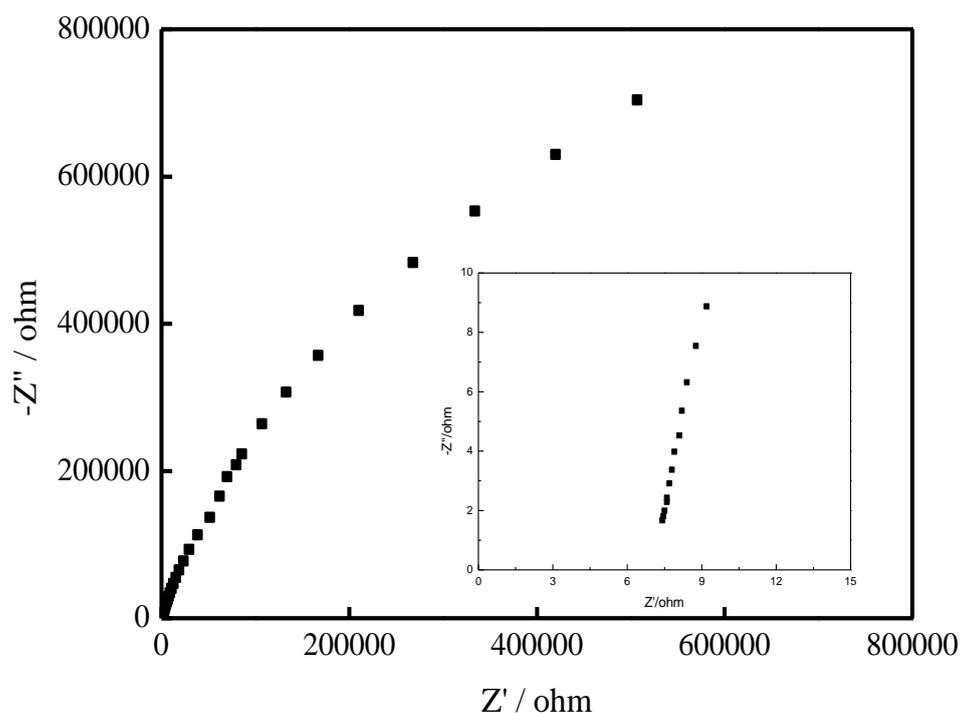
**Figure 3.** Nyquist plot of the blocking cell (SS/composite polymer electrolyte/SS)
