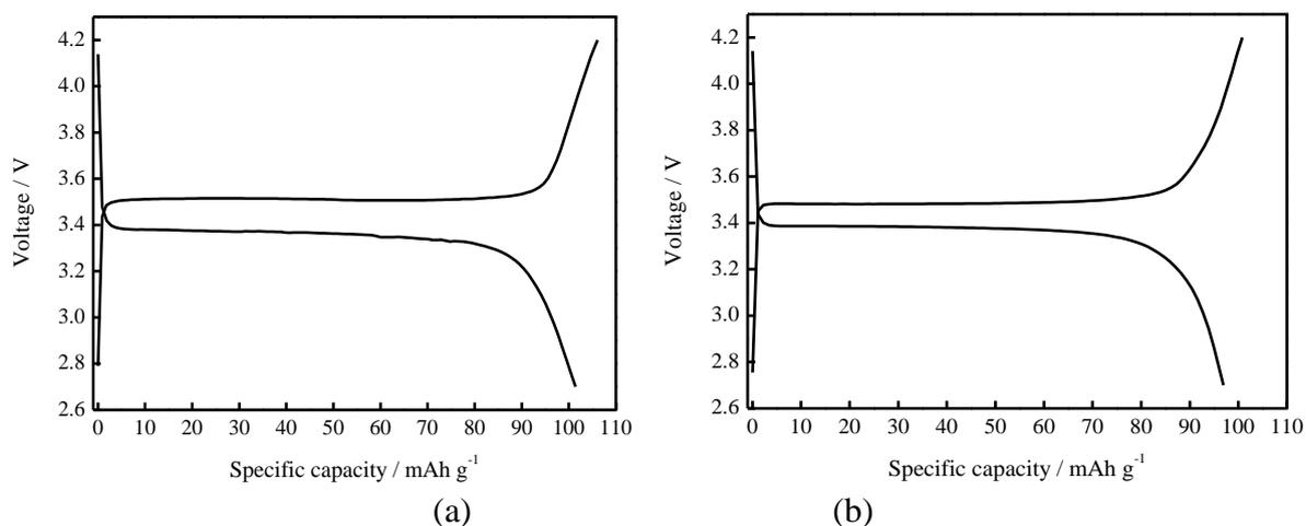
**Figure 5.** Initial voltage profile of the Li/LiFePO<sub>4</sub> cell. (a) PP/PE/PP film in 1 mol L<sup>-1</sup> LiPF<sub>6</sub> (DMC:DEC:EC=1:1:1, w/w/w) used as the electrolyte, (b) composite polymer electrolyte used as the electrolyte
