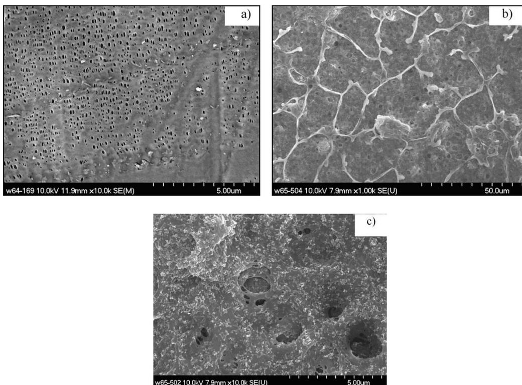
**Figure 1.** SEM images of (a) PP/PE/PP film, (b) dried composite polymer film (low magnification) and (c) dried composite polymer film (high magnification)
