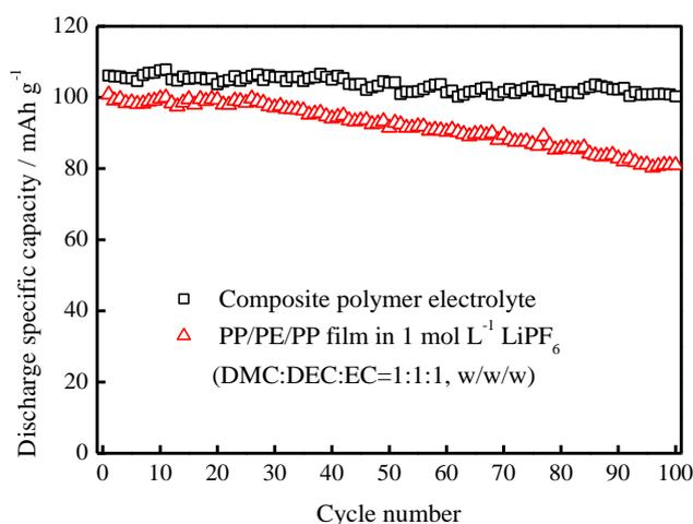
**Figure 6.** Cycle performance of the Li/LiFePO<sub>4</sub> cell. (a) PP/PE/PP film in  $1 \text{ mol L}^{-1} \text{ LiPF}_6$  (DMC:DEC:EC=1:1:1, w/w/w) used as the electrolyte, (b) composite polymer electrolyte used as the electrolyte
