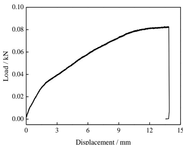
**Figure 2.** Mechanical strength test of the dried composite polymer film
