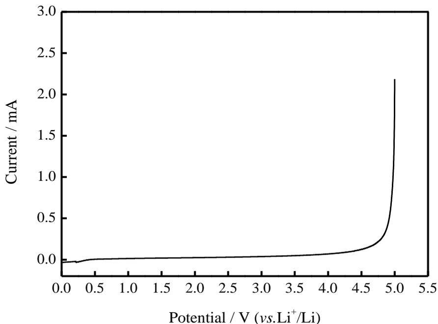
**Figure 4.** LVS diagrams of the composite polymer electrolyte
