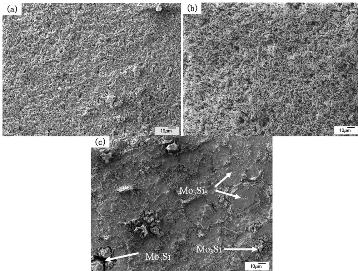
**Figure 6.** Surface morphologies of the Mo<sub>5</sub>Si<sub>3</sub> alloy after anodic potentiodynamic polarization in 1 mol/L HCl(a), 1 mol/L H<sub>2</sub>SO<sub>4</sub>(b) and 1 mol/L NaOH(c).
