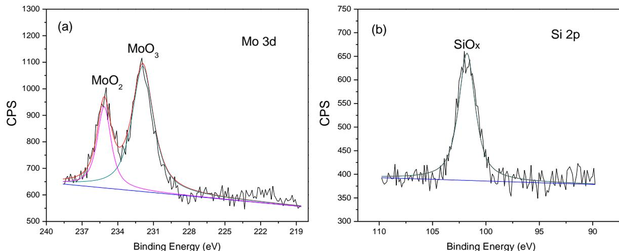
**Figure 5.** High-resolution XPS spectra of Mo<sub>5</sub>Si<sub>3</sub>-based alloy after 10 min potentiostatic polarization at 0.1 V vs. SCE in 1 mol/L HCl solution: (a) Mo 3d, (b) Si 2p
