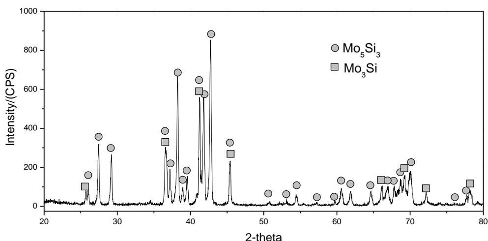
**Figure 1.** X-ray diffraction pattern of the  $\text{Mo}_5\text{Si}_3$  alloy
