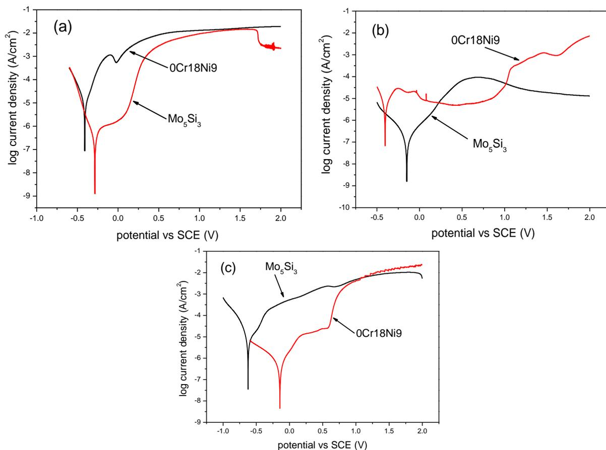
**Figure 3.** Anodic potentiodynamic polarization curves of the  $\text{Mo}_5\text{Si}_3$  alloy in comparison to the stainless steel 0Cr18Ni9 in 1 mol/L HCl (a), 1 mol/L  $\text{H}_2\text{SO}_4$  (b) and 1 mol/L NaOH (c) solutions
