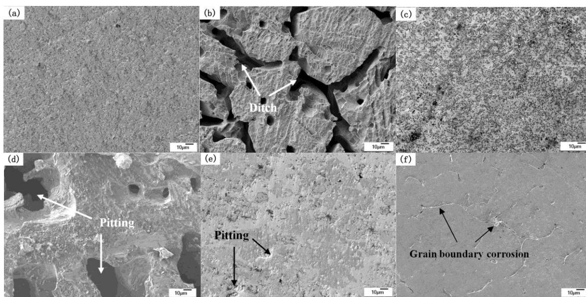
**Figure 7.** SEM images showing the surface morphologies of the  $\text{Mo}_5\text{Si}_3$ -based alloy(a),(c),(e) and austenitic stainless steel(b),(d),(f) after immersion for 100h in 1 mol/L HCl(a),(b), 1 mol/L  $\text{H}_2\text{SO}_4$ (c),(d), and 1 mol/L NaOH solutions(e),(f)
