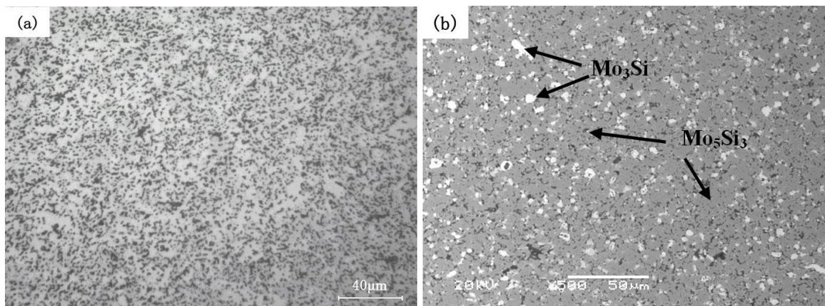
**Figure 2.** OM (a) and SEM (b) micrographs showing microstructure of the  $\text{Mo}_5\text{Si}_3$  metal silicide alloy
