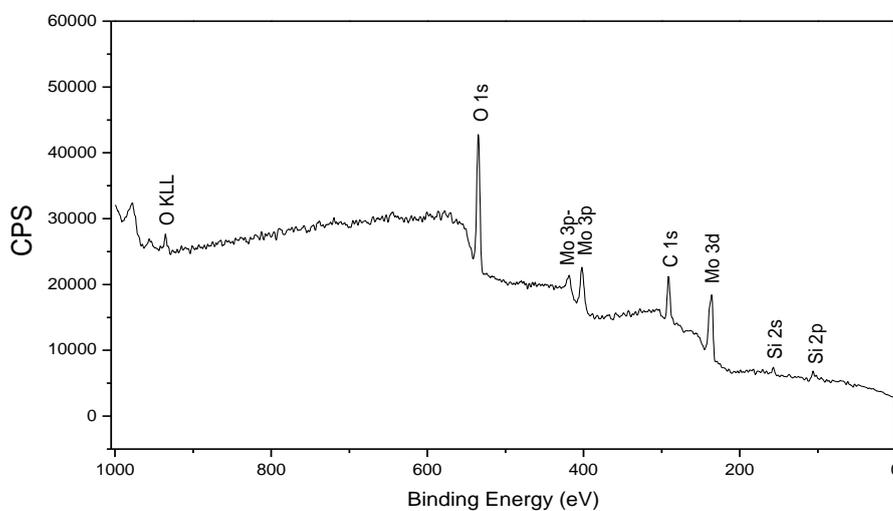
**Figure 4.** XPS survey spectra of the  $\text{Mo}_5\text{Si}_3$ -based alloy after passivation at 0.1 V vs. SCE for 10 min in 1 mol/L HCl solution
