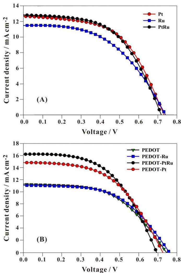
**Figure 4.** Photocurrent density-voltage curves of DSSCs based on CEs of Pt, Ru and PtRu NPs on (A) ITO and (B) PEDOT/ITO, respectively. The measurements were recorded under  $100 \text{ mW cm}^{-2}$ , AM 1.5.
