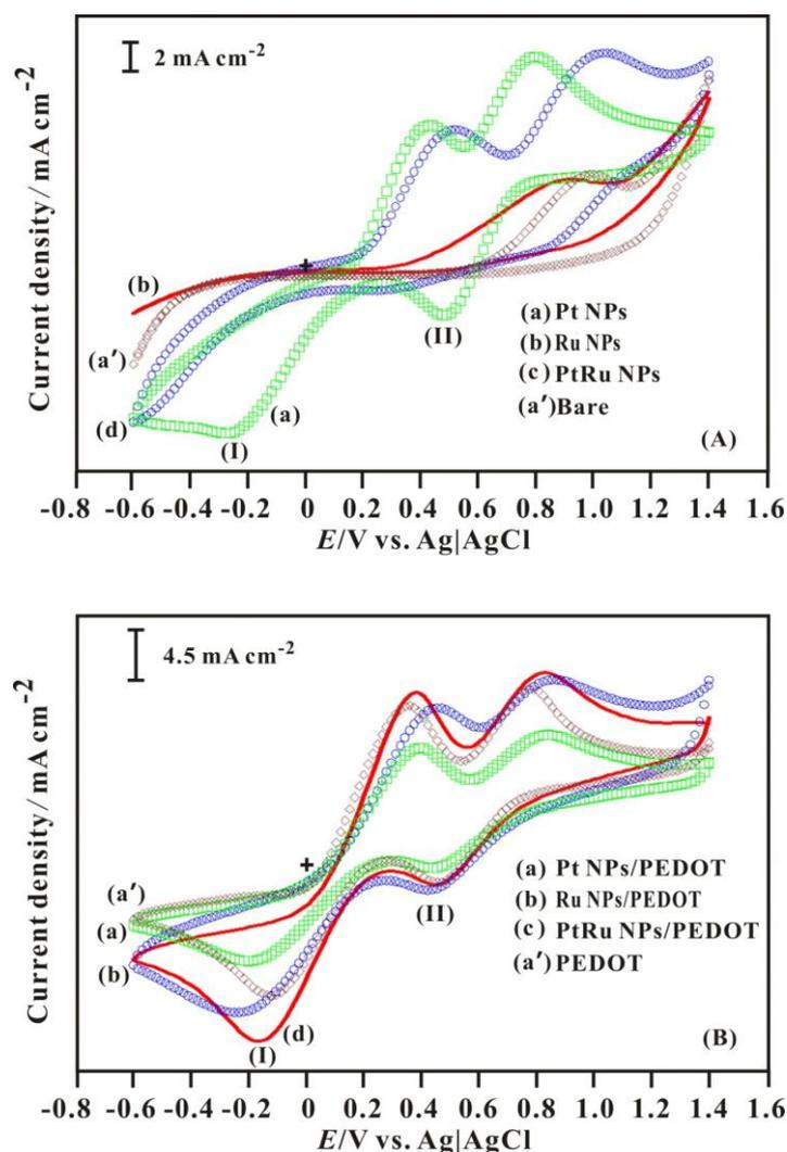
**Figure 3.** Cyclic voltammograms of (A) (a') ITO, (a) Pt, (b) Ru and (c) PtRu NPs electrodeposited on ITO electrode and (B) (a'), (a) Pt, (b) Ru and (c) PtRu NPs electrodeposited on PEDOT/ITO electrode in an acetonitrile solution with 0.01 M LiI, 0.001 M I<sub>2</sub> and 0.1 M LiClO<sub>4</sub>, initial E = + 1.6 V, high E = + 1.6 V, low E = -0.4 V, scan rate = 50 mV s<sup>-1</sup>.
