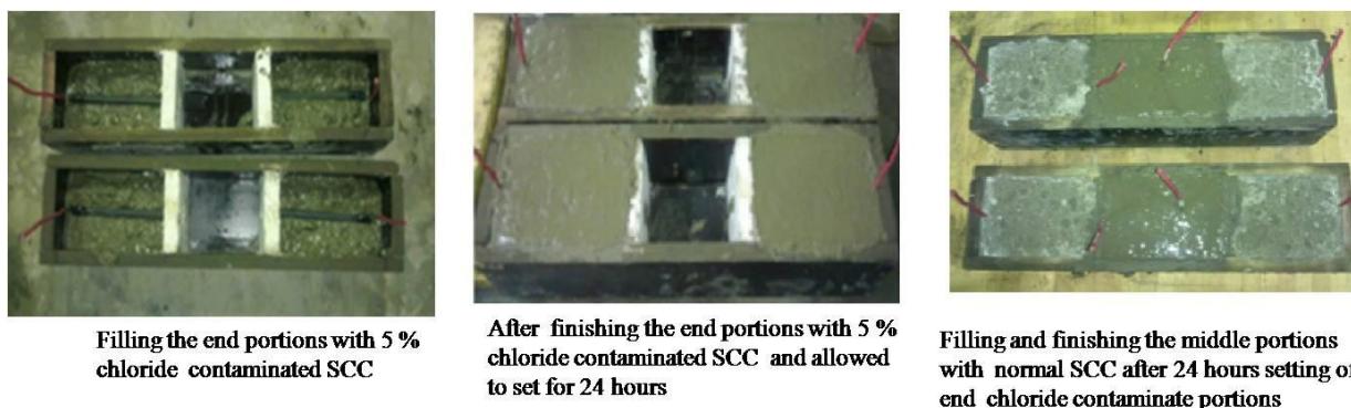
Figure 3. SCC macro-cell specimen preparation.
