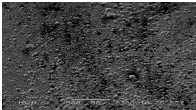
Figure 7. SEM of Ni 82 -P 18 alloy from bath "A "operated at working conditions pH9, 90 °C and duration time 60 min.
