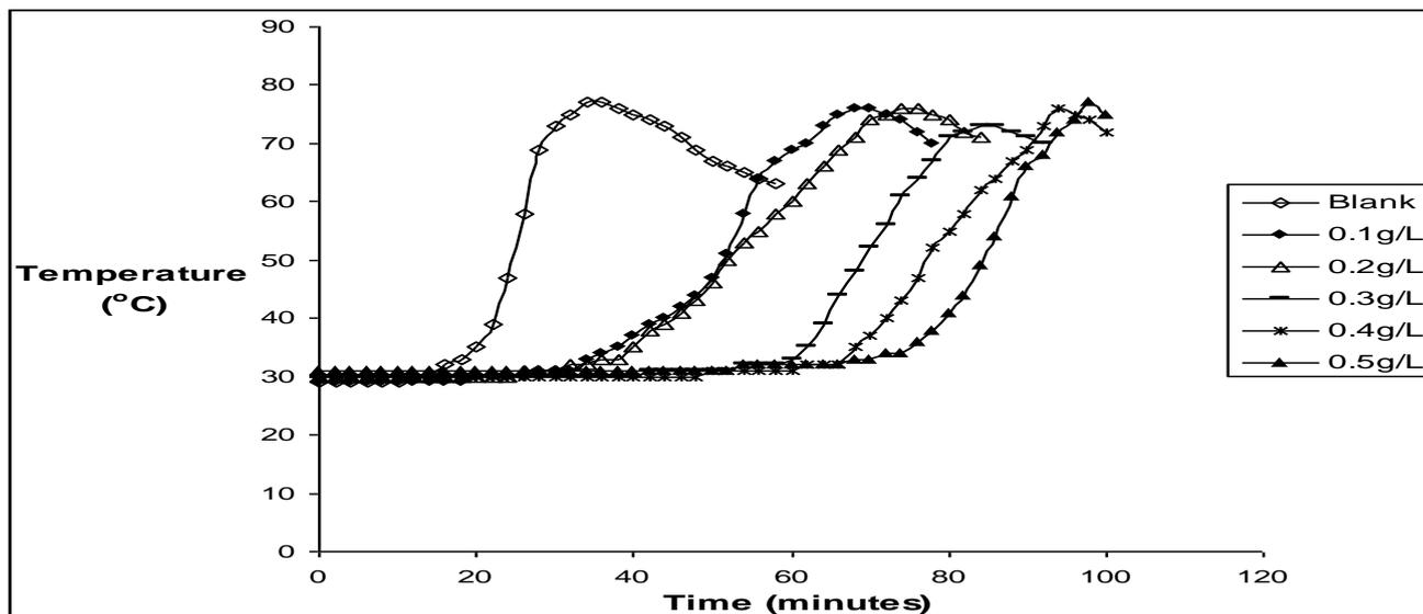
**Figure 7.** Variation of temperature with time for aluminium dissolution in 2.0 M HCl in the absence and presence of ROST.
