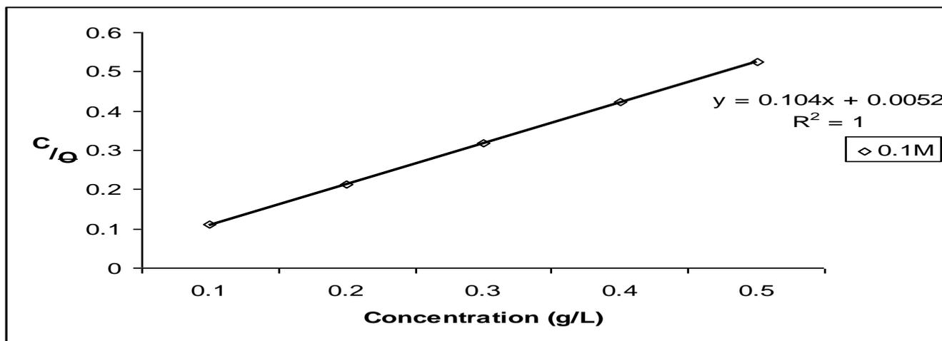
**Figure 14.** Langmuir plots for adsorption data in studied HCl solutions
