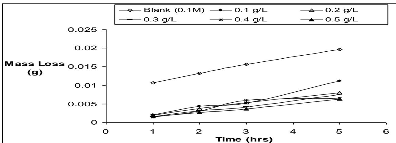
Figure 10. Variation of ROST mass loss with time in 0.1M hydrochloric acid at 50°C.
