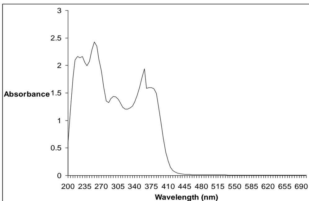
**Figure 2.** UV/visible spectrum of ROST in ethanol
