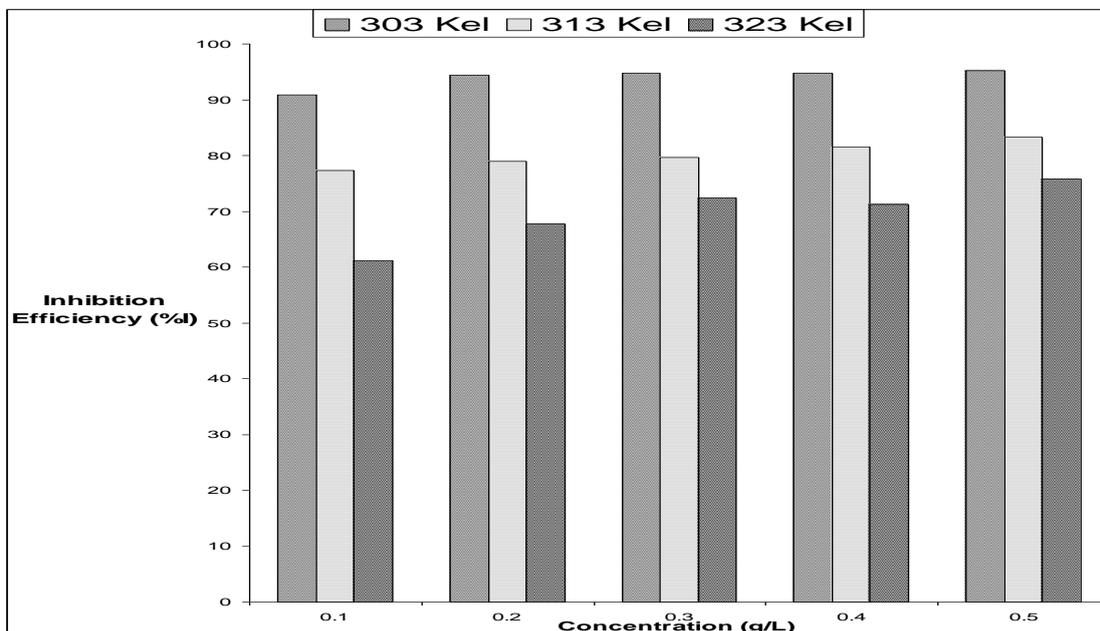
**Figure 4.** Effect of temperature on inhibition efficiency for various ROST concentrations in 0.1M hydrochloric acid.
