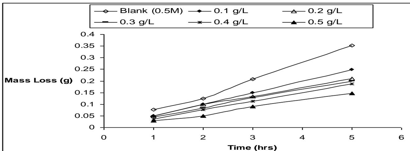
Figure 13. Variation of ROST mass loss with time in 0.5M hydrochloric acid at 50°C.
