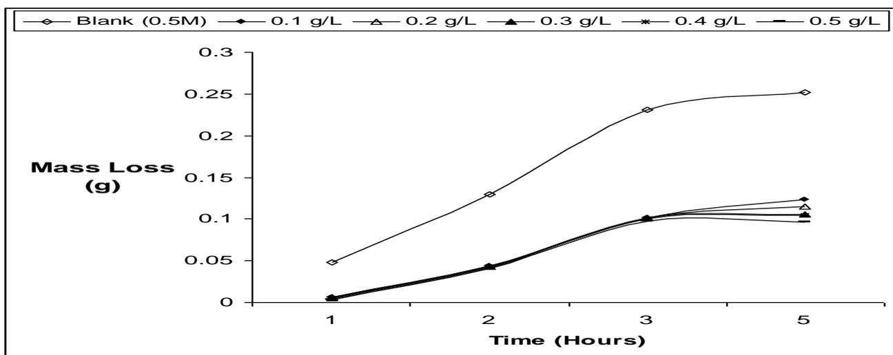
Figure 11. Variation of ROST mass loss with time in 0.5M hydrochloric acid at 30°C.
