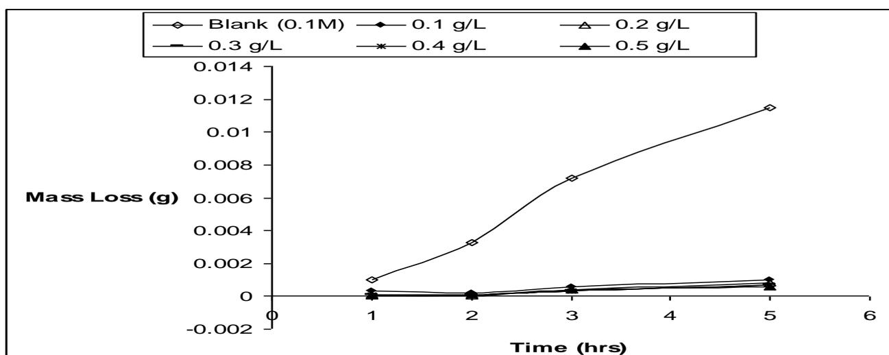
**Figure 8.** Variation of ROST mass loss with time in 0.1M hydrochloric acid at 30°C.
