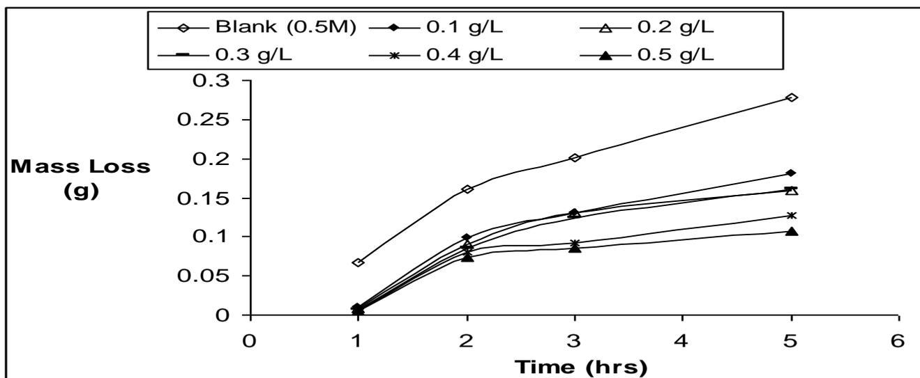
Figure 12. Variation of ROST mass loss with time in 0.5M hydrochloric acid at 40°C.
