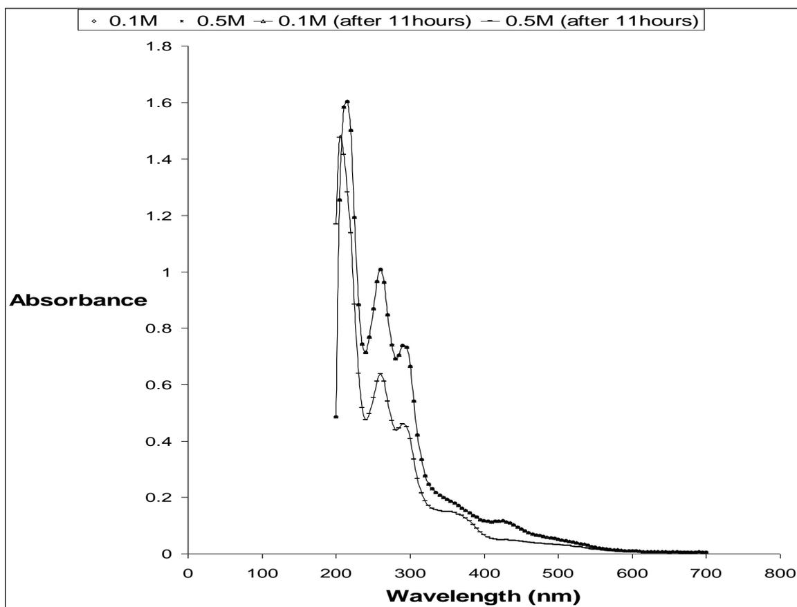
**Figure 6.** UV/visible spectra of ROST in 0.1M and 0.5M HCl solutions after 11 hours.
