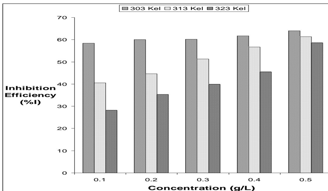
**Figure 5.** Effect of temperature on inhibition efficiency for various ROST concentrations in 0.5M hydrochloric acid.
