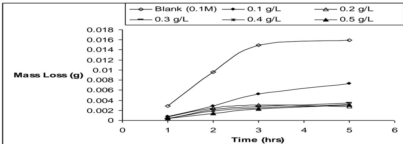
Figure 9. Variation of ROST mass loss with time in 0.1M hydrochloric acid at 40°C.
