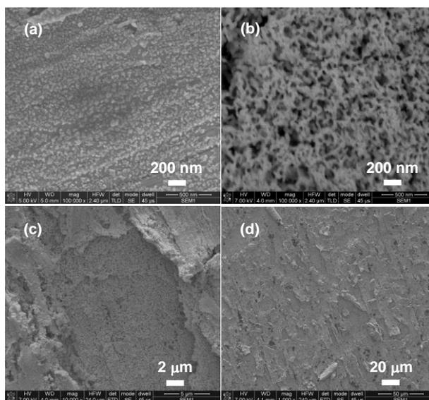
**Figure 4.** SEM images of NPGFs prepared by anodization of gold at 8 V for (a) 10 s and (b–d) 1000 s in 0.1 M OA.
