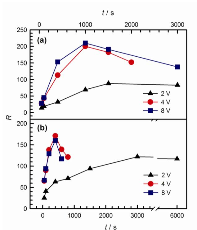
**Figure 3.** The dependence of roughness factor ( $R$ ) on step time at different anodic potentials on the smooth Au electrode in an aqueous solution of (a) 0.1 M and (b) 0.5 M OA.
