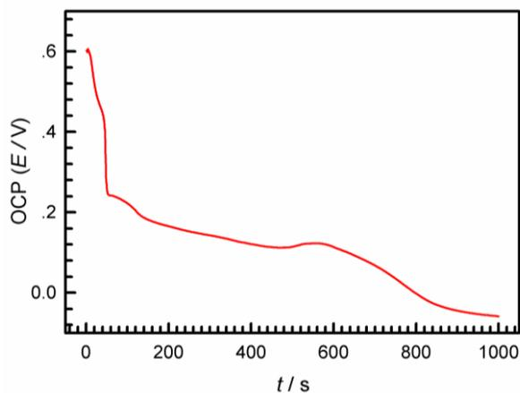
**Figure 2.** Open circuit potential (OCP)–time curve for the thick film of gold oxide in 0.1 M OA solution. The oxide film used here is prepared ex situ by oxidizing the smooth gold electrode at 4 V for 100 s in 0.5 M  $H_2SO_4$  solution.
