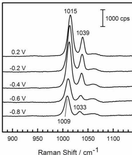
**Figure 6.** SERS spectra of pyridine (Py) on the NPGF electrode in a solution of 0.01 M Py + 0.1 M KCl. The NPGF was prepared under the same condition as shown in Fig. 5.
