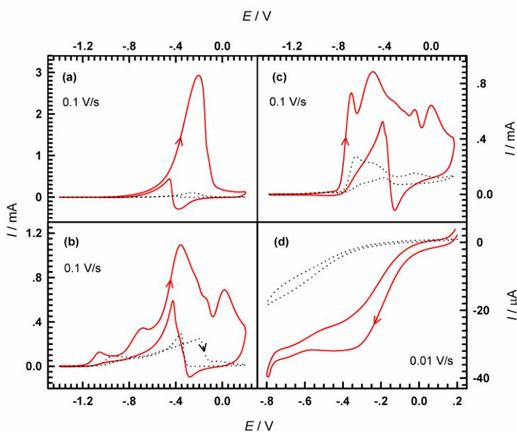
**Figure 5.** CVs on smooth Au (the dotted lines) and NPGF (the solid lines) electrodes in (a) 1 M NaOH + 1 M ethanol, (b) 1 M NaOH + 1 M glucose, (c) 1 M NaOH + 0.1 M ascorbic acid, and (d) 0.5 M  $\text{H}_2\text{SO}_4$  + 0.1 M  $\text{H}_2\text{O}_2$ . The NPGF electrodes were prepared by anodic oxidation at 8 V for 1000 s.
