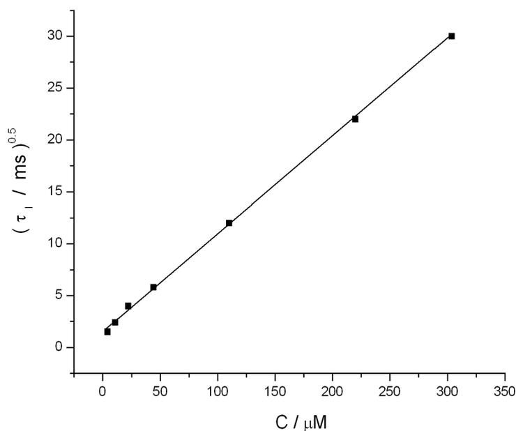
**Figure 3.** The dependence of the square root of the first transition time ( $\tau_1^{0.5}$ ) on the TNT concentration in the range of 4.4 – 304  $\mu\text{M}$ ; the coefficient of determination,  $R^2$ , is 0.9995.
