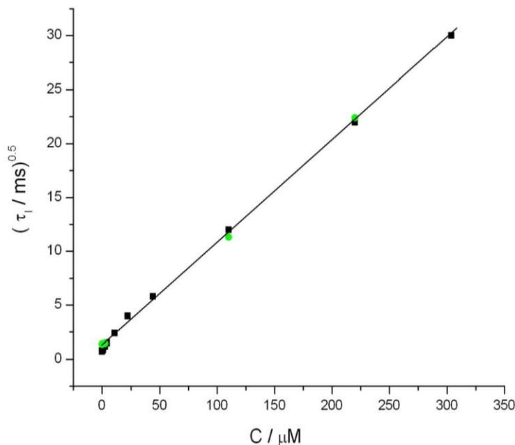
**Figure 7.** The calibration plot as dependence of the square root of the first transition time ( $\tau_1^{0.5}$ ) on the TNT concentration in the range of  $0.09 - 308\mu\text{M}$ , with experimental points obtained in the river water ( $\bullet$ ); the coefficient of determination for the experimental points obtained in the river water,  $R^2$ , is 0.9992.
