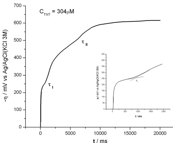
**Figure 1.** The E-t response on the constant current pulse (0.1mA) obtained in the basic electrolyte (0.5 M NaCl with acetonitrile) containing 304 $\mu$ M of TNT. Inset of the Fig.1 shows the way of the transition time determination.
