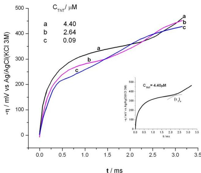
**Figure 4.** The E-t responses on the constant current pulse (0.1mA) obtained in the basic electrolyte (0.5M NaCl with acetonitrile) containing 0.09 – 4.40 μM of TNT. Inset shows the way of the transition time determination.
