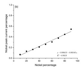
**Figure 3.** Dependence of copper and nickel oxidation peak current percentages on the composition of the copper-nickel alloy (total amount of the sample is 40 mg).
