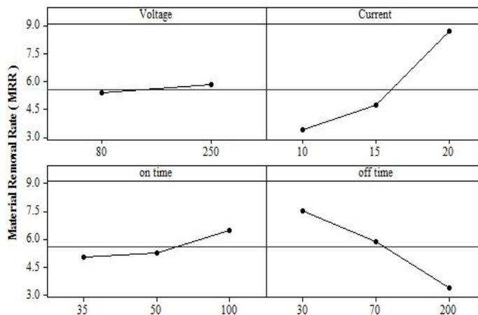
Figure 2. Impact of input parameters of the process on material removal rate of NiTi SMA
