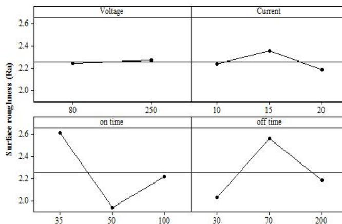
Figure 5. Impact of input parameters of the process on surface roughness
