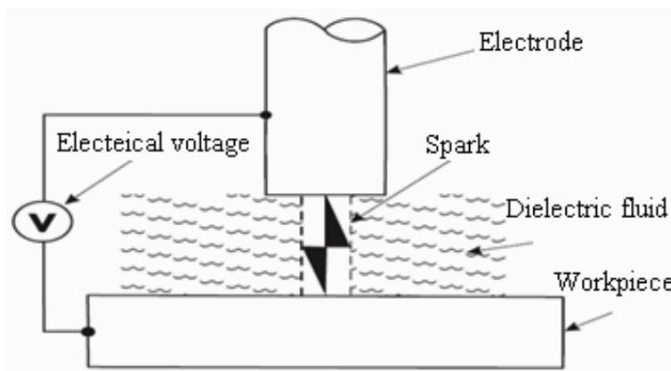
**Figure 1.** Basic components of EDM [13]
