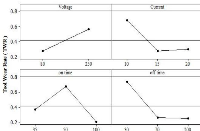
Figure 3. Impact of input parameters of the process on tool wear rate of copper tools
