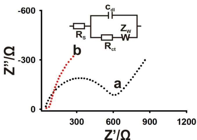
**Figure 4.** EIS of bare GCE (a) and ERGO/GCE (b) modified electrodes in 5 mM  $\text{Fe}(\text{CN})_6^{3-/4-}$  containing 0.1 M KCl. Inset is the Randles equivalent circuit.  $R_s$ ,  $C_{dl}$ ,  $R_{ct}$  and  $Z_w$  represent the resistance of the electrolyte solution, double layer capacitance, charge-transfer resistance and the Warburg impedance, respectively. The frequency range is from 0.1 Hz to 100 kHz.
