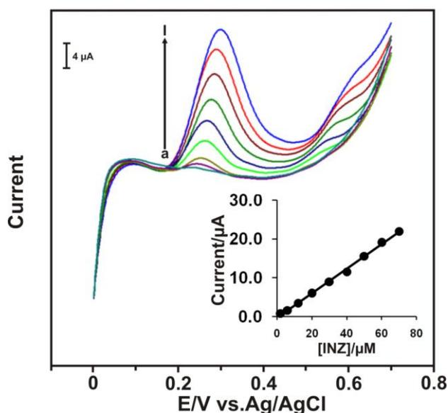
**Figure 8.** LSV of ERGO modified GCE in different concentration of INZ (a-i) in PBS at the scan rate of  $100 \text{ mV s}^{-1}$ . Inset plot shows the linear dependence of  $I_{\text{pa}}$  vs.  $[\text{INZ}]$
