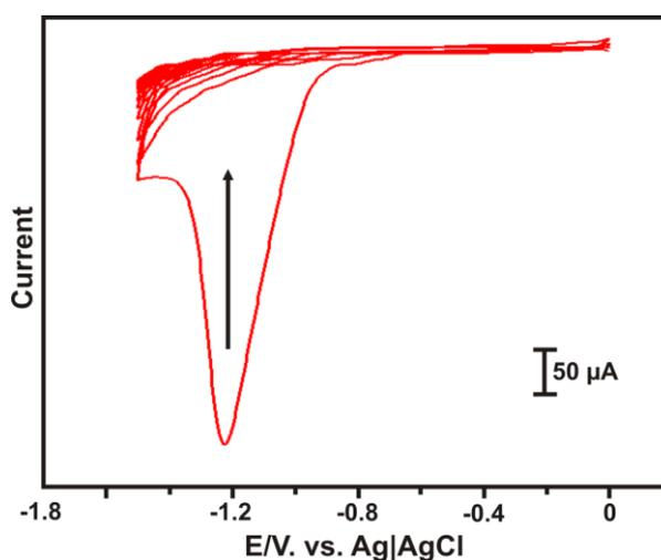
**Figure 2.** 30 successive cyclic voltammograms were performed in GO modified GCE at 0 to -1.5 V in pH 5 solution at the scan rate  $50 \text{ mVs}^{-1}$ .
