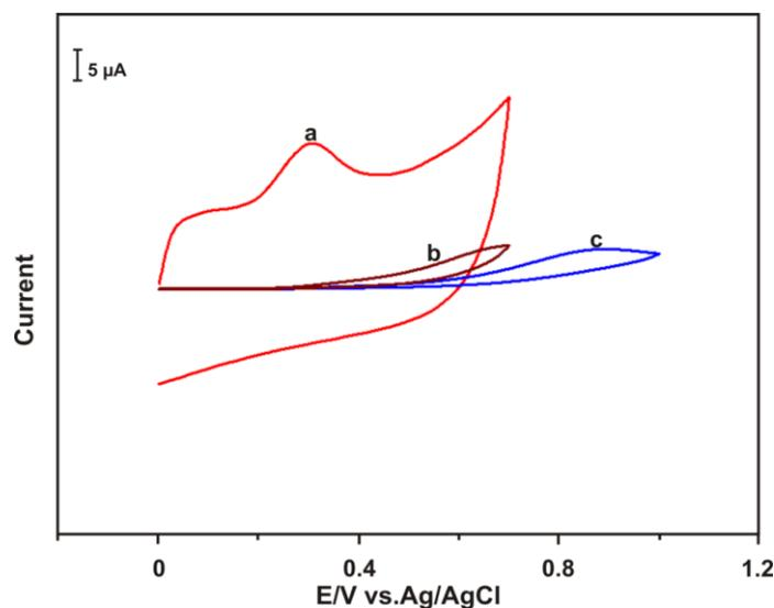
**Figure 5.** Cyclic voltammograms of ERGO/GCE (a),GO/GCE (b), and bare GCE (c) modified electrodes in the presence of 60  $\mu$ M INZ in deoxygenated PBS at 100  $mV s^{-1}$  scan rate.
