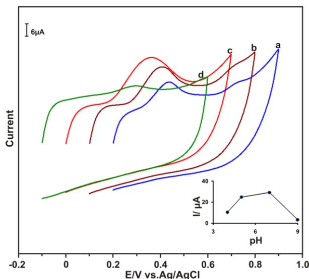
**Figure 7.** Cyclic voltammograms obtained at ERGO/GCE in 60  $\mu\text{M}$  INZ in deoxygenated various pH solutions (4–11) at the scan rate of  $100 \text{ mV s}^{-1}$ .
