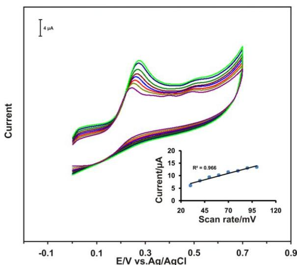
**Figure 6.** Cyclic voltammograms recorded at ERGO/GCE in 60  $\mu\text{M}$  INZ in deoxygenated PBS at different scan rates. The scan rates from inner to outer are: 30 to 100  $\text{mV s}^{-1}$ . Inset shows the linear dependence of  $I_{pa}$  vs scan rate (30 to 100  $\text{mV s}^{-1}$ ).
