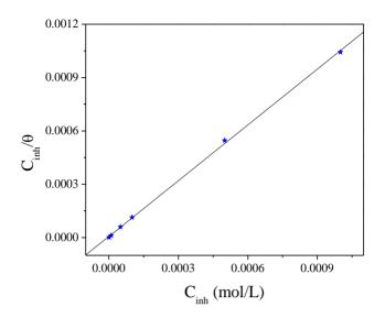
**Figure 8.** Langmuir isotherm adsorption model of N-NEDHME on the surface of C38 steel in 1.0 M HCl.
