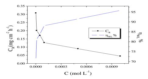
Figure 7. Variation of the corrosion rate and inhibitive efficiency against the N-NEDHME concentrations.
