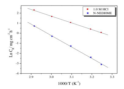
**Figure 8.** Arrhenius plots of Ln C<sub>R</sub> vs. 1/T for steel in 1.0 M HCl in the absence and the presence of N-NEDHME at optimum concentration.
