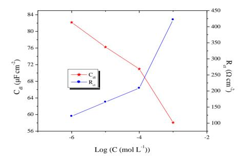
**Figure 6.** Evolution of transfer resistance and capacitance as function of logarithm of N-NEDHME concentration.
