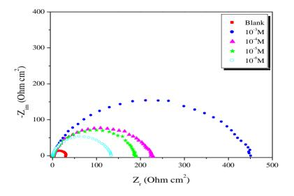
**Figure 3.** Typical Nyquist plots obtained for the C38 steel in 1.0 M HCl in the absence and presence of four different concentrations of N-NEDHME.
