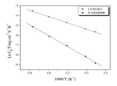
**Figure 9.** Arrhenius plots of Ln C<sub>R</sub>/T vs. 1/T for steel in 1.0 M HCl in the absence and the presence of N-NEDHME at optimum concentration.
