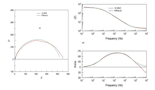
Figure 4. EIS Nyquist (a) and Bode (b) plots for carbon steel/1.0 M HCl +  $10^{-3}$ M N-NEDHME interface: (....) experimental data; (—) calculated.
