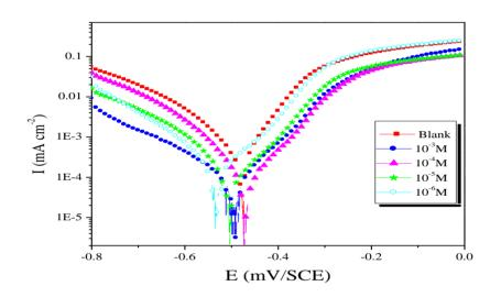
**Figure 2.** Polarization curves for Steel in 1.0 M HCl in the absence and presence of different concentrations of N-NEDHME at 308K.
