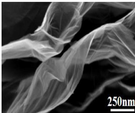
Figure 1. The SEM image of graphene particles
