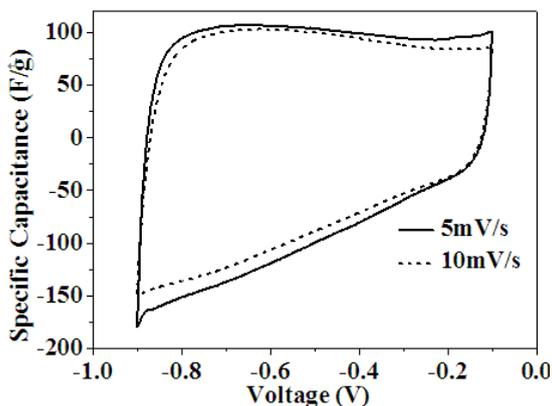
Figure 3. Cyclic voltammograms of the graphene-based supercapacitor
