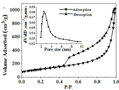
Figure 2. Nitrogen sorption isotherm of graphene at 77K, inset shows the pore size distribution
