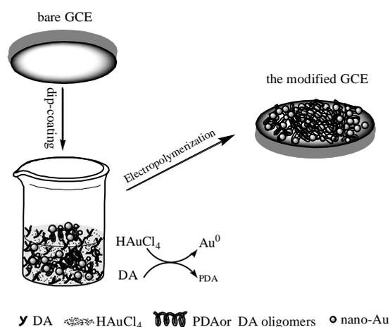
**Scheme 1.** Schematic illustration of the construction of the PDA-nanogold composites modified electrode
