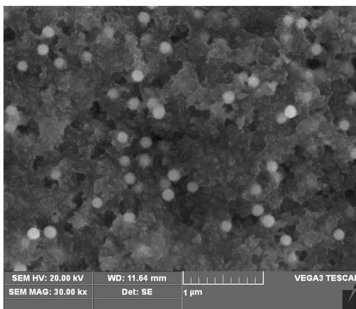
**Figure 1.** SEM micrograph of the PDA-nanogold composites film
