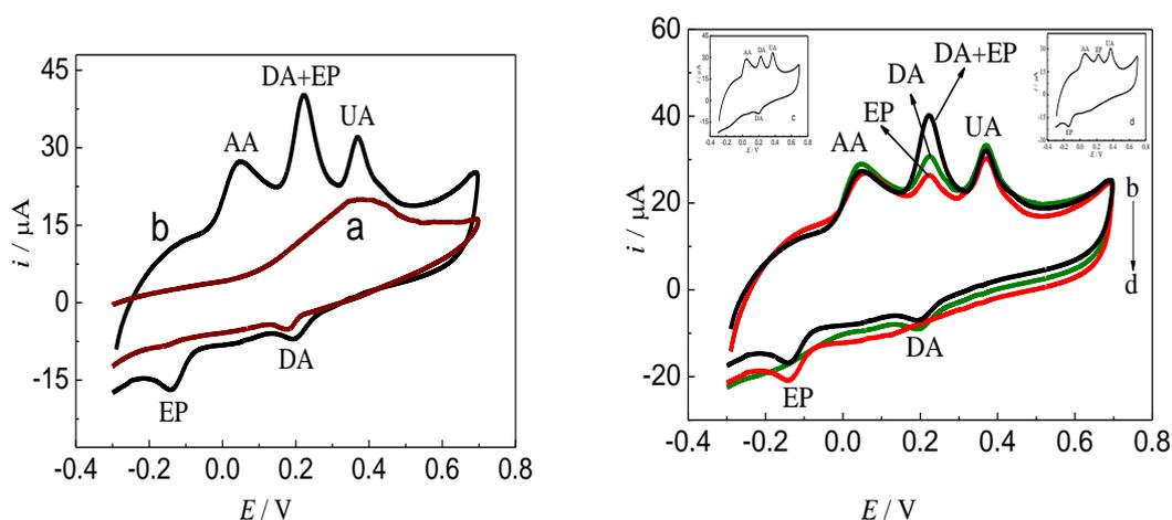
**Figure 3.** CVs of a mixture containing (a) and (b) EP (20.0  $\mu\text{M}$ )+DA (20.0  $\mu\text{M}$ )+AA (500.0  $\mu\text{M}$ )+UA(30.0  $\mu\text{M}$ ); (c) DA (20.0  $\mu\text{M}$ )+AA (500.0  $\mu\text{M}$ )+UA(30.0  $\mu\text{M}$ ); (d) EP (20.0  $\mu\text{M}$ )+AA (500.0  $\mu\text{M}$ )+UA(30.0  $\mu\text{M}$ ) at the bare GCE (a) and the modified electrode (b, c, d). Scan rate: 50 mV/s.
