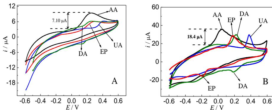
**Figure 2.** CVs of DA (20.0  $\mu\text{M}$ ), EP (30.0  $\mu\text{M}$ ), AA (600.0  $\mu\text{M}$ ) and UA (30.0  $\mu\text{M}$ ) singly at (A) a bare GCE and (B) modified electrode in PBS (pH 7.0).
