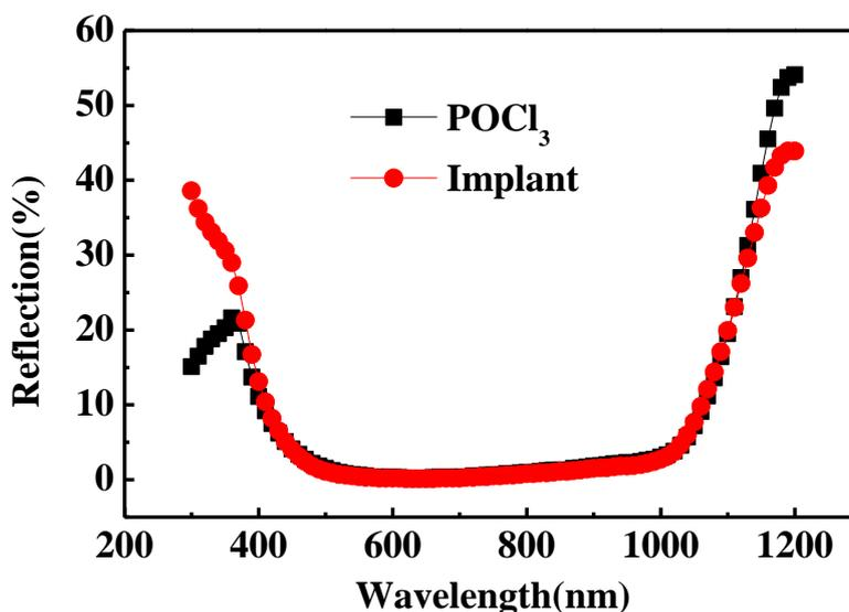
**Figure 3.** Surface reflection of POCl<sub>3</sub> and implant wafers after SiN<sub>x</sub> deposition
