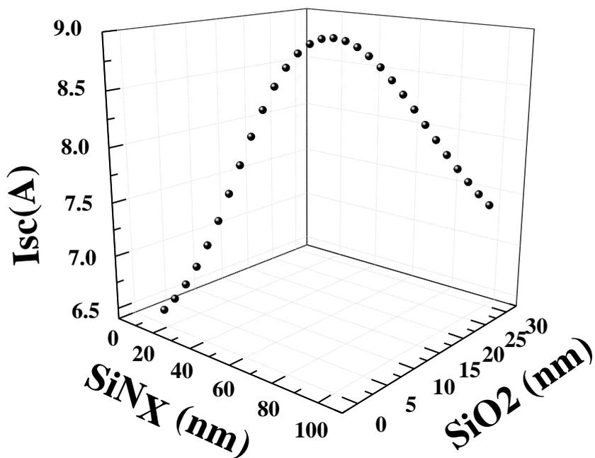
Figure 6. Simulation of the relationship between Isc, SiNx, and SiO2
