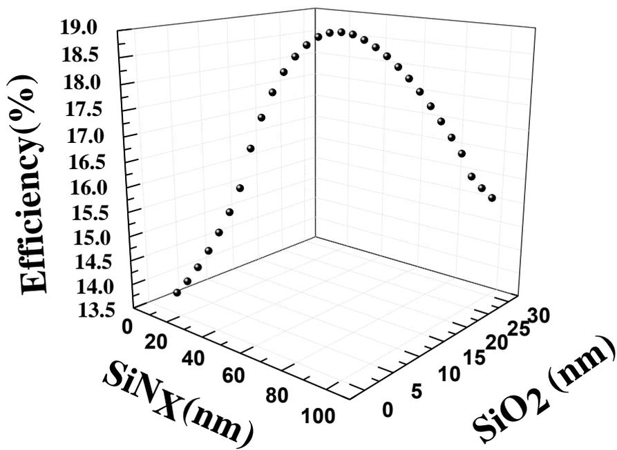
Figure 7. Simulation of the efficiency in relation to SiN<sub>x</sub> and SiO<sub>2</sub>
