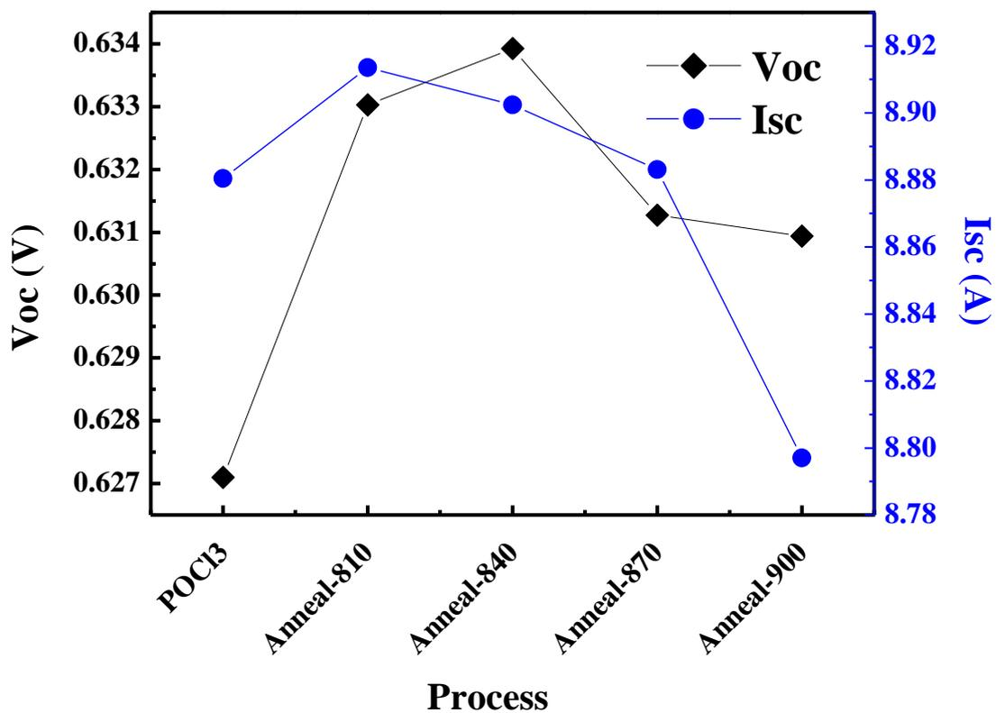
Figure 8. Voc and Isc of POCl<sub>3</sub> and the implant process
