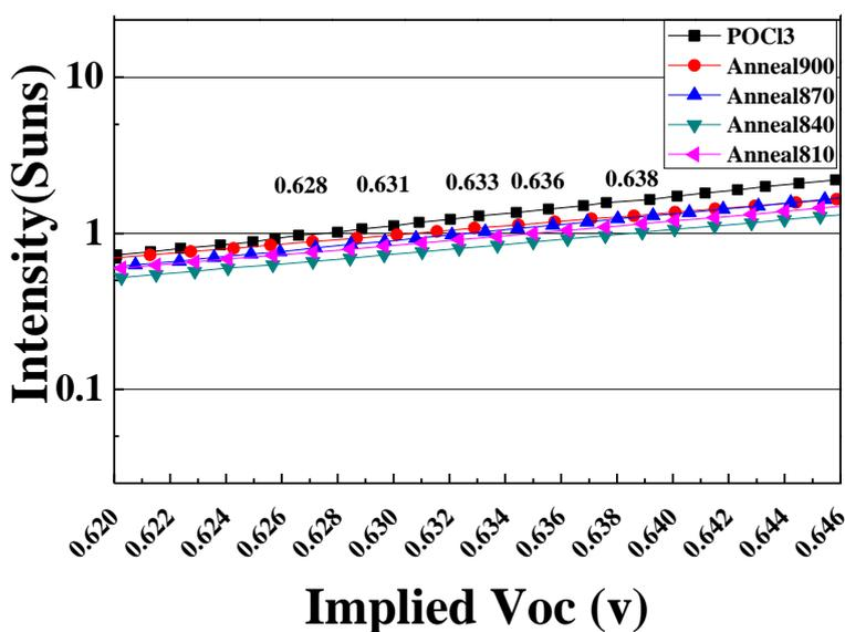
**Figure 2.** Implied Voc of POCl<sub>3</sub> and the implant process with a passivated double-sided layer
