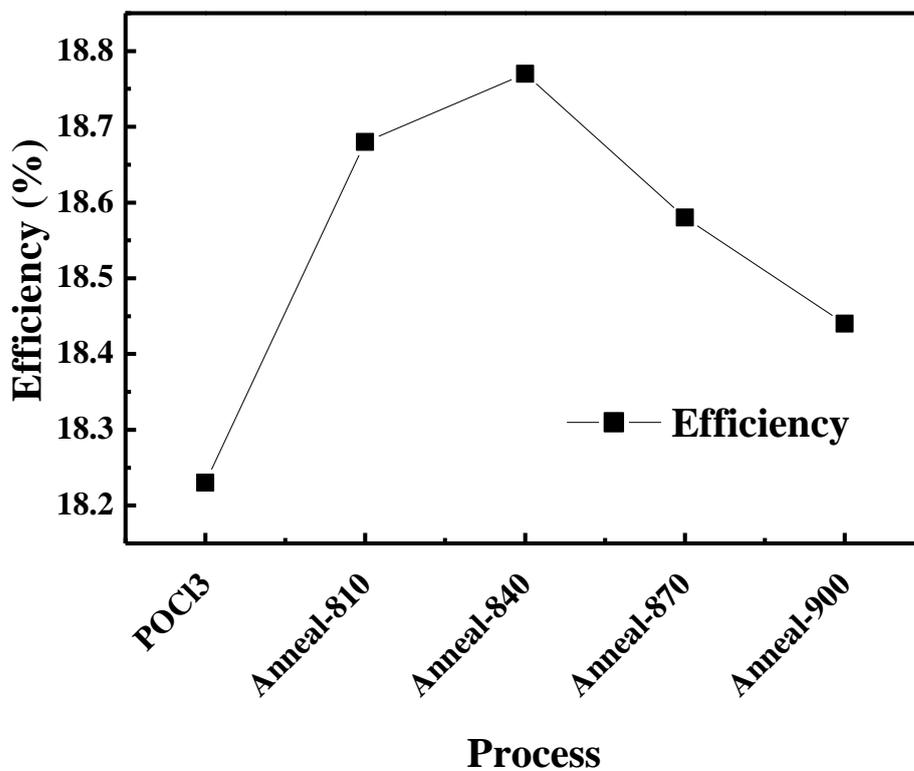
Figure 10. Efficiency of POCl<sub>3</sub> and the implant process
