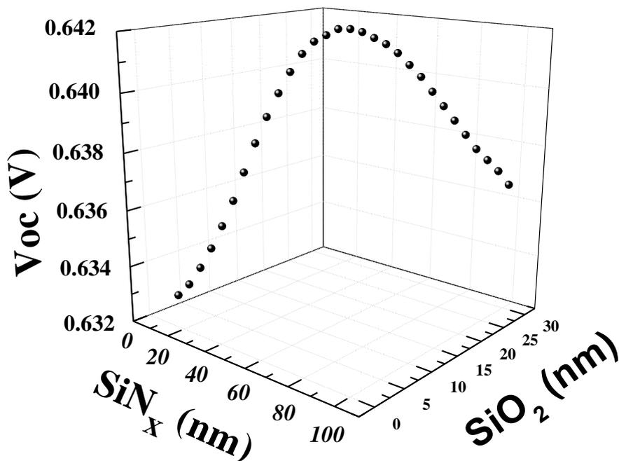
Figure 5. Simulation of relationship between Voc, SiNx, and SiO2
