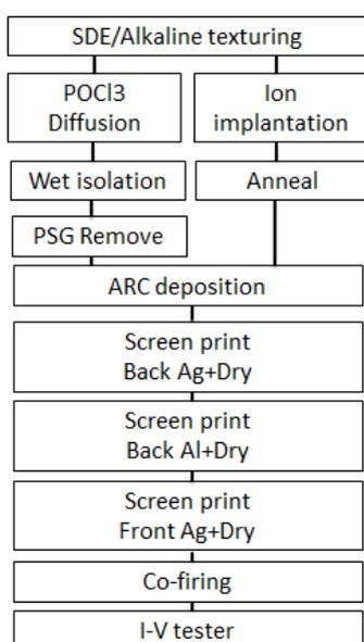
**Figure 1.** The process flowchart for conventional and ion-implanted solar cell production
