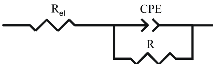
Figure 7. Equivalent electrical circuit used to fit the impedance spectra.
