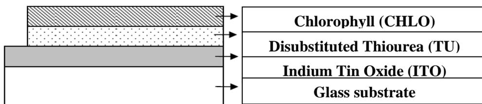
**Figure 2.** The general illustration of layer arrangement in thin film
