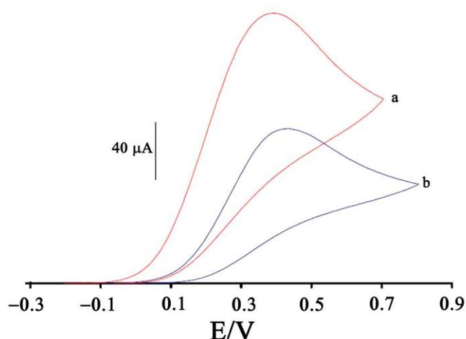
**Figure 4** Cyclic voltammograms of a) NiO/NPs/CPE, and b) CPE in presence of  $300$   $\mu\text{M}$  vitamin C at a pH 7.0, respectively.
