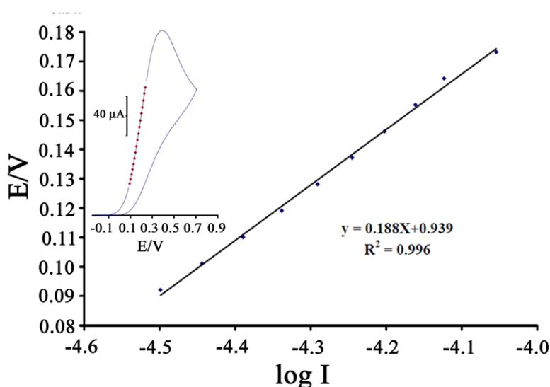
**Figure 5.** Tafel plot for NiO/NPs/CPE in 0.1 M PBS (pH 7.0) with a scan rate of  $50 \text{ mV s}^{-1}$  in the presence of  $300 \mu\text{M}$  vitamin C.
