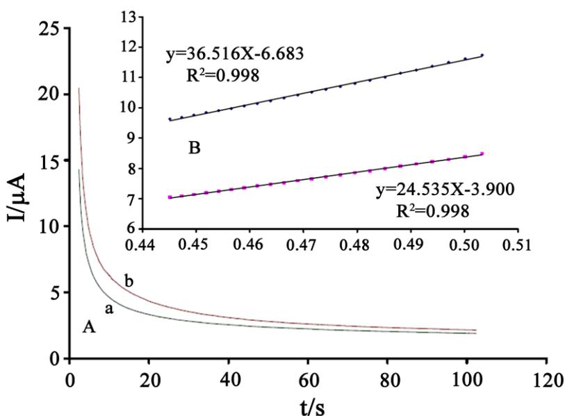
**Figure 6** A) Chronoamperograms obtained at the NiO/NPs/CPE in the presence of a) 100; and b) 200  $\mu\text{M}$  vitamin C in the buffer solution (pH 7.0). B) Cottrell's plot for the data from the chronoamperograms.
