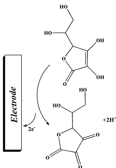
**Scheme 1.** The mechanism for electrooxidation of vitamin C
