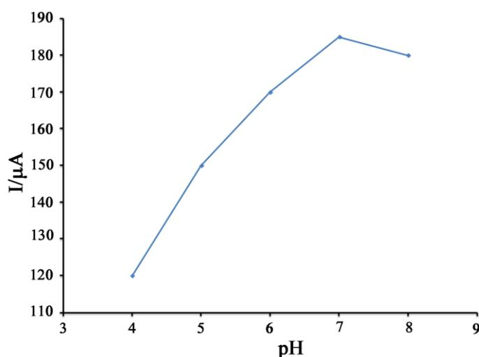
**Figure 3.** Current–pH curve for electrooxidation of  $300.0$   $\mu\text{M}$  vitamin C at NiO/NPs/CPE with a scan rate of  $50$   $\text{mV s}^{-1}$ .
