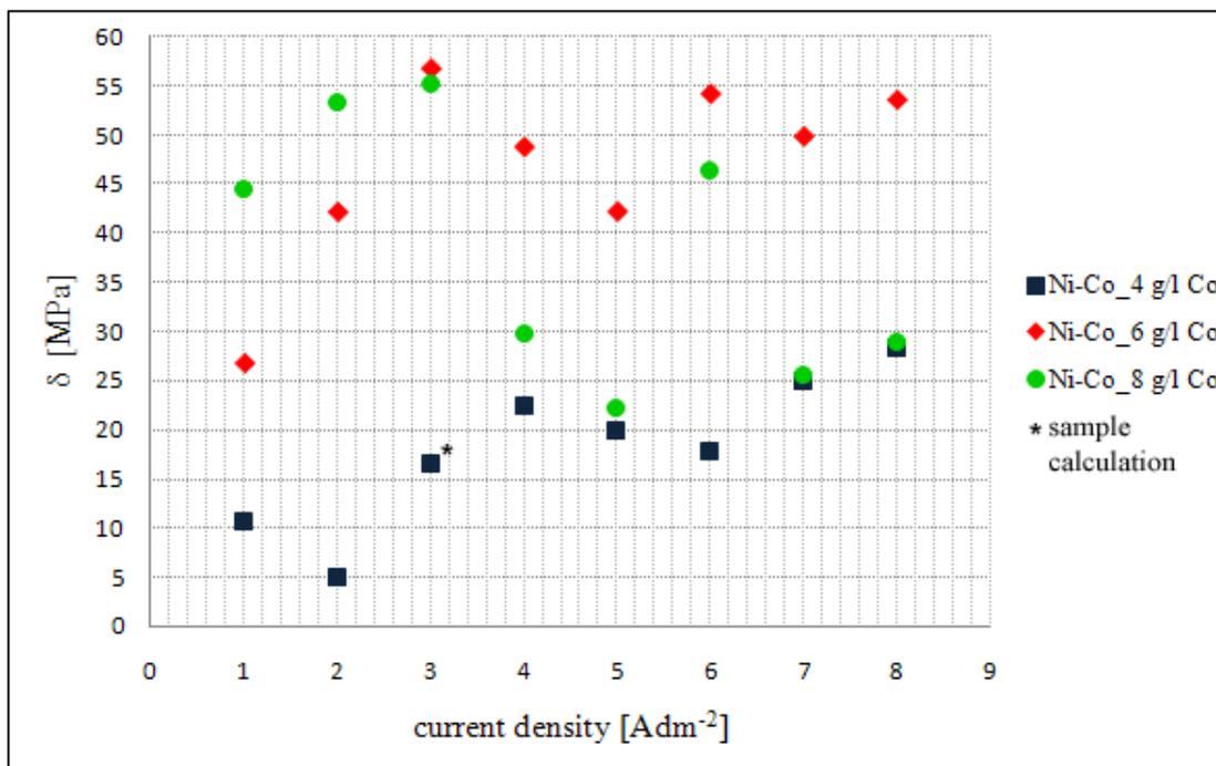
**Figure 4.** Magnitude of internal stresses in the Ni-Co coatings for individual concentrations of Co in the electrolyte in dependence on the current density
