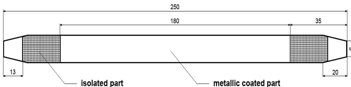
**Figure 1.** Shape and dimensions of the specimen used for determination of internal stresses
