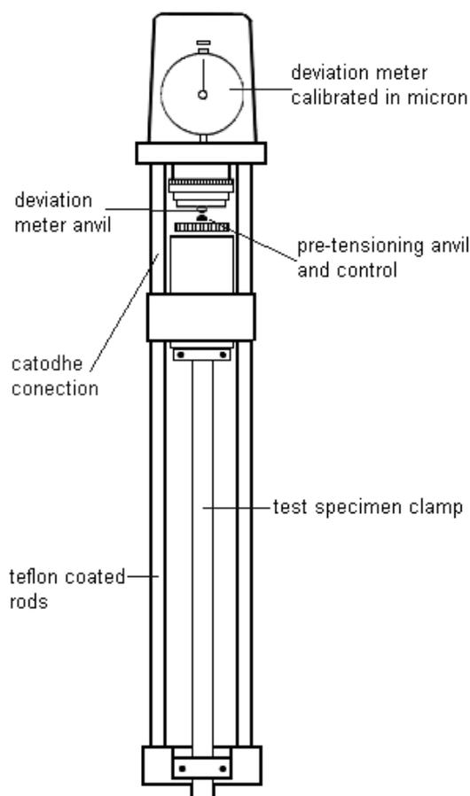
**Figure 2.** Scheme of the IS meter [3]
