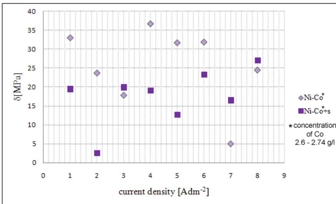
**Figure 5.** Internal stresses for Ni-Co coating without and with addition of saccharin into the electrolyte
