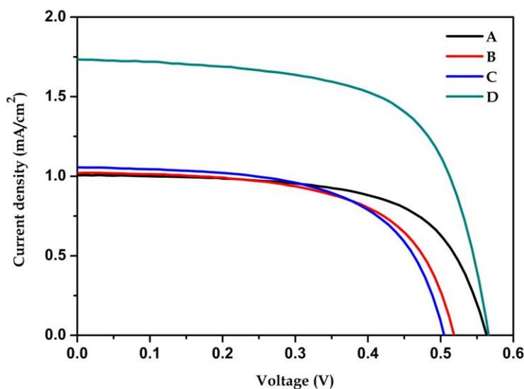
**Figure 5.** Photocurrent-voltage characteristics of the DSSC using the natural dye of *Curcuma longa* L. (A – Curcumin; B – Curcumin treated with hydrochloric acid; C – Curcumin treated with nitric acid; D – Curcumin treated with acetic acid)
