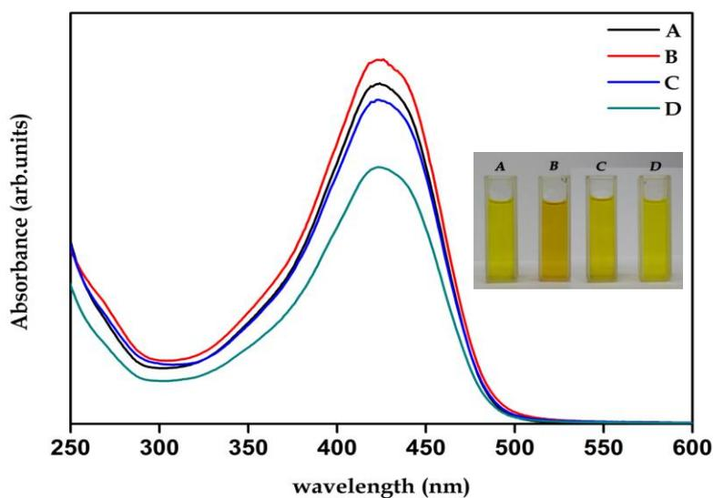
**Figure 2.** UV absorption spectra of natural dye solution extracted from *Curcuma longa* L. A - Curcumin; B - Curcumin treated with hydrochloric acid; C - Curcumin treated with nitric acid; D - Curcumin treated with acetic acid (Inset figure: Image of fresh dye solutions)
