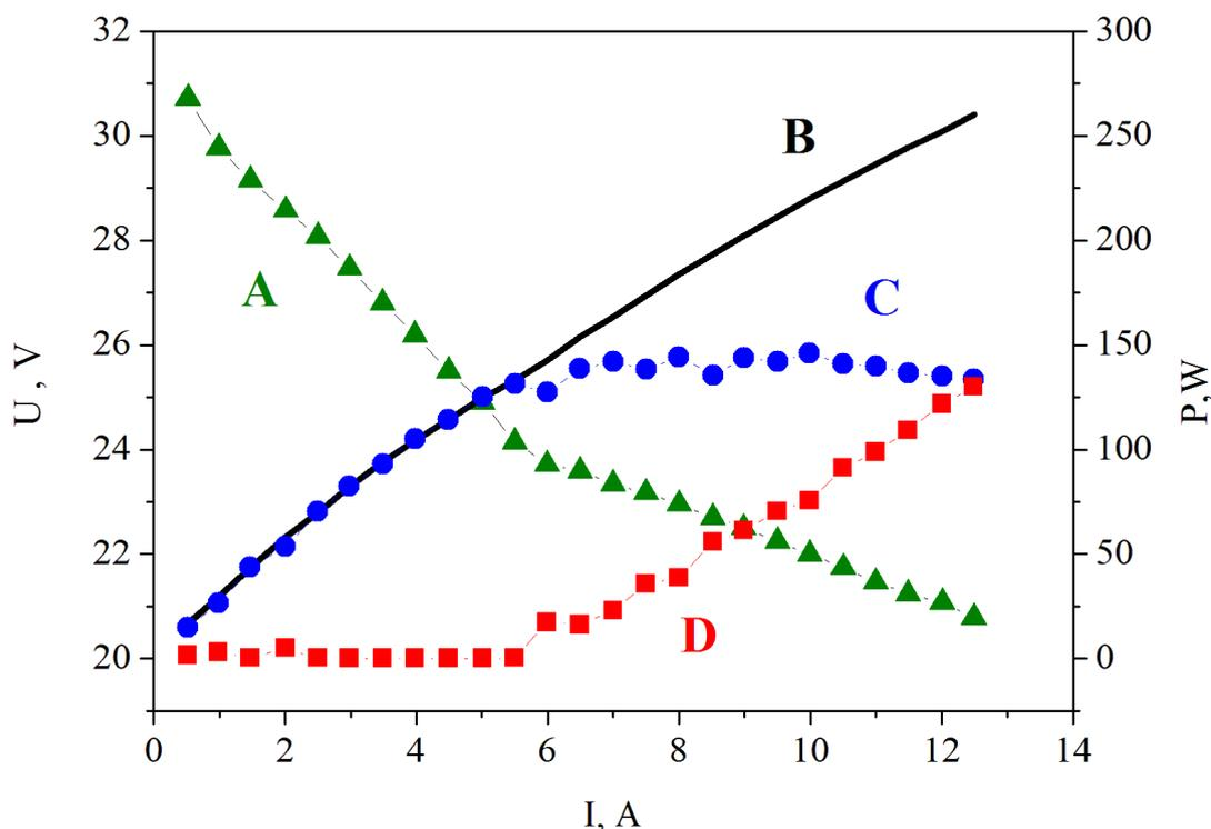
**Figure 3.** b) The voltage ( $U$ ) vs. current ( $I$ ) (A) and power ( $P$ ) – current ( $I$ ) (B) dependences determined for Areopack hybrid system (battery + PEM stack). The separate curves P-I for the battery pack (D), and PEM stack (C) only were added
