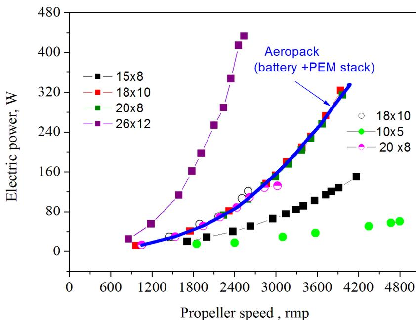
**Figure 7. b)** The dependences of the electric power on the propeller speed for the C50 Hacker motor with different propellers. Square and circle centered points correspond to supply with (Li-Po) 6s battery pack and AEROPACK, respectively. The size of a propeller (diameter and pitch) is given in inches next to the centered points.
