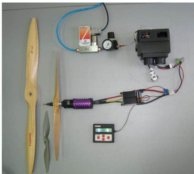
**Figure 7. a)** The photo of an experimental setup: the Hacker 13XL C50 brushless motor together with propellers
