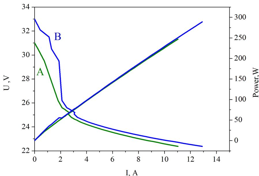
**Figure 3.** a) The voltage ( $U$ ) – current ( $I$ ) and power ( $P$ ) – current ( $I$ ) dependences determined for the AEROPACK hybrid system. The fuel cell stack was supplied with compressed hydrogen from the regular steel (A) and composite cylinder (B).
