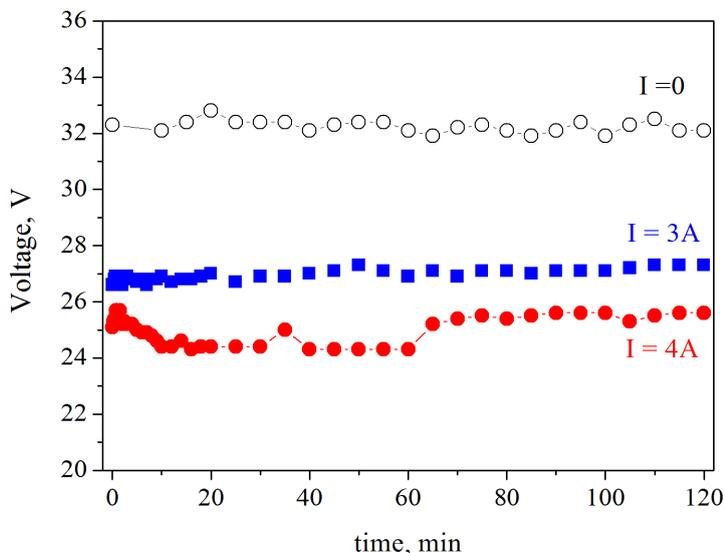
**Figure 5. a)** Time stability of voltage at the output unloaded (OCV,  $I=0$ ) and loaded with the constant current ( $I_1 = 3$  A and  $I_2 = 4$  A) hybrid system;
