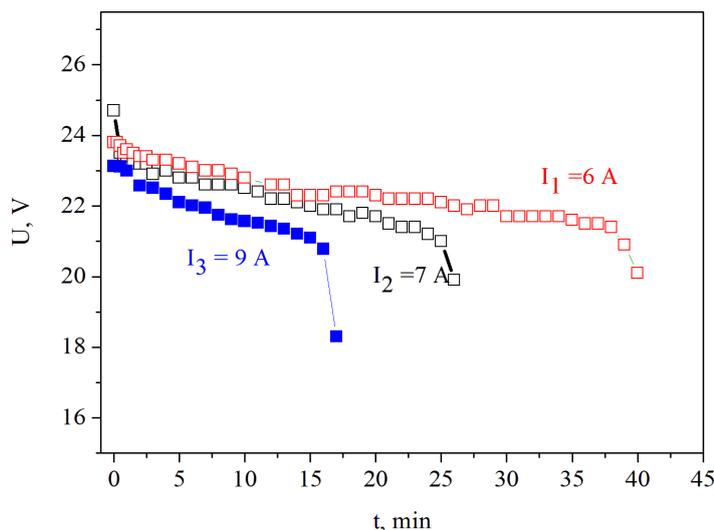
**Figure 5.** c) dependence of the voltage ( $U$ ) on the time during loading with the constant current  $I_1 = 6\text{ A}$ ,  $I_2 = 7\text{ A}$ ,  $I_3 = 9\text{ A}$
