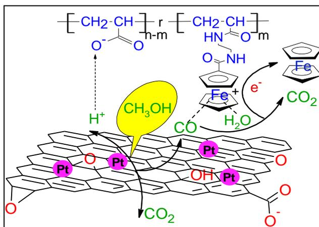
**Figure 6.** Schematic diagram explaining the high electro-catalytic performance of Pt NPs/PAA-Fc/GN for methanol oxidation.
