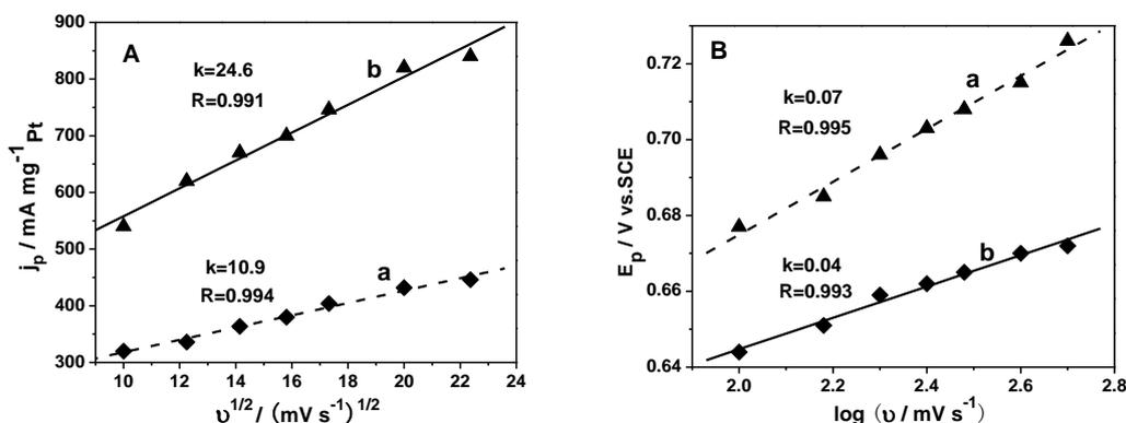
**Figure 5.** The relationship of peak current density ( $j_p$ ) vs. the square root of scan rate ( $v^{1/2}$ ) of Pt NPs/GN (a) and Pt NPs/PAA-Fc/GN (b) in 0.5 M  $\text{H}_2\text{SO}_4$ +0.5 M methanol aqueous solution (A), and the corresponding relationship of peak potential ( $E_p$ ) vs.  $\log(v)$  (B).
