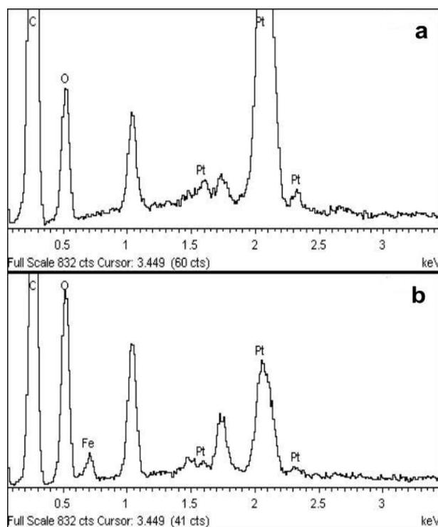
**Figure 3.** EDX spectra of Pt NPs/GN (a) and Pt NPs/PAA-Fc/GN (b).
