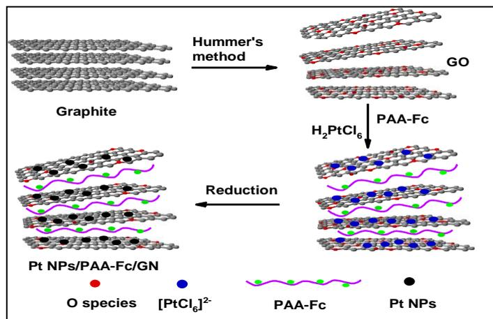
**Figure 1.** Schematic of the fabrication procedure of Pt NPs/PAA-Fc/GN catalyst.
