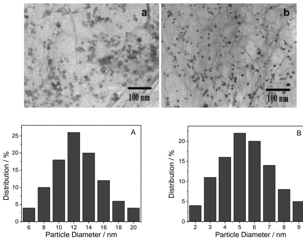
**Figure 2.** TEM images of Pt NPs/GN (a) and Pt NPs/PAA-Fc/GN (b), and the corresponding diameter distribution histograms (A: Pt NPs/GN; B: Pt NPs/PAA-Fc/GN).
