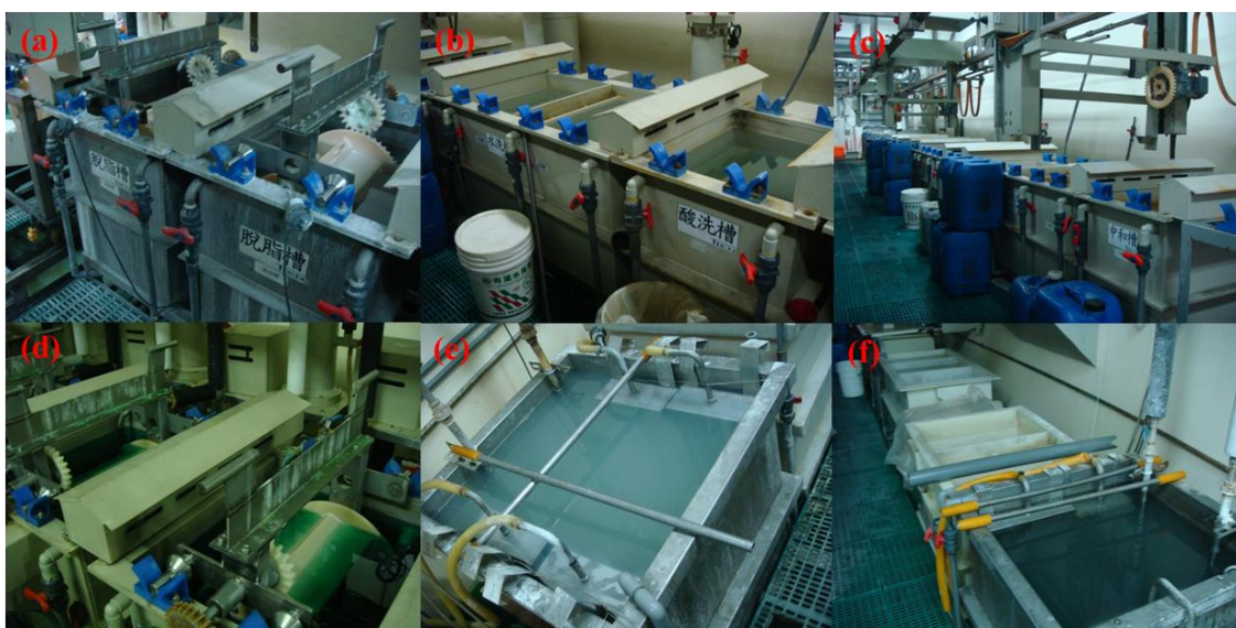
Figure 3. Electroless plating setup for the electroless plating of Ni (a) degreasing (b) acid cleaning (c) neutralizing with alkaline (d) electroless plating of Ni (e) ultrasonic cleaning (f) water cleaning and rinsing
